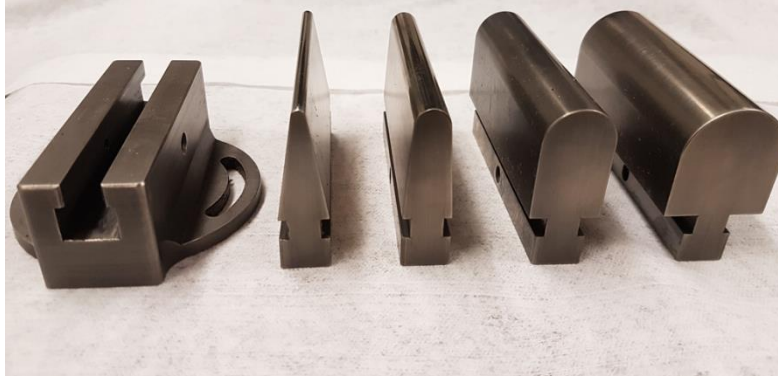
Figure 3-6 – ASBT punch platform (left) and punches with radius of (left to right): 1, 5, 10, 15 mm
