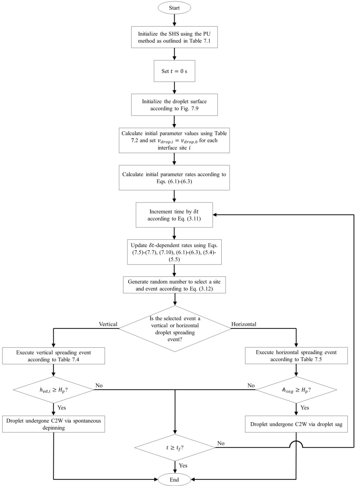
Figure 7.8: Flowchart of the SHS-MFkMC algorithm
