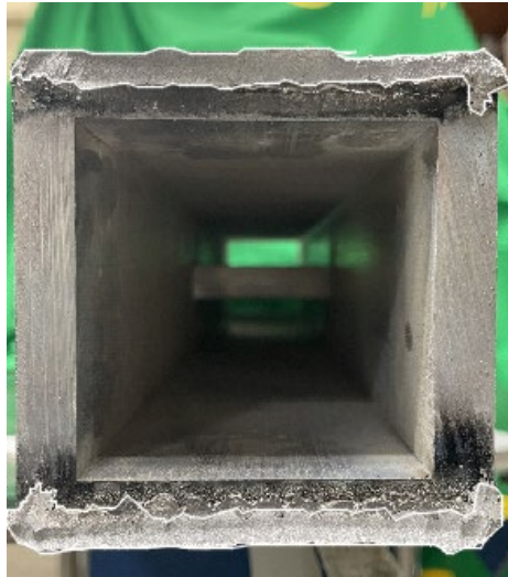
Figure 3.12: Specimens failed in fatigue showing region of weld where effective throat was measured by calculating area surrounded by white lines.
