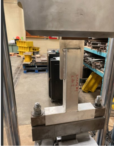
Figure 3.3: Experimental setup of R4.8 specimen in Shorewestern Frame.
