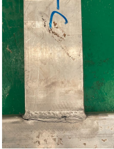
Figure 3.11: Fatigue cracking in the heat affected zone of an R-HG sample.
