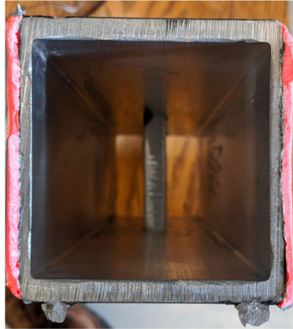
Figure 3.7: A failed tubular sample with weld area highlighted in red [27].
