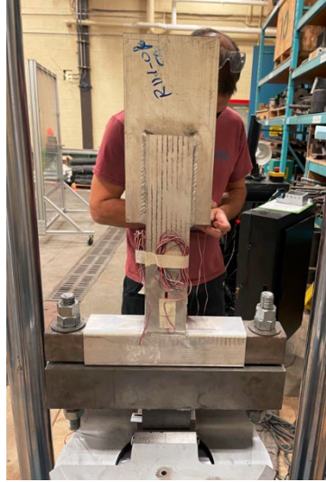
Figure 3.9: Placement of strain gauges for verification of specimen alignment.
