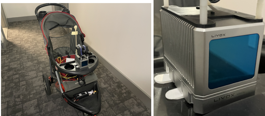
Figure 3.2 Mobile Laser Scanning system (left) and the Livox Horizon laser scanner(right)
