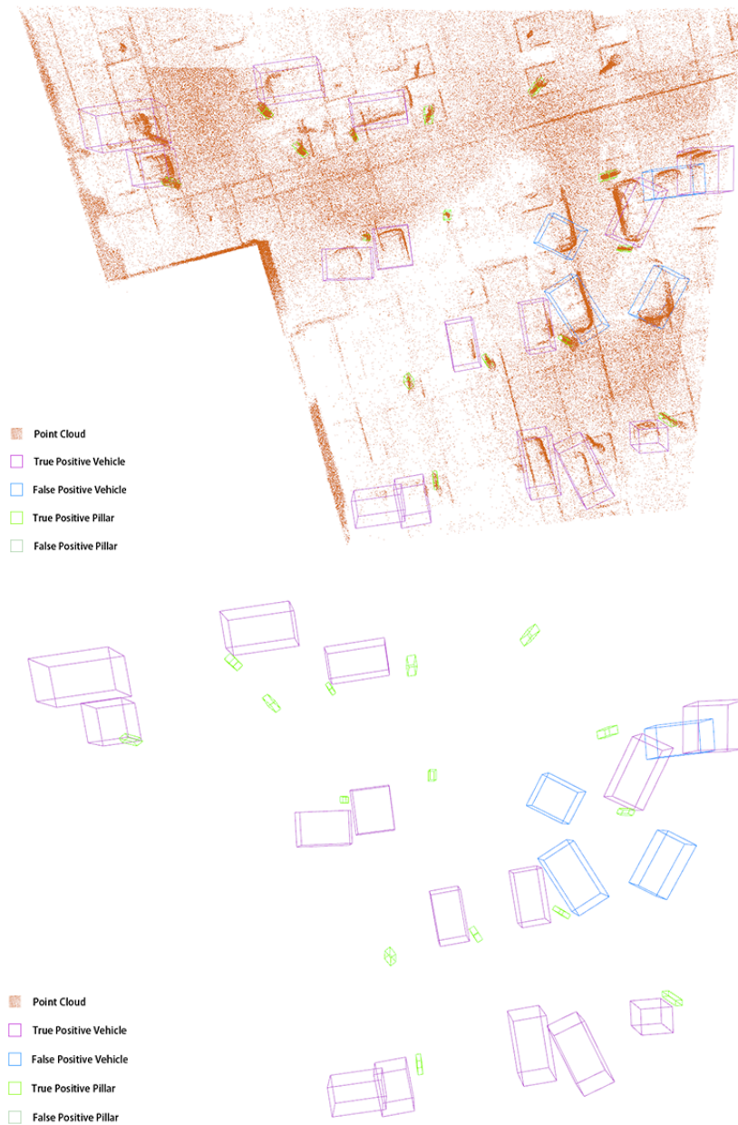
Figure 4.3 Object Detection Result of low-density point cloud
