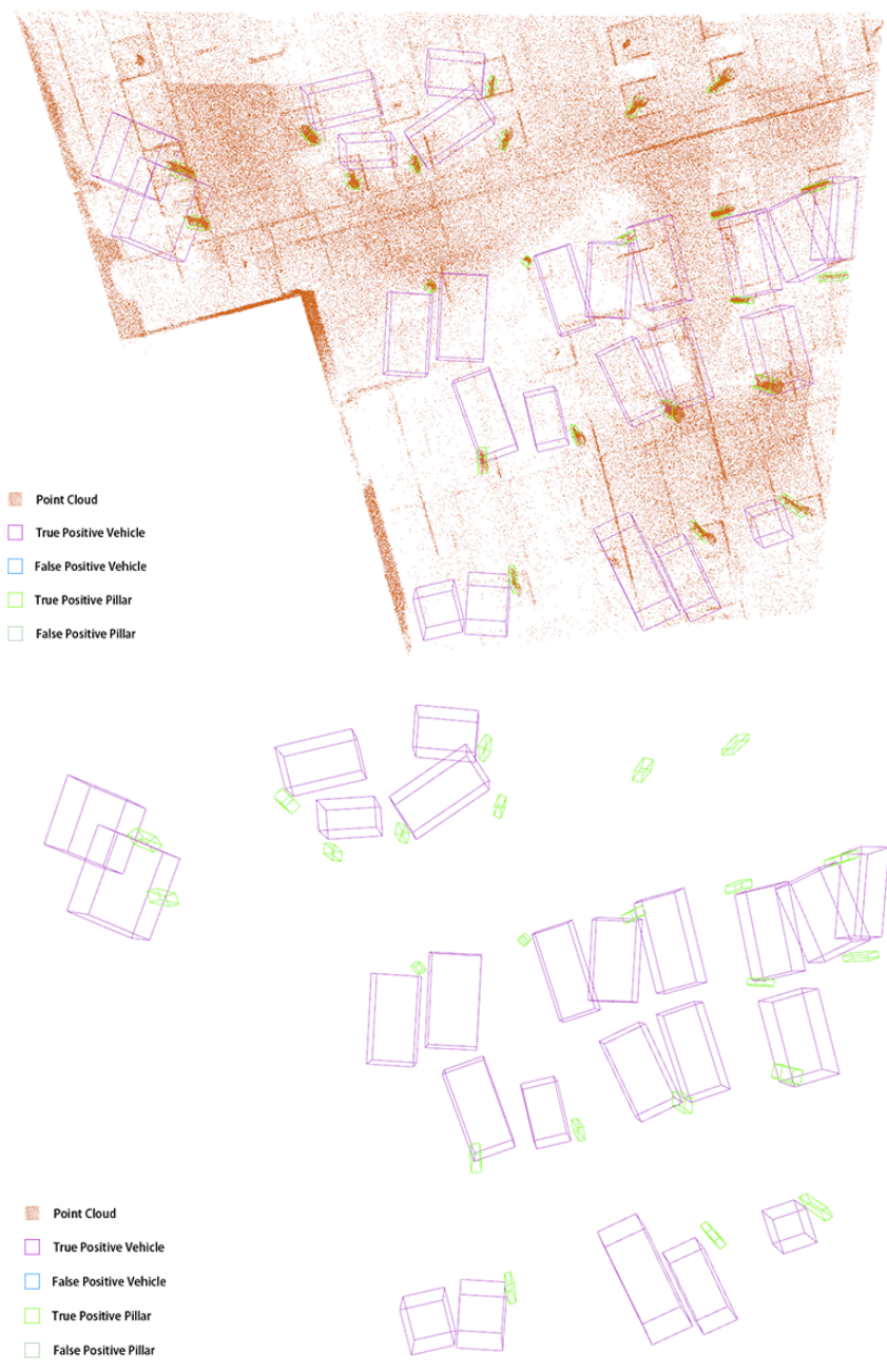
Figure 4.2 Reference point cloud and ground truth bounding boxes
