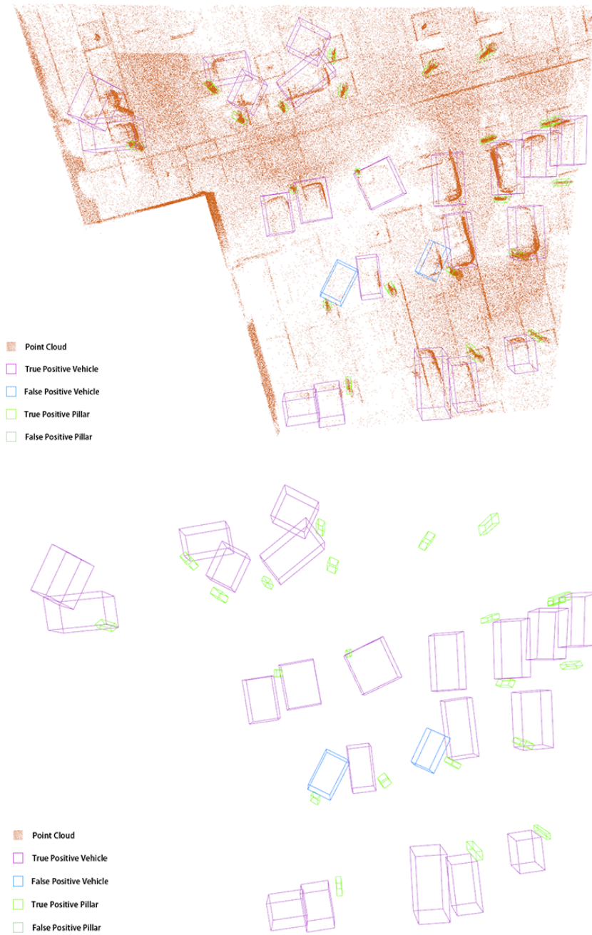
Figure 4.4 Object Detection Result of upsampled point cloud by PU-Net
