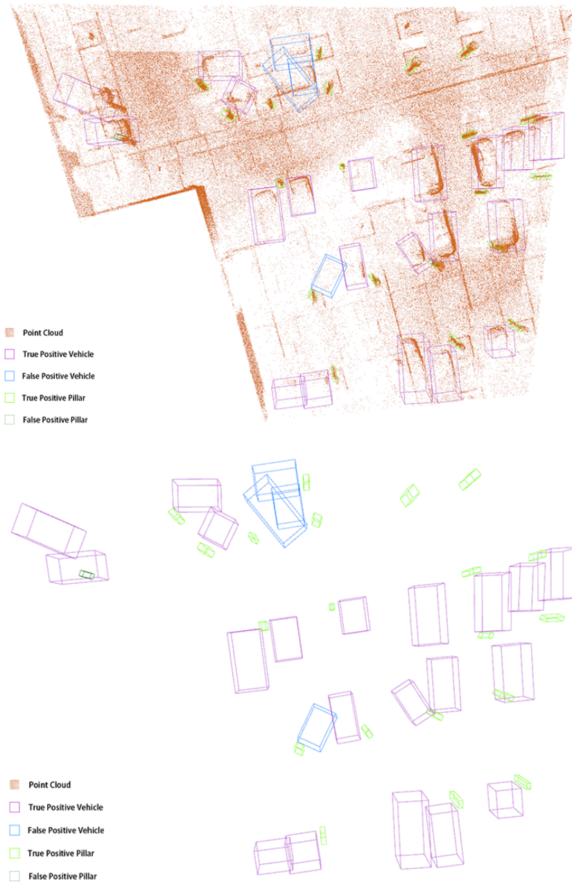
Figure 4.6 Object Detection Result of upsampled point cloud by PU-GCN
