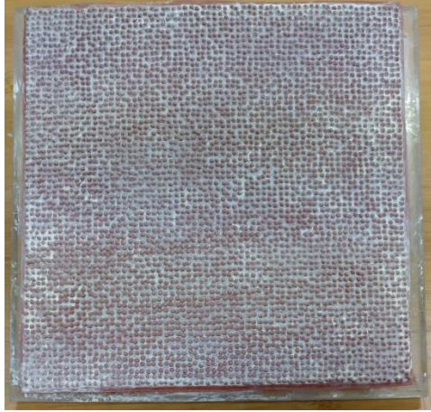
Figure 97: Tactical speckling rubber stamp with a dot size of 0.66 mm made by Correlated Solutions
