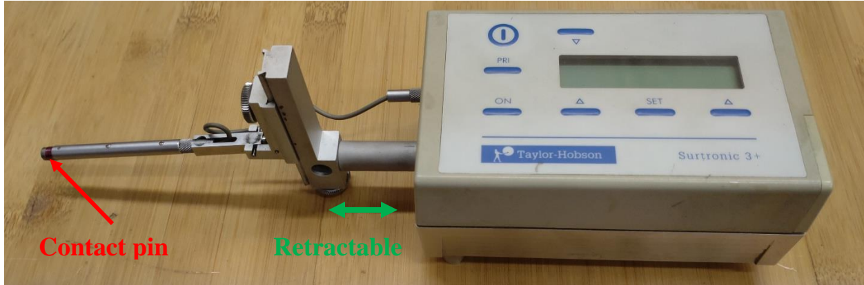
Figure 25: Taylor-Hobson contact profilometer. The contact pin is located on the underside of the retractable arm.
