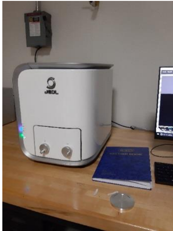
Figure 26: Table-Top JEOL Scanning Electron Microscope.
