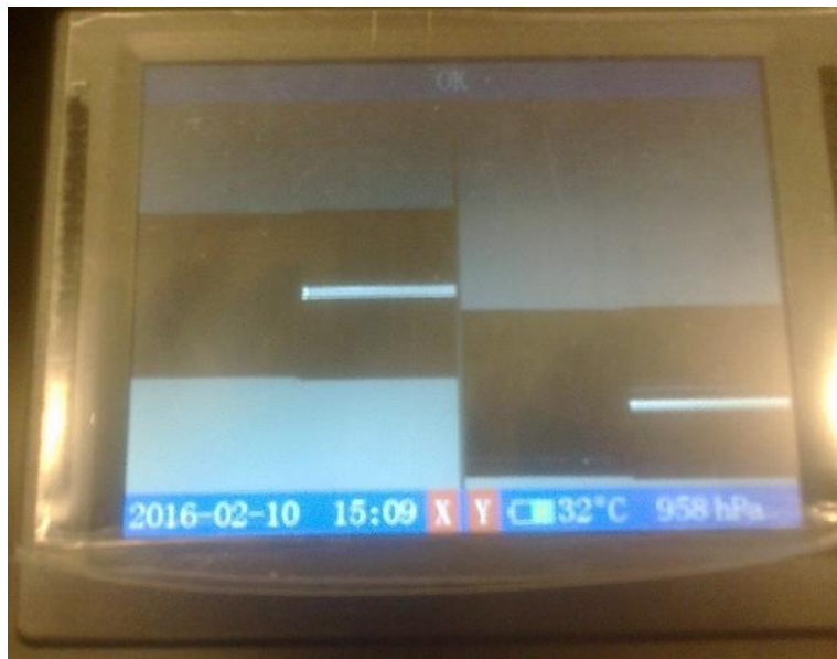
Figure 85: The splicer screen showing a top view of the HC-PCF & capillary interface (left of the screen) and a side view of the interface (right of the screen).
