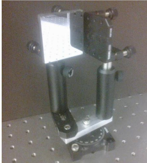
Figure 98: The assembled Lloyd Interferometer. The holder on the right is covered with partially sticking tape for easier loading and unloading of samples (the setup is enclosed in a box to minimize airflow avoiding optical path differences).
