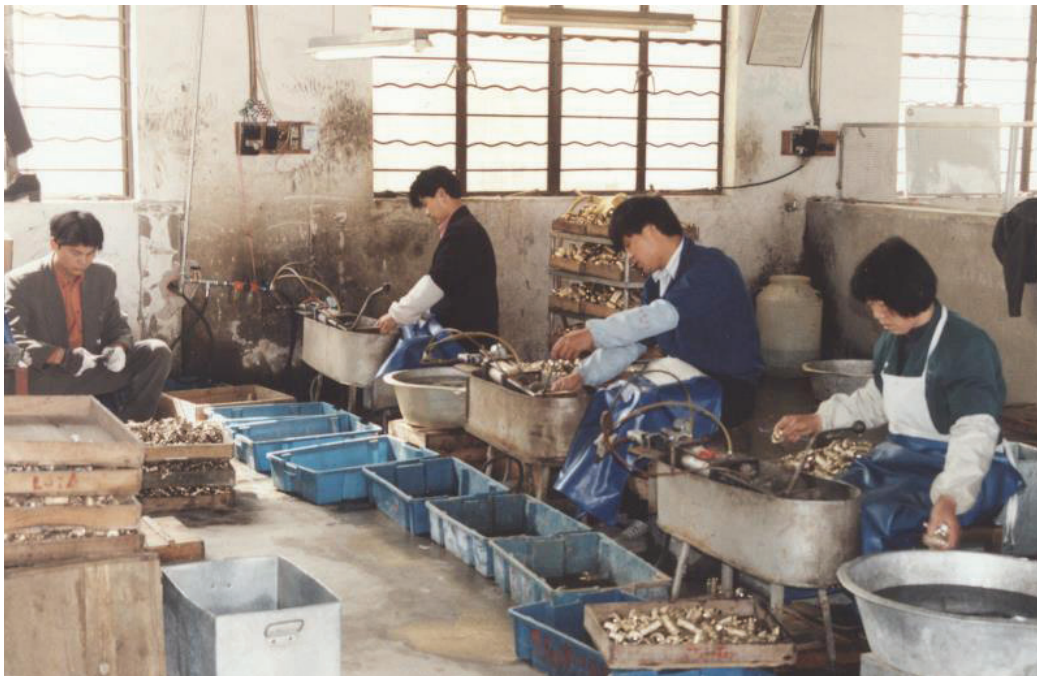
fig.4.10 Few stations set up for testing plumbing valves beside the machining workshop in the Xibin Factory. (Photograph taken on October 29th, 1994)
