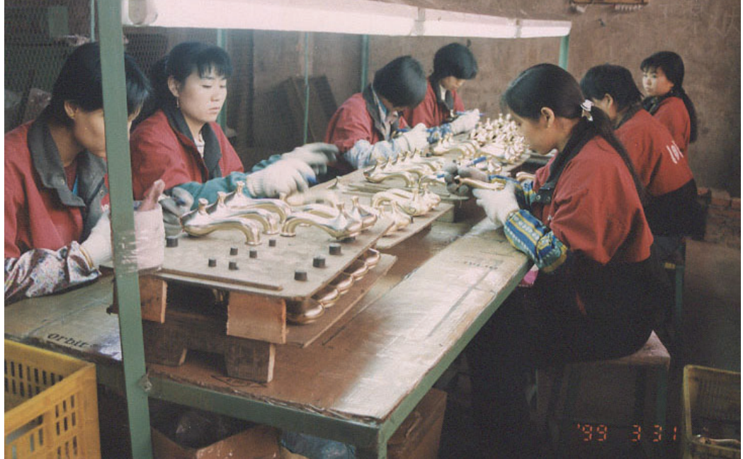
fig.4.12 Photograph of workers in uniforms checking the faucet spouts for quality control purpose before they were assembled. (Photograph taken on March 31st, 1999)
