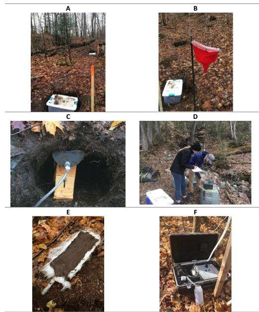
Figure B2 Images of field equipment used in TLW: A) shows two lysimeter pits in C32 B) throughfall collector in C31, C) mineral soil zero tension lysimeter during instillation, D) ISCO automated sampler being programed E) mineral soil zero tension lysimeter before instillation, F) peristaltic pump collecting groundwater.
