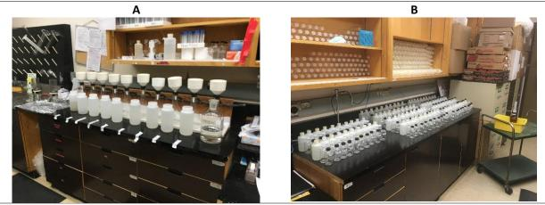
Figure B3 Images of laboratory set up in the Great Lakes Forestry Centre: A) water sample splitting apparatus that filters water samples from field bottles to laboratory bottles, B) water sample laboratory bottles.
