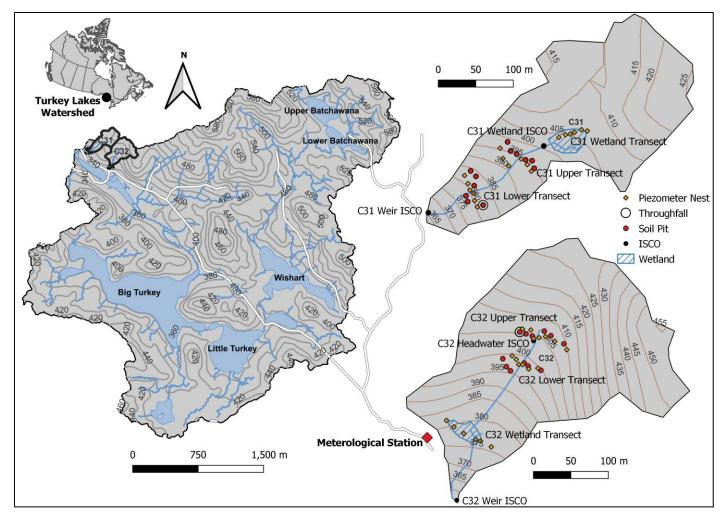
Figure 3.1 Maps of Turkey Lakes Watershed (left) and sub catchments C31 (clear-cut; top right) and C32 (control; bottom right). Locations of stream water sampling sights, groundwater piezometers, soil pits, throughfall collectors and wetlands are marked.
