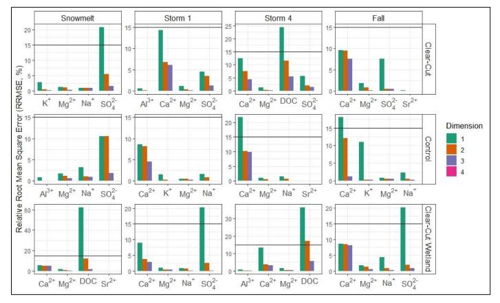
Figure 3.8 Relative root mean square error (RRMSE, %) for the tracers used in the EMMA models. Horizontal line represents the 15% cut off threshold recommended by James & Roulet, (2006). Colour represents the RRMSE explained by each principal component or dimension of the mixing subspace.
