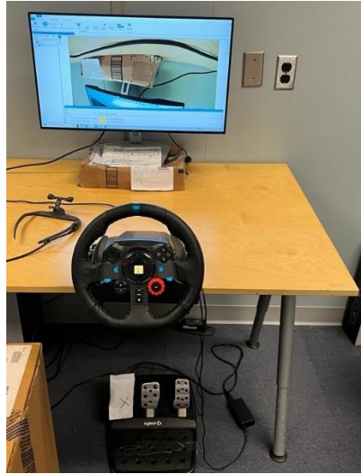
Figure 3.2 Simulator setup – includes the Logitech G29 steering wheel and pedal set.
