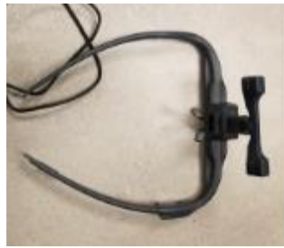
Figure 3.3 Ergoneers Dikablis Glasses 3 Eye Tracker used in the experiment [70]
