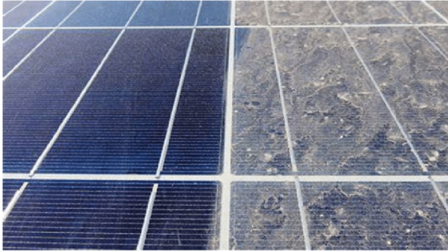
Figure 1.3: Clean vs Soiled PV Module. Image presented in [10]
