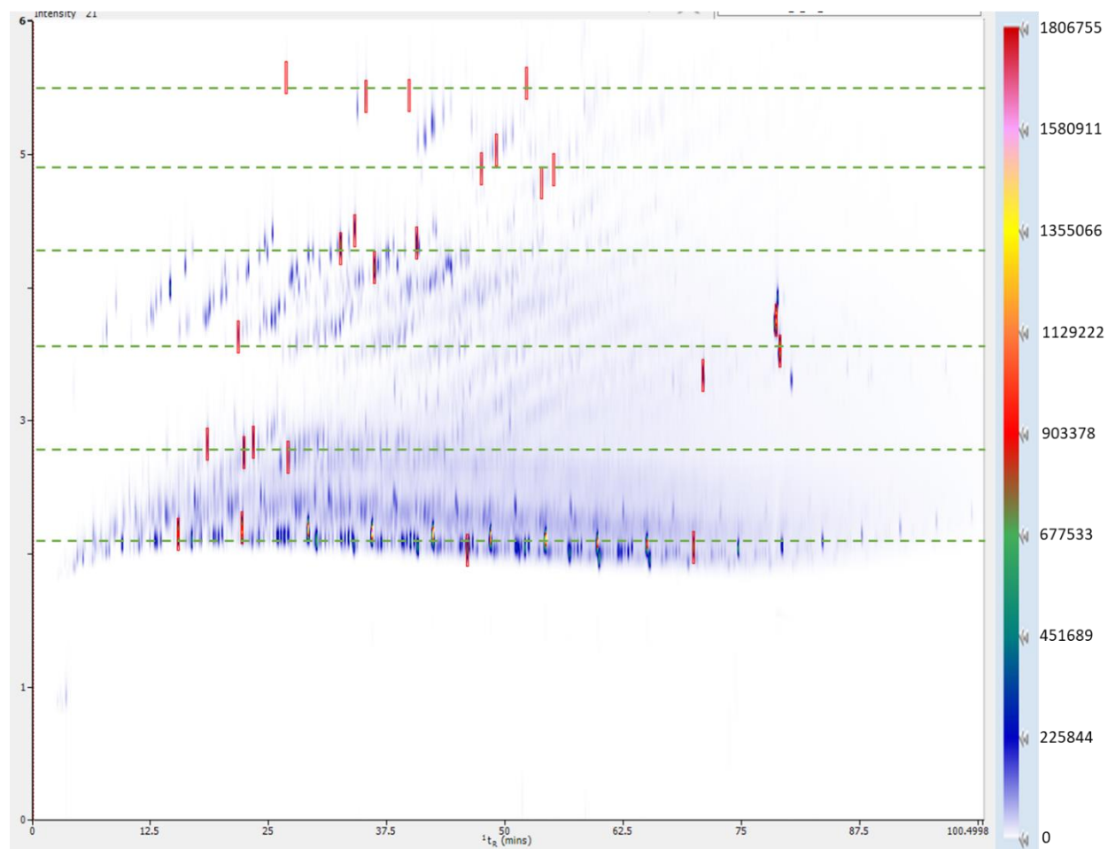
Figure C - 4: GC×GC-FID separation of diesel with 2 D temperature programming using an Rxi-5Sil MS W/Integra-Guard (39.219 m × 0.242 mm × 0.25 μm) 1 D column and an MXT-WAX (1.00 m × 0.25 mm × 0.25 μm) 2 D column. 2 D temperature programming: 2.5 s delay, 70 °C linear temperature increase over 1.5 s (at 20 °C/s), hold at 60 °C for 1.5 s, cool for 0.5 s. Optimized 2 D peak width (no wraparound peaks).
