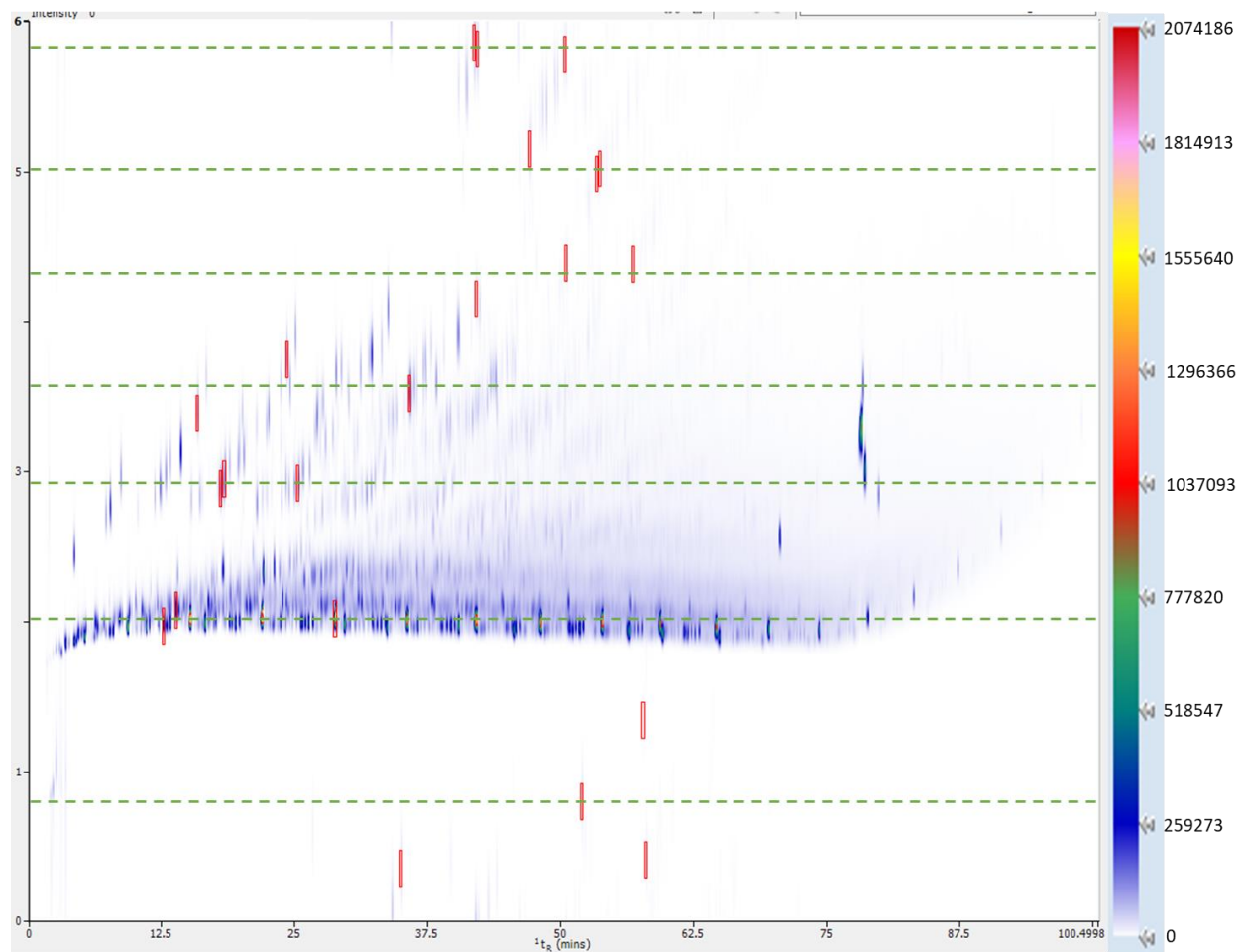
Figure C - 5: GC×GC-FID separation of diesel with secondary oven using an Rxi-5Sil MS W/Integra-Guard (39.219 m × 0.242 mm × 0.25 μm) 1 D column and an MXT-WAX (1.00 m × 0.25 mm × 0.25 μm) 2 D column. Constant temperature offset of +55 °C. Optimized 2 D peak width (no wraparound peaks).
