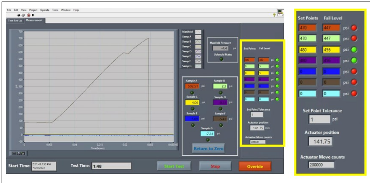
Figure 5.4: LabVIEW software interface for pressure testing at the University of Waterloo test facility.
