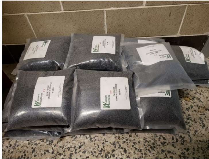
Figure 3.4: Lead shots obtained to adjust container weight to create various equivalent stresses on multiple CIPP specimens.
