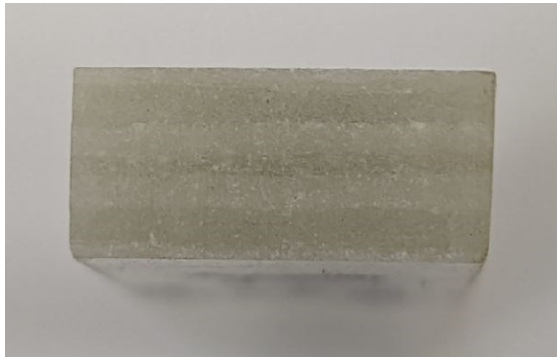
Figure 2.7: Cross-section of the composite I-Main CIPP liner having a uniform cross-section with no distinct reinforcement layers.
