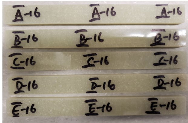
Figure 2.6: Flexural test specimens prepared for ASTM D790 testing.
