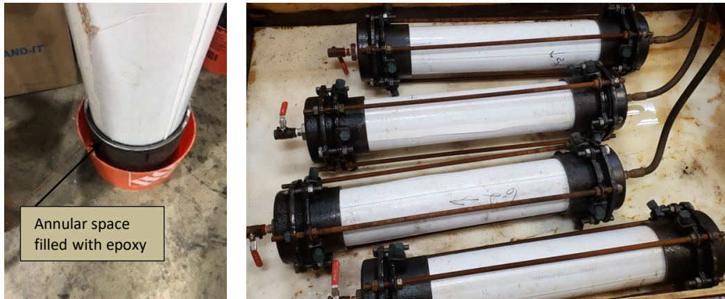
Figure 5.3: CIPP specimens prepared for pressure testing.
