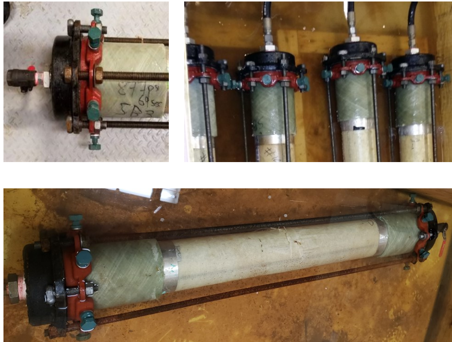
Figure 4.8: CIPP specimens after prepping with the MJ end caps and high-yield threaded bars.
