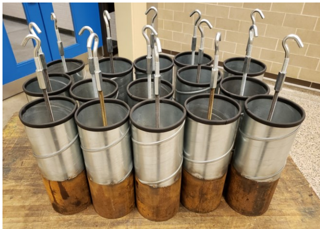
(a) Cylindrical-shaped hanging weight fabricated to test non-reinforced CIPP specimens.
