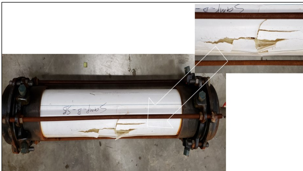
Figure 5.8: Failure that occurred in one of the CIPP specimens under sustained internal pressure.
