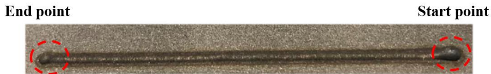
Figure 6-3: Effect of acceleration and deceleration of the deposition head on the start and end point of a single track
