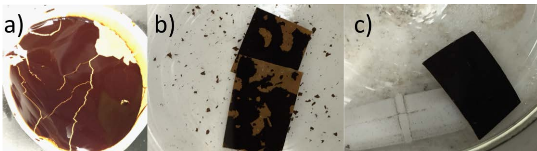
Figure 3-3: Membrane stability enhancement by \text{Zn}^{2+} crosslinking: (a) vacuum filtered GO membrane immersed in water for 30 min; (b,c) squares of membrane exposed to high speed mechanical stirring with no zinc treatment: squares in (b) have no \text{Zn}^{2+} treatment while the membrane in (c) was soaked in the \text{Zn}^{2+} solution for 24 h.
