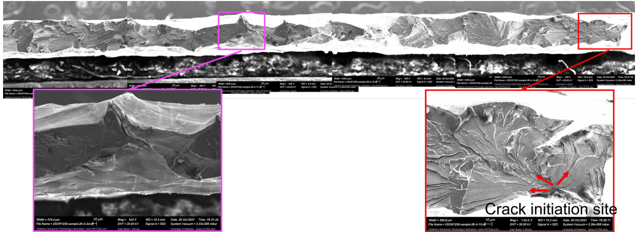
Figure 7.11: Typical fracture surface for low cycle Fatigue life specimens.
