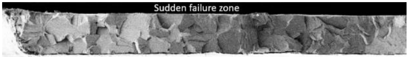
Figure 7.6: SEM image showing region of brittle fracture characterized by cleavage facets on the fracture surface
