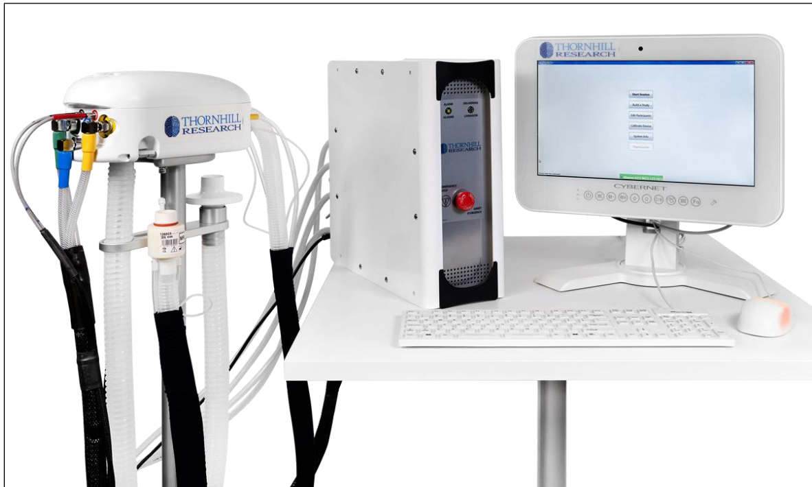
Figure 2.2: The RespirAct RA-MR device used for controlling gas delivery in breathing studies [25]
