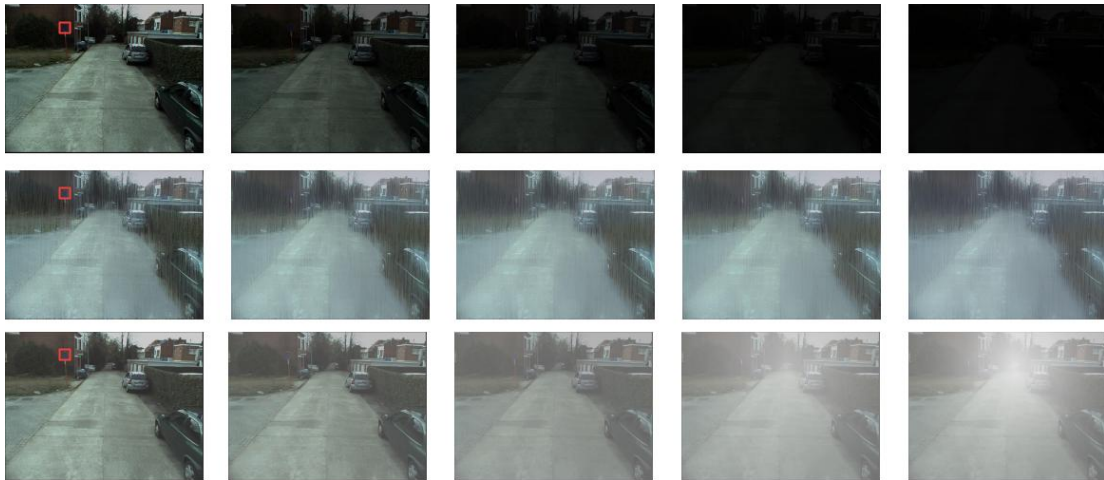
Figure 4.5: Example images from CURE-TSD with challenge levels 1 to 5 (from left to right). The top row corresponds to the dark perturbation, the middle is associated with rain and the bottom row is the haze effect.
