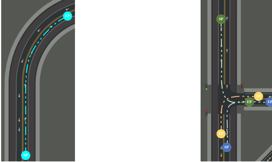
Figure 3.5: The testing scenarios used in this study. Left: driving straight following the lane at single-lane tertiary. Right: one-turn road following task based on the directional command at T-junction. The ego-vehicle is initiated at the spawning point (SP), and the mission is to driving towards the corresponding ending point (EP).
