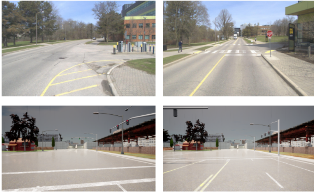
Figure 5.8: Sample front images from real (top row) and virtual (bottom row) driving environments. The left corresponds to the cases where the reference lane markings are unavailable, whereas the right two images correspond to the case with shorter lane information approaching the intersection.
