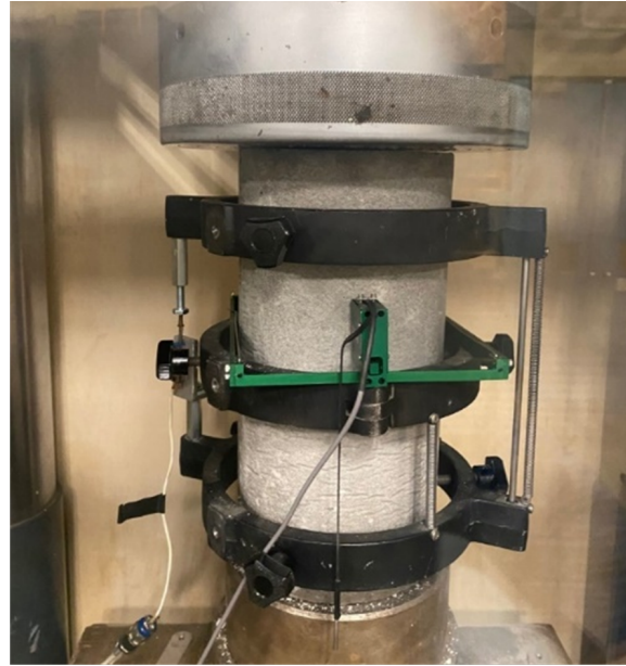
Modulus of Elasticity and Poisson's ratio test setup
