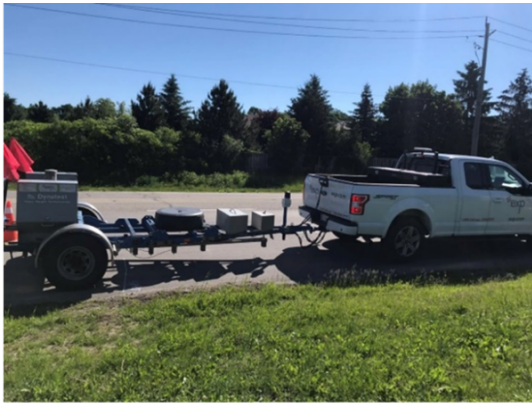
Falling Weight Deflectometer testing at Erbsville
