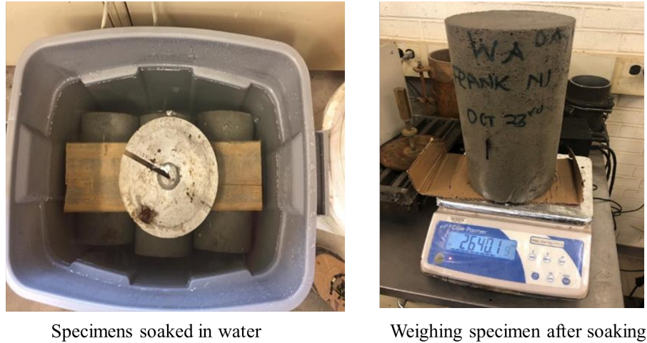
Figure 3.6: Water Absorption testing setup
