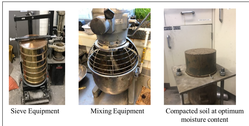
Figure 3.8: Sieve analysis and moisture content setup
