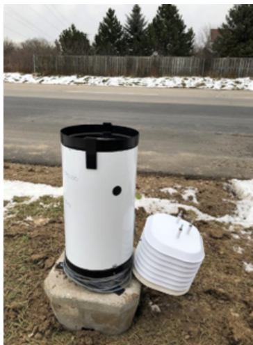
Figure 3.4: Rain gauge and Solar radiation shield
