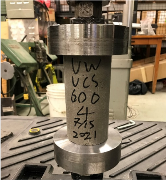
Unconfined Compressive Strength test setup
