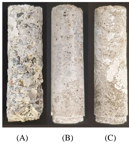
Figure 5.3. (A) Control, (B) MS-5%, (C) MS-10%, (D) PS-5%, and (E) PS-10% Concrete Specimens after 40 Freeze-Thaw Cycles
