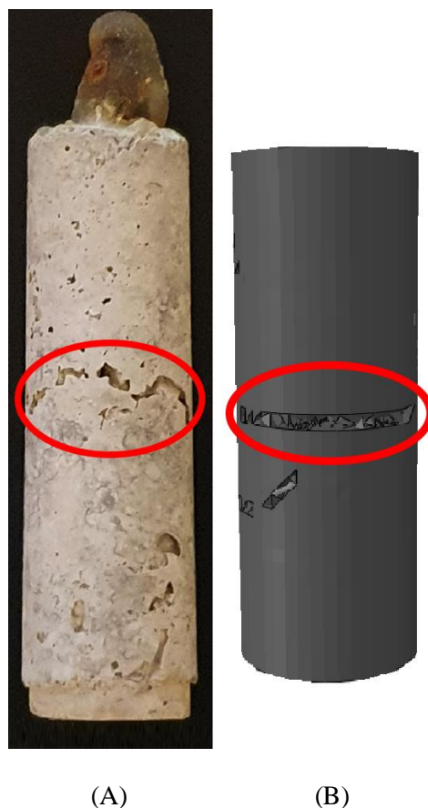
Figure 6.10. Comparison between (A) the Actual Concrete Damage and (B) the Simulated Concrete Damage at 1.5% of Reinforcement Expansion
