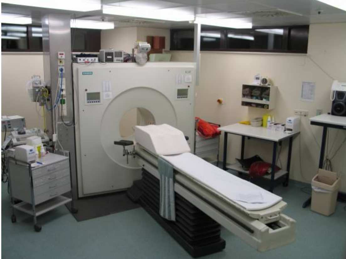
Figure 2.3: A typical PET scanner facility. Many modern PET scanners combine PET and computed tomography (CT), which helps image the anatomical structures, to form PET/CT machines capable of identifying and locating abnormalities in bodily functions. Public domain image adapted from [14].
