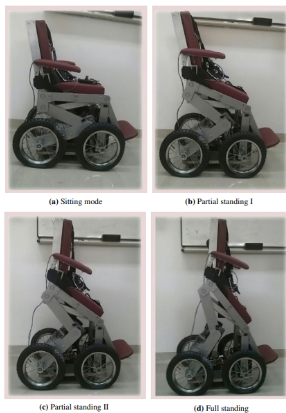
Figure 2.2: A robotic wheelchair with STS assistance and walking aid ( image taken from [3])
