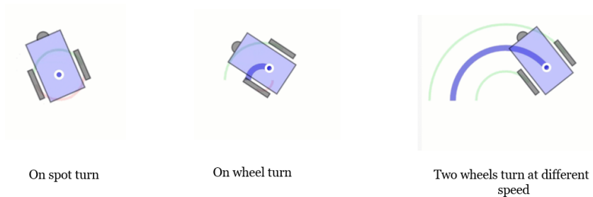
Figure 6.11: Three different types of turning. On spot turn will not change the robot position, only direction. Two wheels at the same speed need to go in opposite direction to stay in place. On wheel turn happen when one wheel is stationary and the other wheel rotate. This will change the position and the direction of the robot. It has a bigger turning radius compare to the on spot turn. Finally Two wheels turn at different speed has the biggest turning radius between turning types. it happen when one wheel is turning faster than the other on
