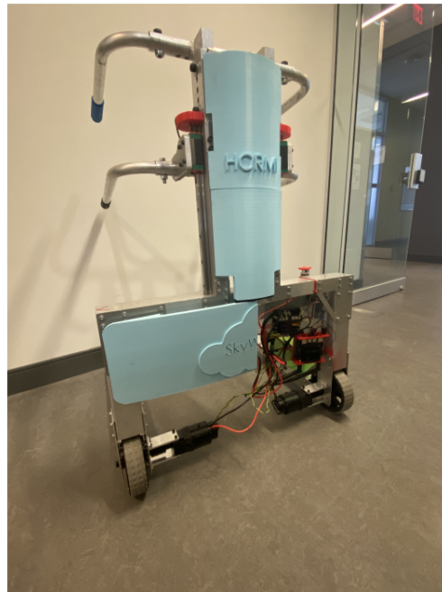
Figure 3.4: SkyWalker design with shell to hide electronics and motors
