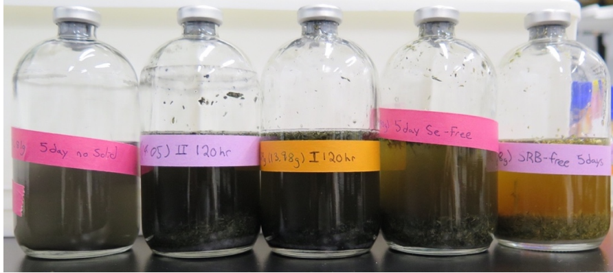
Figure 4.3: Sample vessels and controls 4 days after spiking with Se(IV). Note dark appearance of sand in all vessels except where there is no solid or no SRB.
