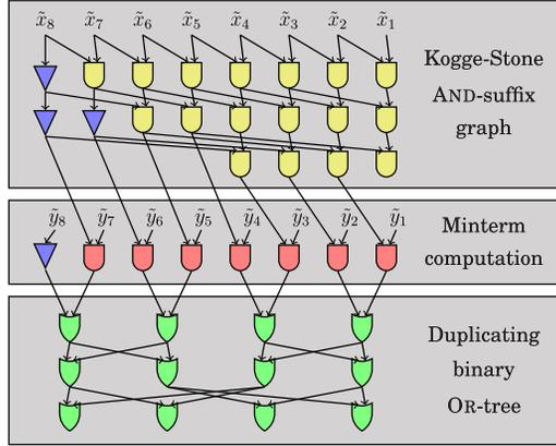
Fig. 3. A  $2^r$ -input  $2^{r-1}$ -output generate gate for  $r = 3$ . The top three rows are a  $2^r$ -input Kogge-Stone AND-suffix graph.
