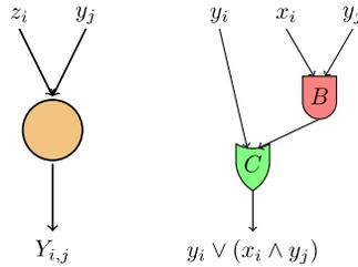
Fig. 7. The reduced output correction prefix gate of a refined Brent-Kung step with propagate signal computation omitted.
