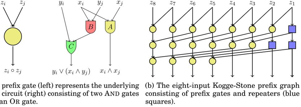
Fig. 1. Examples of a prefix gate and a prefix graph.
