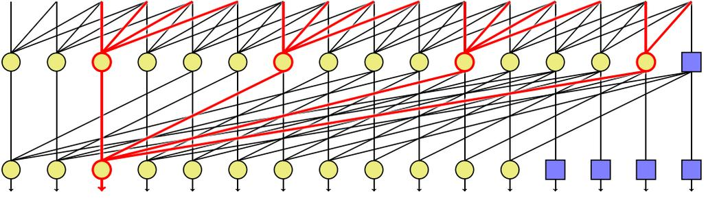
Fig. 5. A multi-input multi-output generate gate adder for  $r = k = 2$ , where yellow circles represent multi-input generate gates, and blue squares represent balanced binary repeater trees. The ancestors of one output are highlighted in red.
