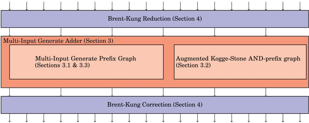
Fig. 2. High-level adder description.
