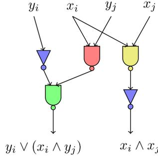
Fig. 8. A NAND/NOT prefix gate used for a modified Brent-Kung reduction step.
