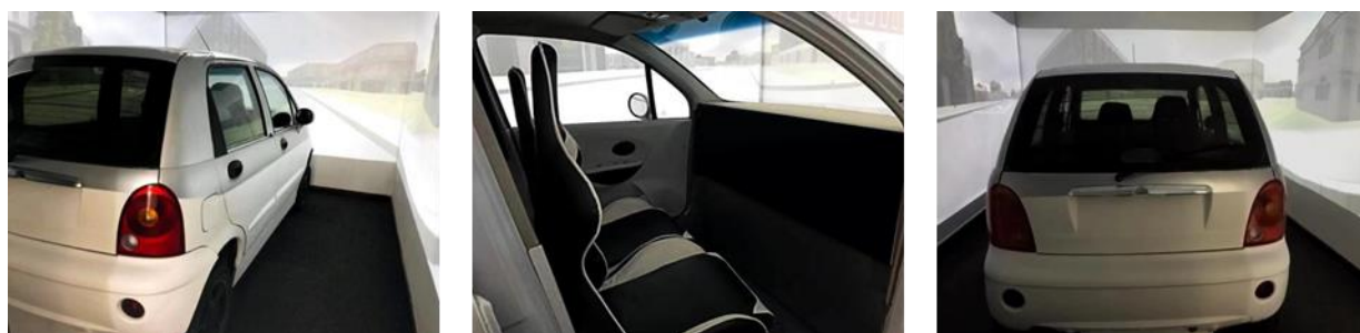
Figure 1. A fixed-based driving simulator with a 360° visual field of view
