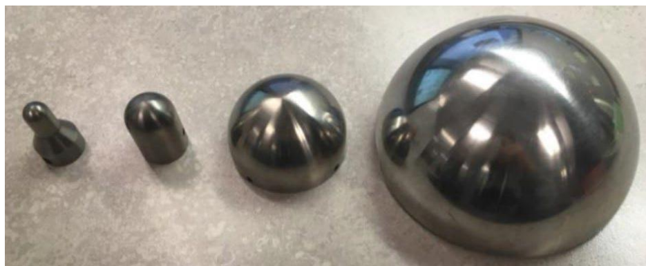
Figure 15: Punches used for equal-biaxial dome tests. From left to right: 5 mm, 10 mm, 25 mm, and 50.8 mm in radius Cheong et al. (2019; 2018).
