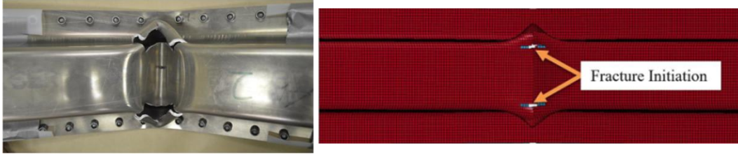
Figure 45: Visual comparison of the predicted and observed extent of fracture for the AA7075-T6 sheet alloy.
