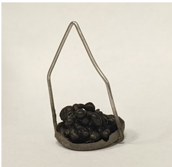
Figure 29. Example sample material after undergoing heating for thermogravimetric analysis.
