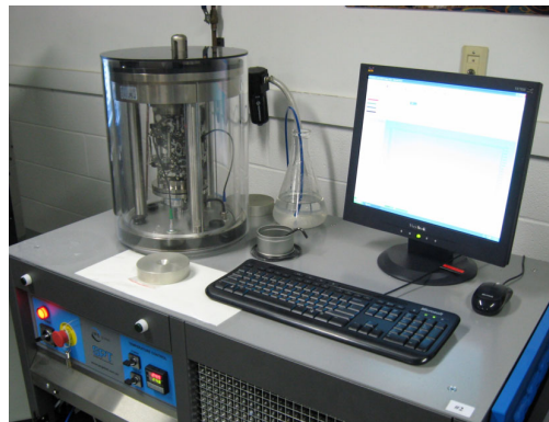
Figure 1-3: Setup of AMPT for testing asphalt mixes
