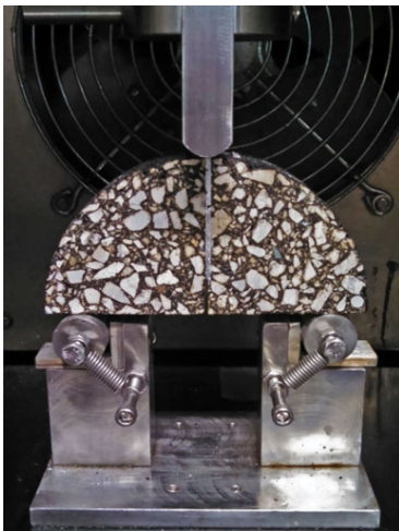
Figure 1-2: I-FIT test setup and example plot of results (Illinois-DOT, 2016)
