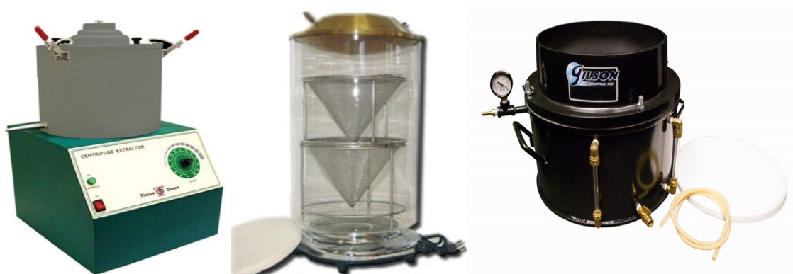
Figure 2-1: Asphalt cement extractor, from left to right: centrifuge (Method A), reflux extractor (Method B), vacuum extractor (Method C)
