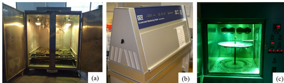
Figure 2-6: Accelerated weather aging devices: (a) Accelerated Weathering Machine; (b) Accelerated weathering tester; (Menapace et al., 2016) (c) UV aging oven (Zhu et al., 2018)
