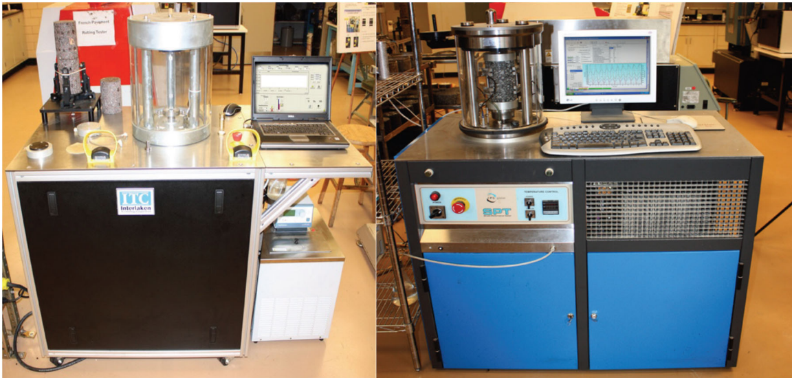
Figure 3-6: Photographs of AMPT Equipment by Interlaken Technology Corporation (left) and IPC Global (right)
