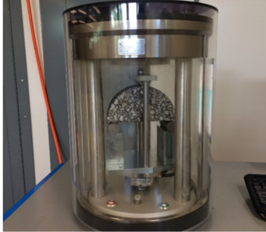
Figure 3-7: I-FIT Test using Semi-Circular Bending (SCB) specimen geometry
