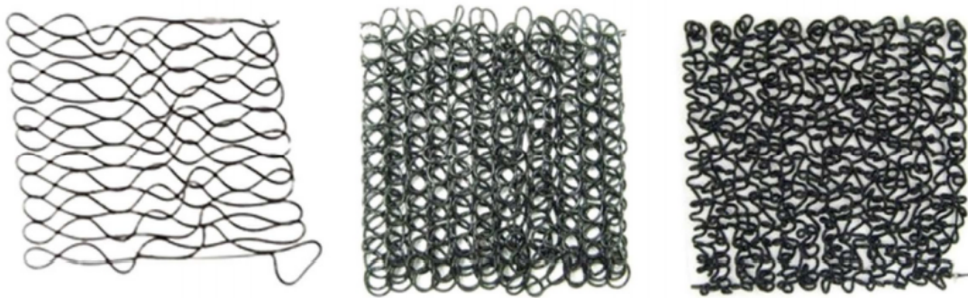
Figure 2.12: The demonstration of the Viscous Thread Instability (VTI) by Lipton. The patterns are obtained with the moving nozzle over the print bed with the increased flow rate. This can induce patterns such as meanders (left side), translated coil (middle), and alternating coil (right side) [69].
