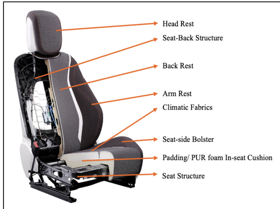
Figure 1.3: Demonstration of Automotive seat design structure [7], labelling the features: Head Rest, Seat-Back Structure, Back-Rest, Armrest, Seat-side Bolster, Padding (PUR foam In-seat Cushion), Climatic Fabrics, and Seat structure. (Source: By Johnson Controls and labelled by Gurkamal Saggu).
