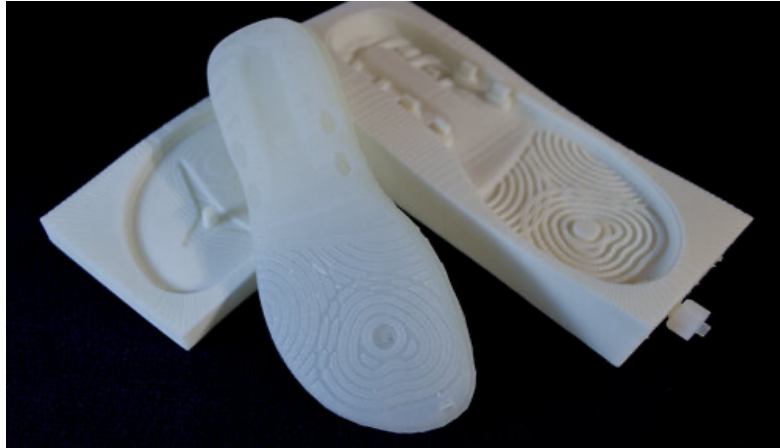
Figure 2.1: Illustration of Silicone Casting of Shoes' sole [33]. (Source: https://www.estructur3d.io/photos ).
