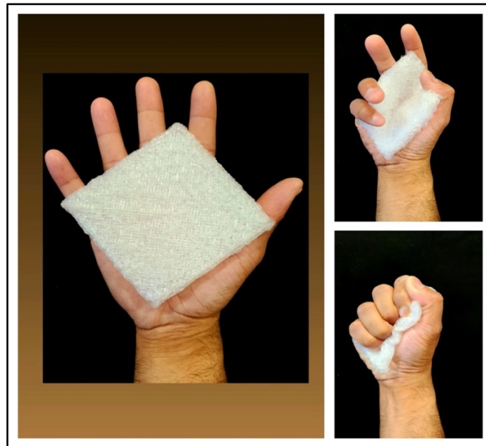
Figure 1.2: Soft part fabricated by Silicone Whipping Additive Manufacturing (SWAM), illustrating the flexibility of silicone-made soft structure. The deformation of the part being squeezed is reversible. (Source: By Gurkamal Saggi)
