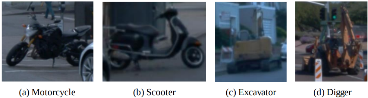
Figure 3.5: Examples of Waymo objects - type ⑦ OOD. A PointPillars detector trained on KITTI recognizes these objects mostly as cars. Some instances of Motorcycle and Scooter are recognized as Cyclist and Pedestrian. Excavator is sometimes recognized as a group of Pedestrians.
