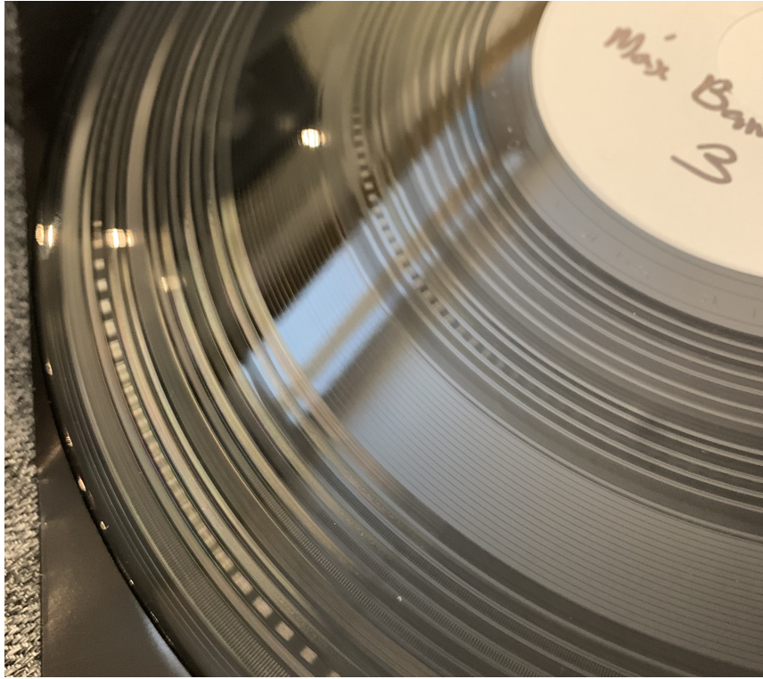
Figure 2.1: An image of the test record, note the two sets of signals and the large space of silence in between them. The transition track is visible as the spaced out grooves in the middle of the record connecting the two sets of signals.
