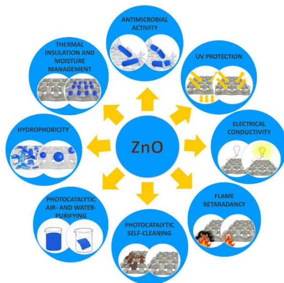
Figure 2.6. Schematic representation of functionalities that ZnO can add to textiles [14].
