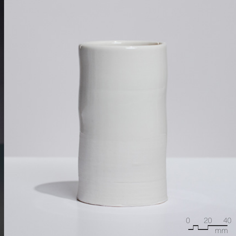
Figure 4.3.21 Clear liner glaze on Laguna Frost, fired to cone 6, 90mm x 90mm x 180mm, extrusion variability.
