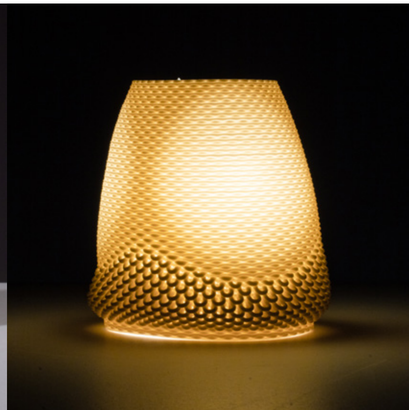
Figure 4.3.30 Unglazed Laguna Frost, fired to cone 6, 90mm x 90mm x 90mm, 2 layer sequence (x2), extrusion variability.
