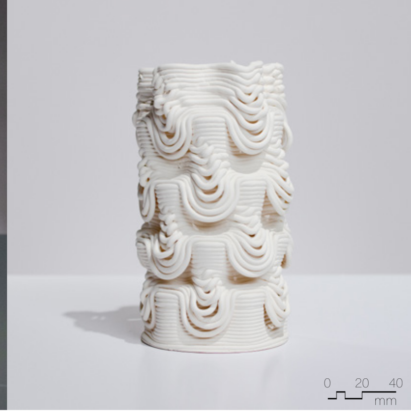
Figure 4.6.29 Unglazed PSH-515, fired to cone 04, 90mm x 90mm x 180mm, 20 layer sequence (x2).
