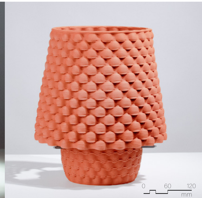
Figure 4.5.36 Unglazed PSH-425, fired to cone 06, 300mm x 300mm x 420mm, 11 layer sequence (x2).
