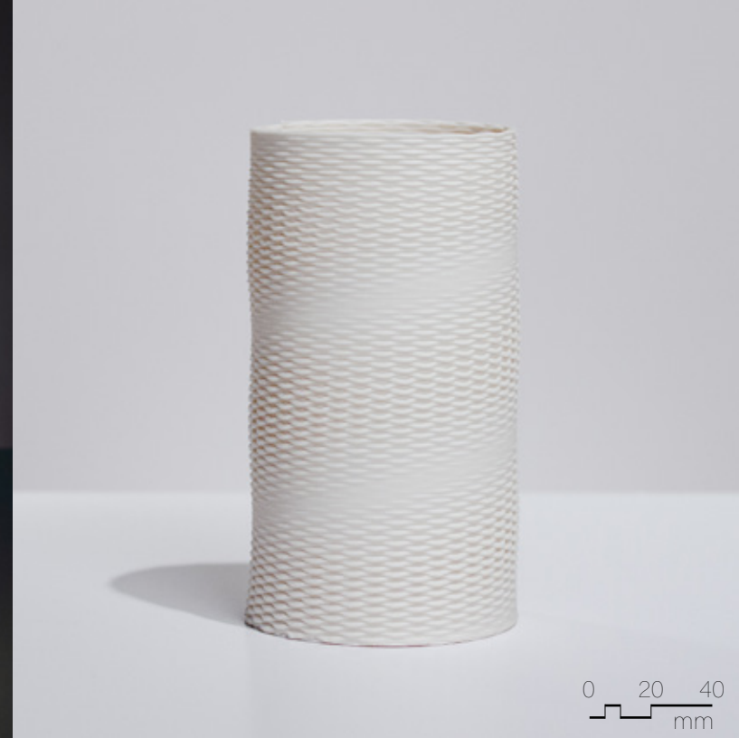
Figure 4.3.19 Clear liner glaze on Laguna Frost, fired to cone 6, 90mm x 90mm x 180mm, 2 layer sequence (x2), extrusion variability.
