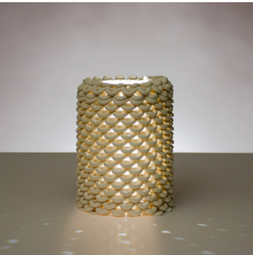
Figure 4.4.37 Unglazed PSH-515, fired to cone 04, 90mm x 90mm x 150mm, 3 layer sequence (x2), inverted loop pattern.
