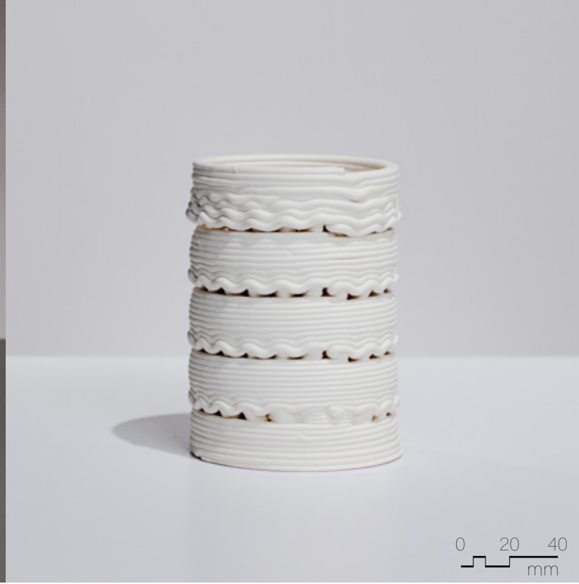
Figure 4.5.29 Unglazed PSH-515, fired to cone 04, 90mm x 90mm x 140mm, 13 layer sequence.
