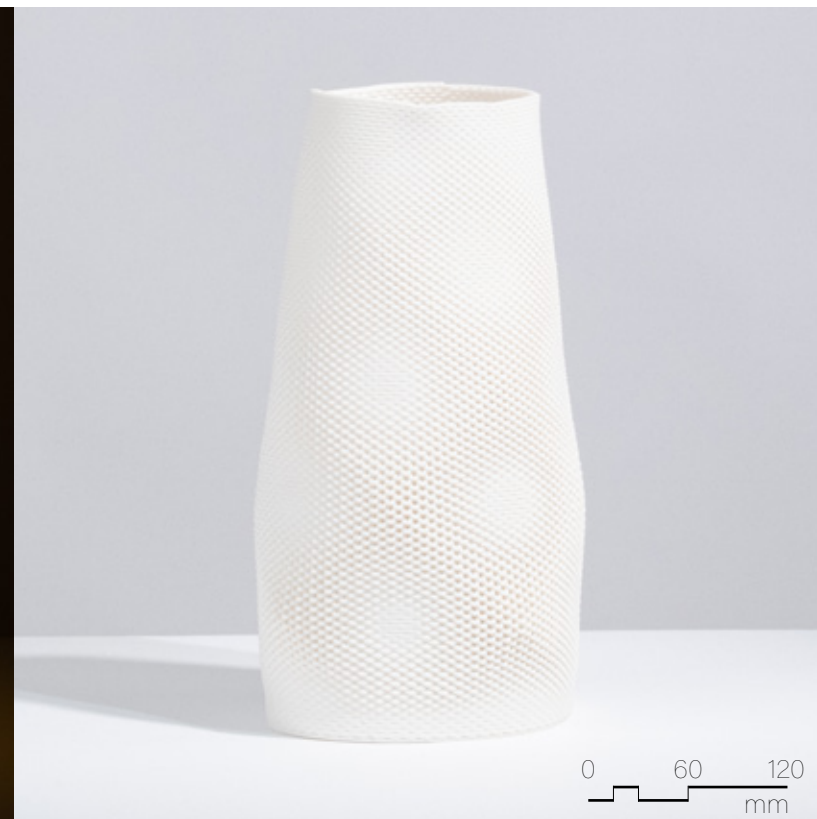
Figure 4.3.32 Unglazed Laguna Frost, fired to cone 6, 160mm x 160mm x 300mm, 2 layer sequence (x2), extrusion variability.
