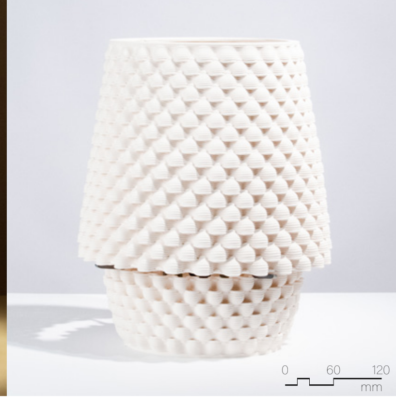
Figure 4.5.37 Unglazed PSH-516, fired to cone 04, 300mm x 300mm x 420mm, 11 layer sequence (x2).
