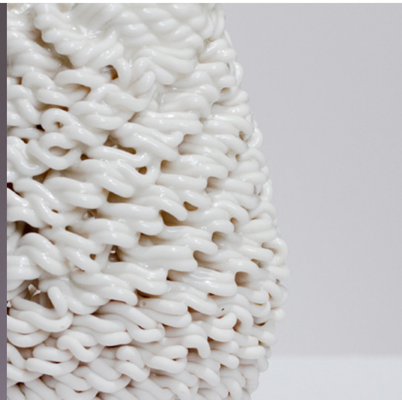
Figure 2.5.3 Tool path variability across a porcelain clay body (100mm x 100mm x 200mm).
