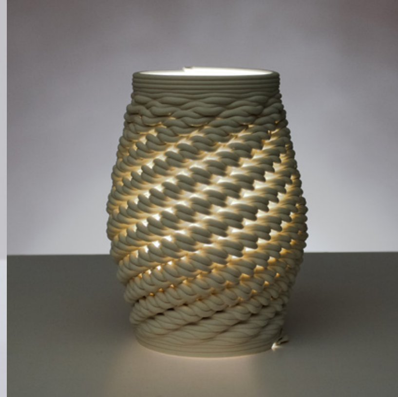
Figure 4.4.42 Unglazed PSH-515, fired to cone 04, 90mm x 90mm x 180mm, 2 layer sequence (x4), spiral pattern.
