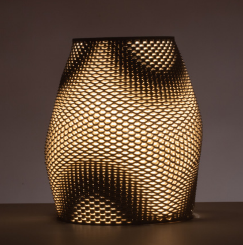
Figure 4.4.52 Unglazed PSH-516, fired to cone 04, 230mm x 230mm x 340mm, 3 layer sequence (x2).
