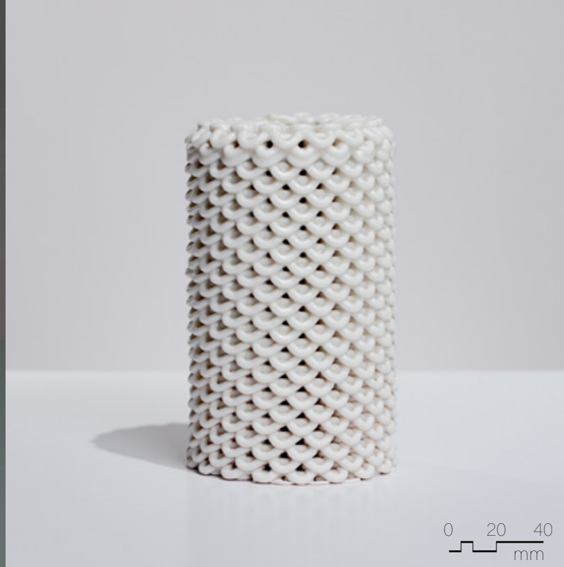
Figure 4.4.36 Unglazed PSH-515, fired to cone 04, 90mm x 90mm x 180mm, 3 layer sequence (x2), inverted loop pattern.
