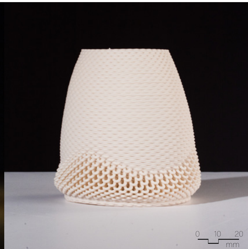
Figure 4.3.30 Unglazed Laguna Frost, fired to cone 6, 90mm x 90mm x 90mm, 2 layer sequence (x2), extrusion variability.
