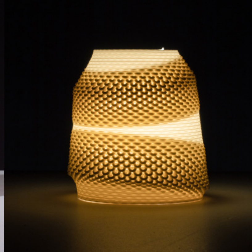
Figure 4.3.29 Unglazed Laguna Frost, fired to cone 6, 90mm x 90mm x 90mm, 2 layer sequence (x2), extrusion variability.
