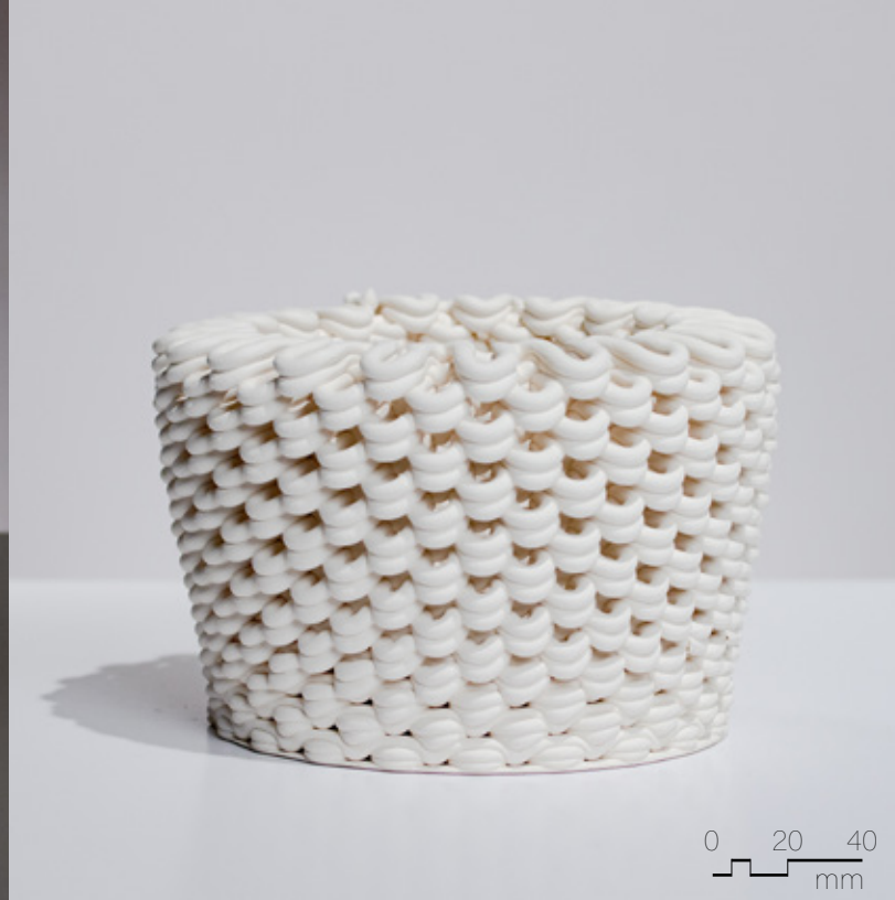
Figure 4.4.32 Unglazed PSH-515, fired to cone 04, 130mm x 130mm x 120mm, 2 layer sequence (x2).
