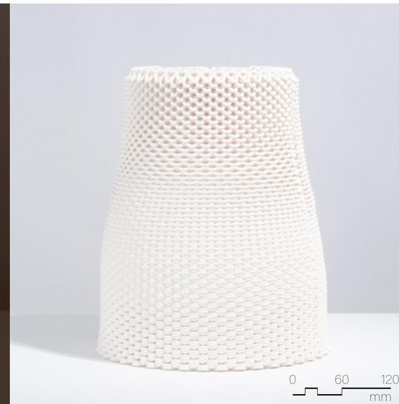
Figure 4.4.63 Unglazed PSH-516, fired to cone 04, 280mm x 280mm x 350mm, 3 layer sequence (x2).
