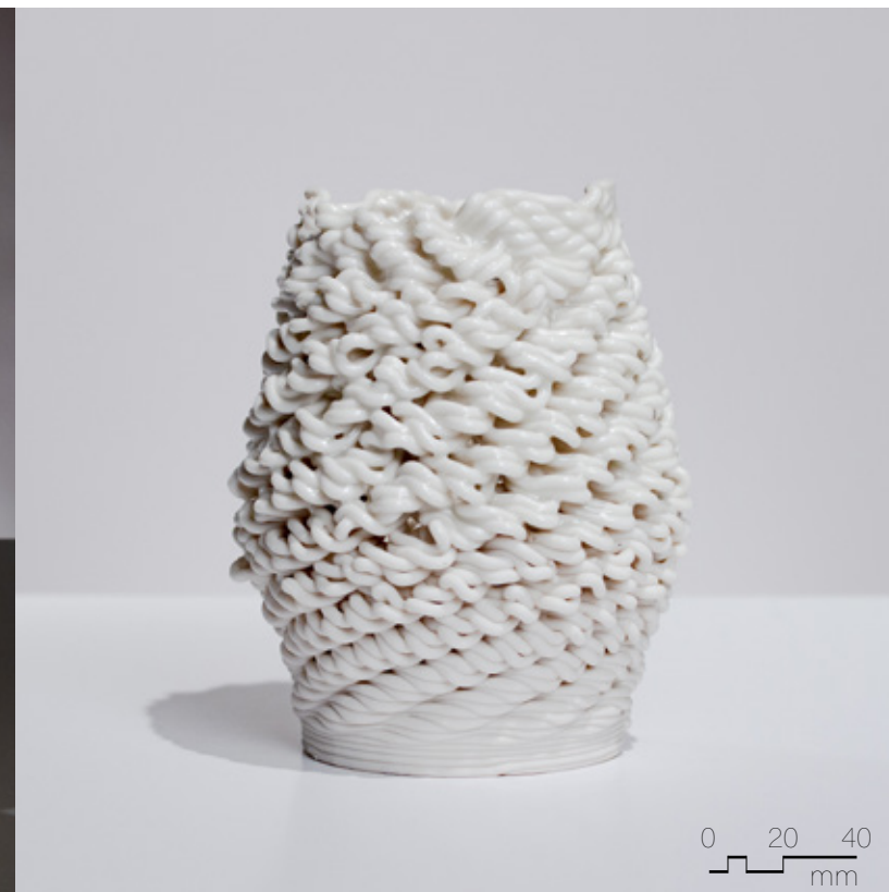
Figure 4.4.41 Clear Linear glaze on Polar Ice, fired to cone 6, 90mm x 90mm x 180mm, 2 layer sequence (x4), spiral pattern.
