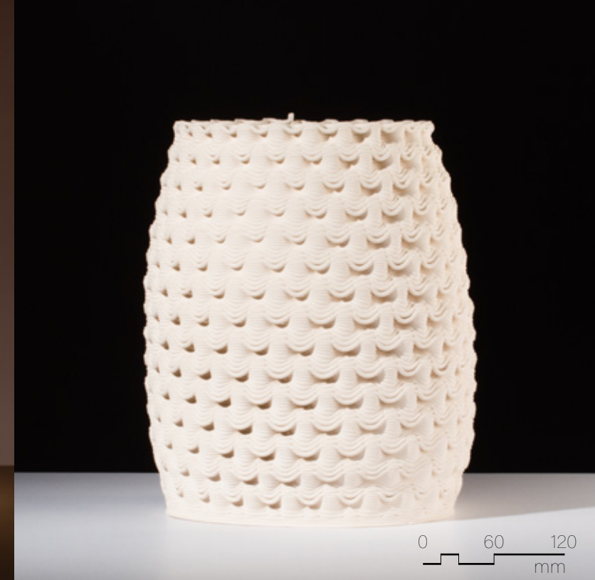
Figure 4.5.35 Unglazed PSH-516, fired to cone 04, 230mm x 230mm x 340mm, 11 layer sequence (x2), inverted scoop pattern.
