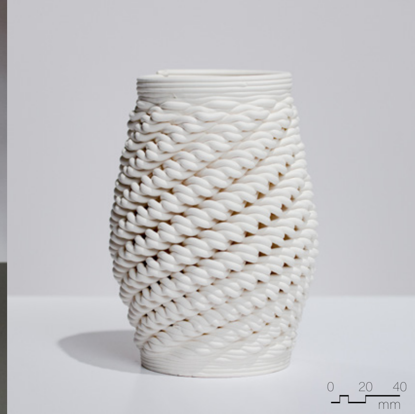
Figure 4.4.42 Unglazed PSH-515, fired to cone 04, 90mm x 90mm x 180mm, 2 layer sequence (x4), spiral pattern.
