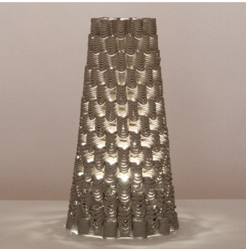
Figure 4.6.36 Unglazed PSH Dark Granite, fired to cone 6, 200mm x 200mm x 380mm, 20 layer sequence (x2).
