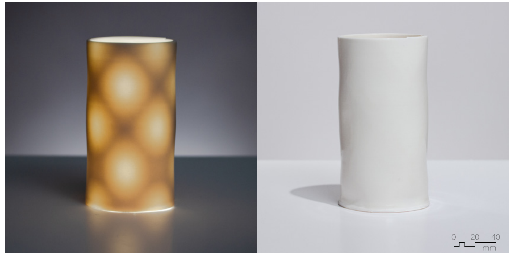
Figure 4.3.18 Clear liner glaze on Laguna Frost, fired to cone 6, 90mm x 90mm x 180mm, extrusion variability.
