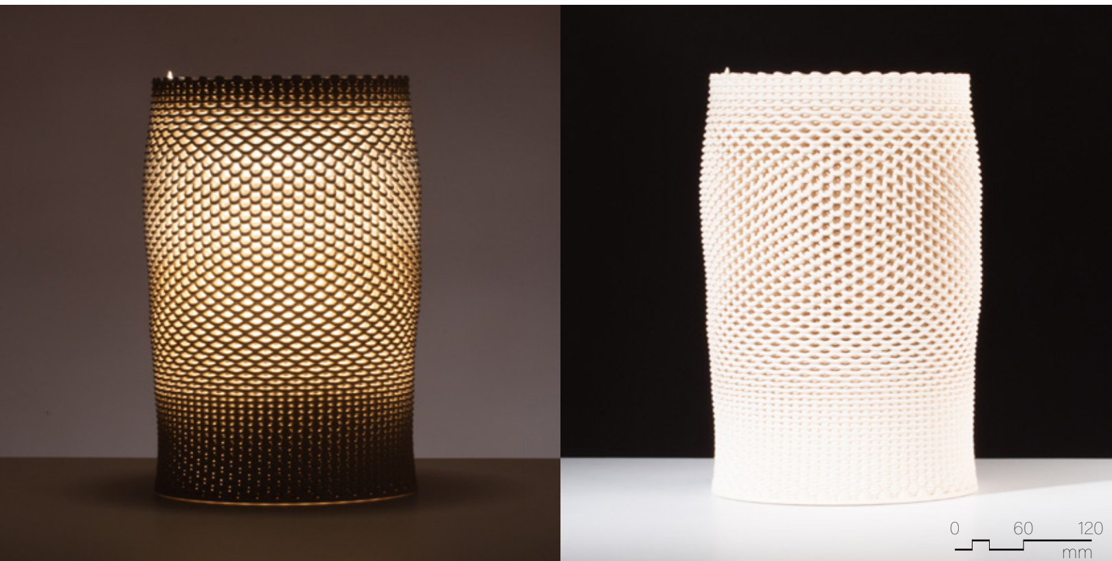
Figure 4.4.57 Unglazed PSH-516, fired to cone 04, 260mm x 260mm x 400mm, 3 layer sequence (x2).
