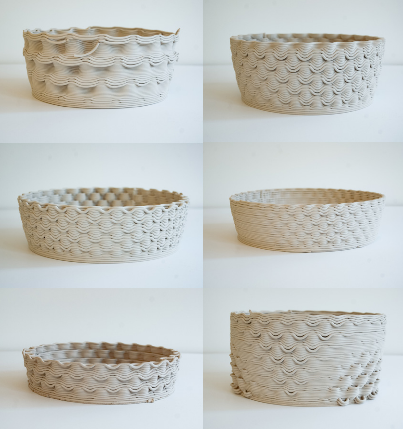
Figure 4.5.23 Rapid iteration of aperture sizes and scoop profiles. The final iteration in the sequence incorporates both inward and outward-facing scoops.
