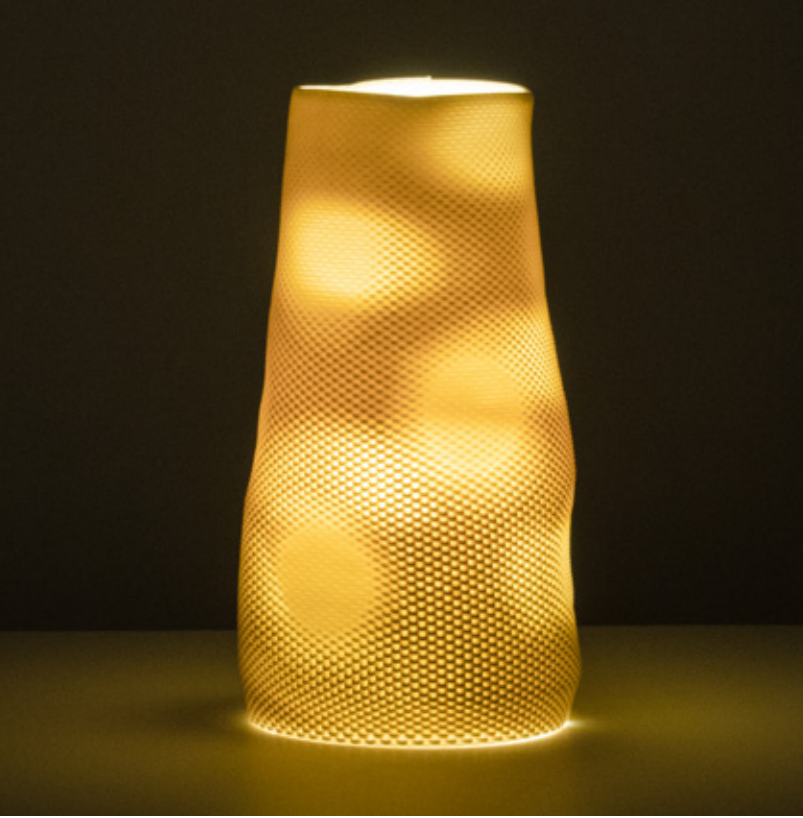
Figure 4.3.31 Clear liner glaze on Polar Ice, fired to cone 6, 160mm x 160mm x 300mm, 2 layer sequence (x2), extrusion variability.
