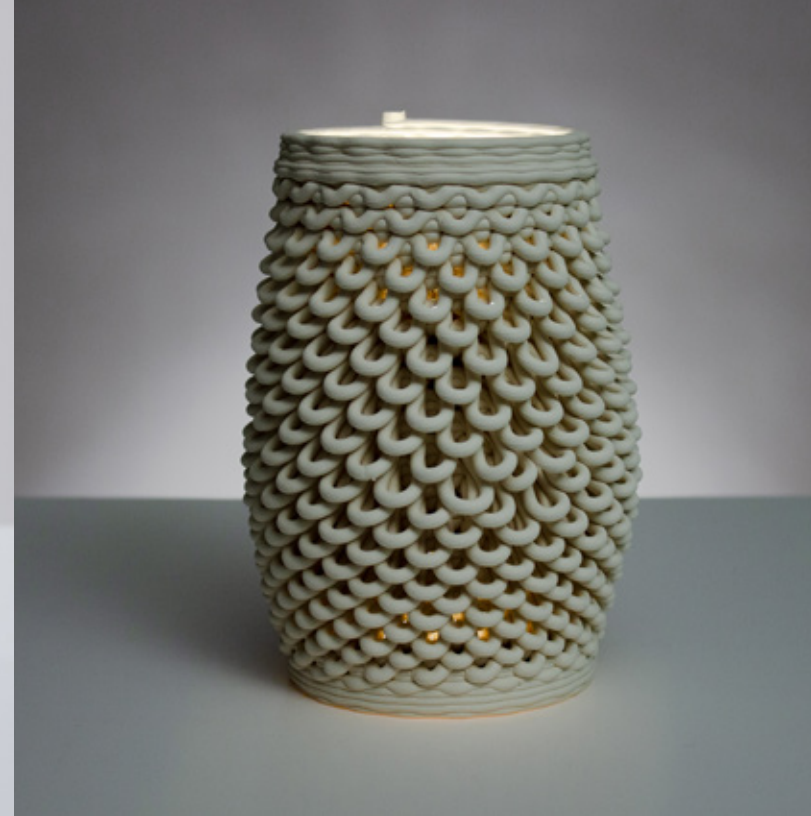
Figure 4.4.34 Unglazed PSH-515, fired to cone 04, 90mm x 90mm x 180mm, 3 layer sequence (x2).
