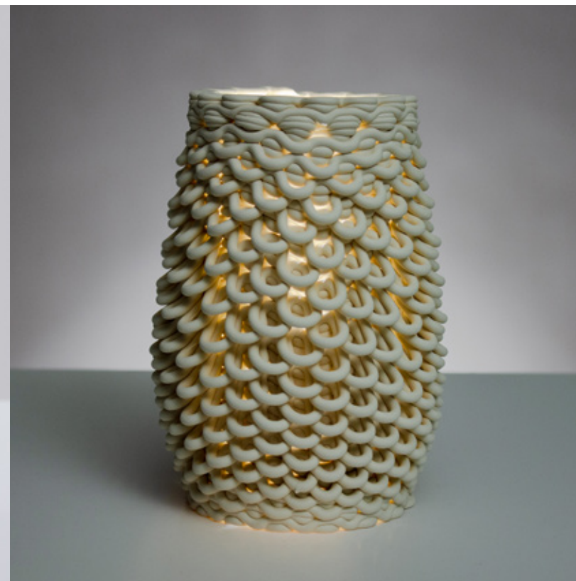
Figure 4.4.35 Unglazed PSH-515, fired to cone 04, 90mm x 90mm x 180mm, 3 layer sequence (x2), non-planar pattern.
