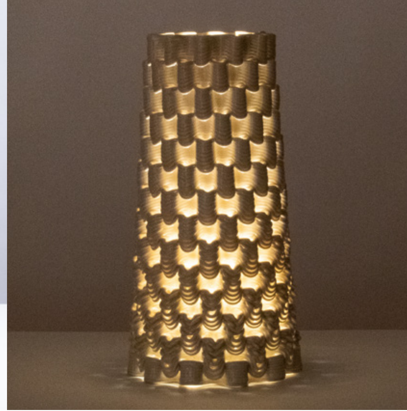
Figure 4.6.37 Clear liner glaze on PSH-515, fired to cone 6, 200mm x 200mm x 380mm, 20 layer sequence (x2).
