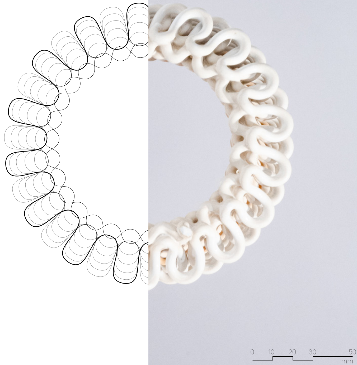
Figure 4.4.26 Loop pattern tool path plan (left) and physical print plan (right).
