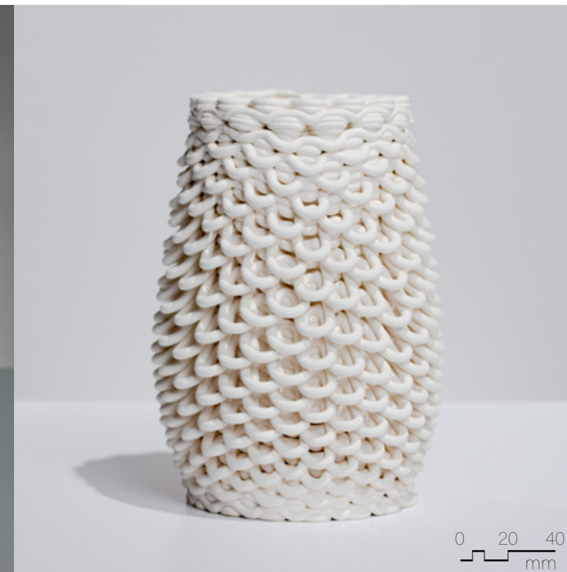
Figure 4.4.35 Unglazed PSH-515, fired to cone 04, 90mm x 90mm x 180mm, 3 layer sequence (x2), non-planar pattern.
