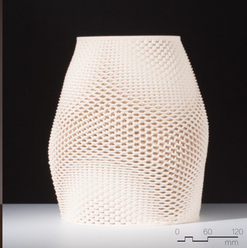
Figure 4.4.52 Unglazed PSH-516, fired to cone 04, 230mm x 230mm x 340mm, 3 layer sequence (x2).
