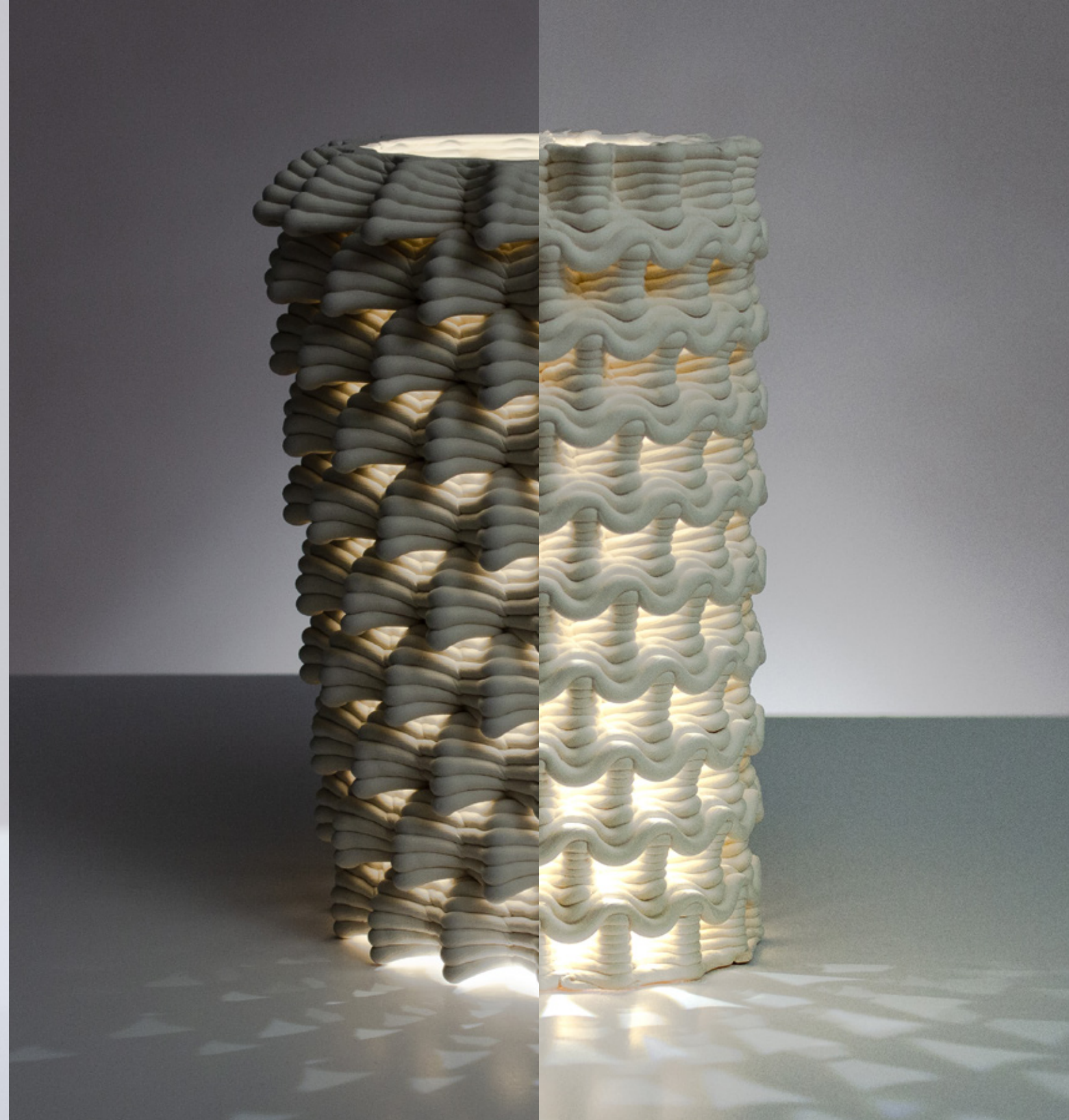
Figure 4.5.22 Two prints with identical print parameters, the only difference being the left print has inverted wave amplitudes.
