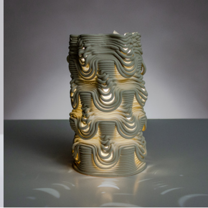
Figure 4.6.29 Unglazed PSH-515, fired to cone 04, 90mm x 90mm x 180mm, 20 layer sequence (x2).
