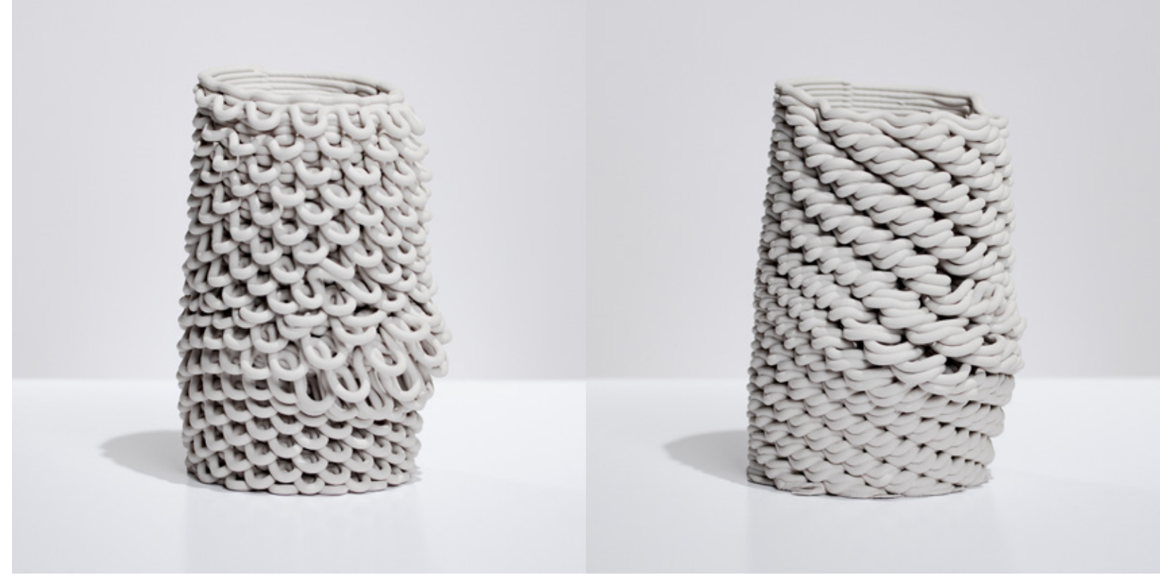
Figure 4.4.28 Non-planar looping print studies displaying deformation and reformation.
