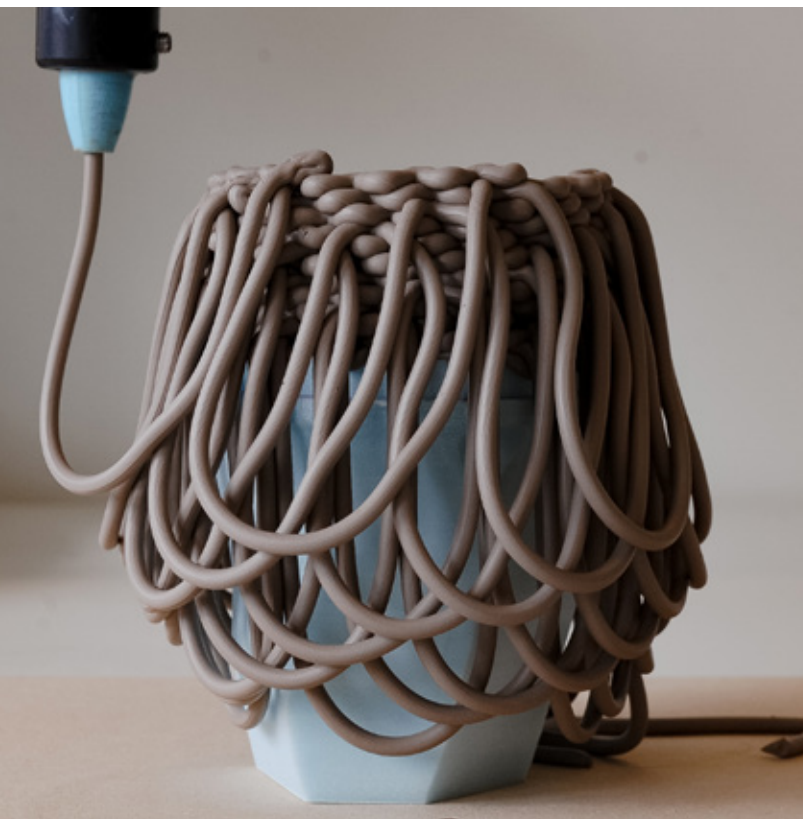
Figure 4.4.21 Oversized/Overhanging loop pattern print in progress (left) and illuminated (right).
