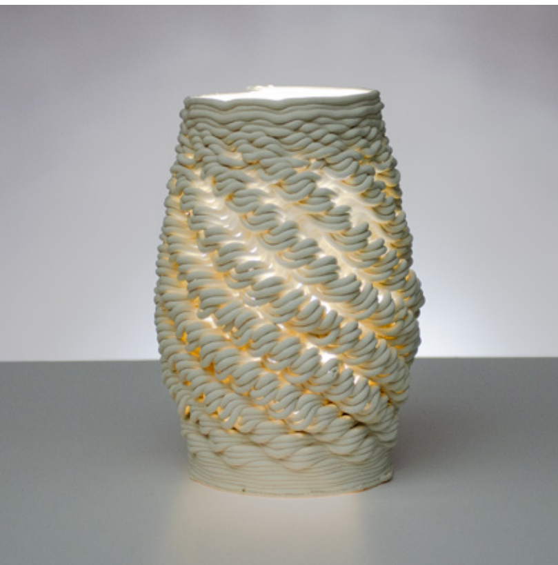
Figure 4.4.45 Unglazed PSH-515, fired to cone 04, 90mm x 90mm x 180mm, 3 layer sequence (x4), spiral pattern.
