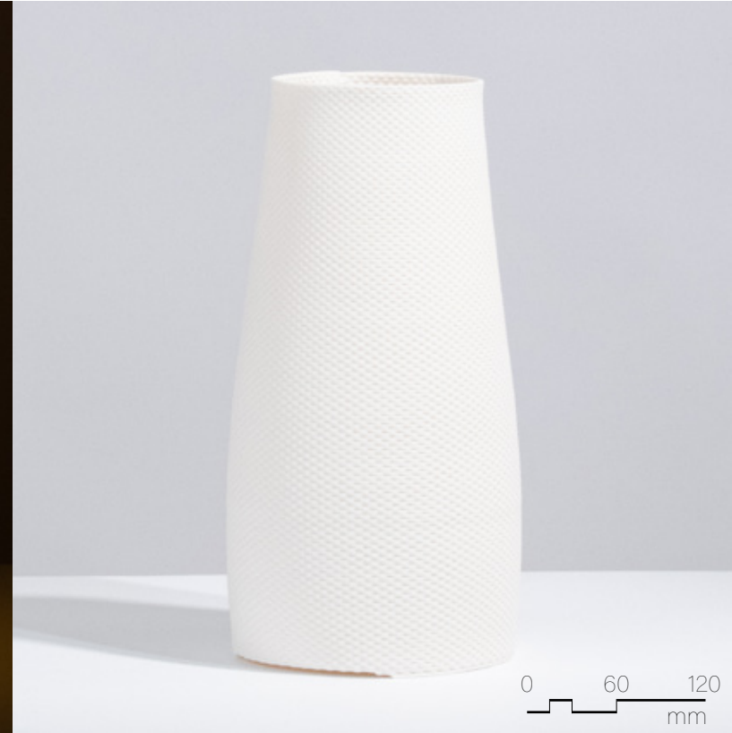
Figure 4.3.33 Unglazed Laguna Frost, fired to cone 6, 160mm x 160mm x 300mm, 2 layer sequence (x2), extrusion variability.
