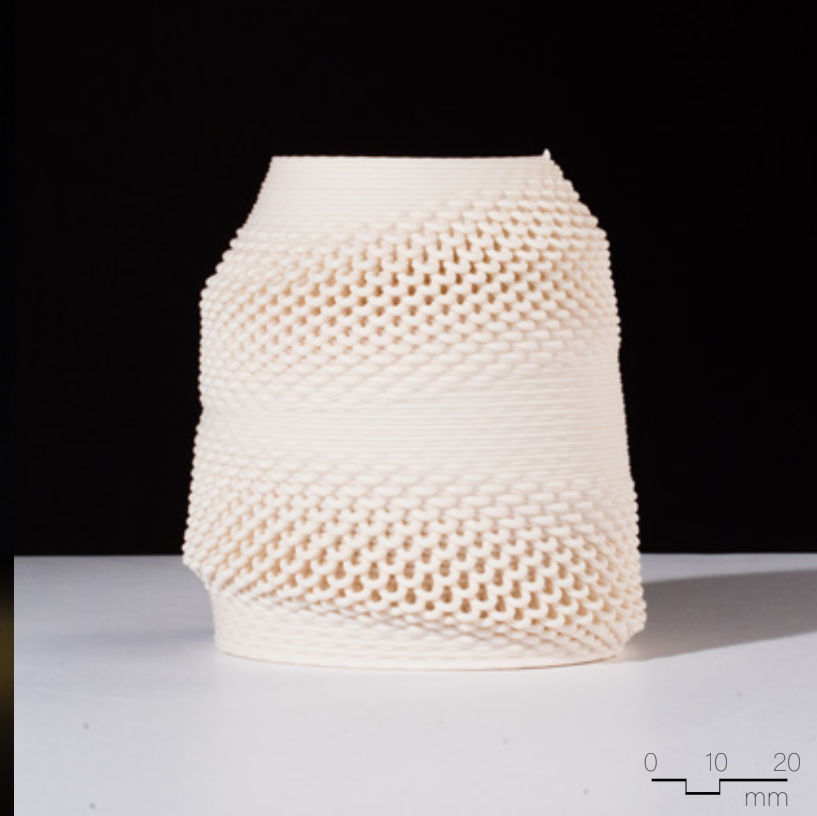
Figure 4.3.29 Unglazed Laguna Frost, fired to cone 6, 90mm x 90mm x 90mm, 2 layer sequence (x2), extrusion variability.
