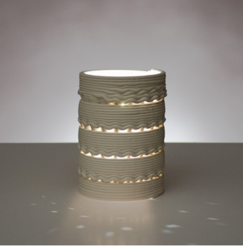
Figure 4.5.29 Unglazed PSH-515, fired to cone 04, 90mm x 90mm x 140mm, 13 layer sequence.
