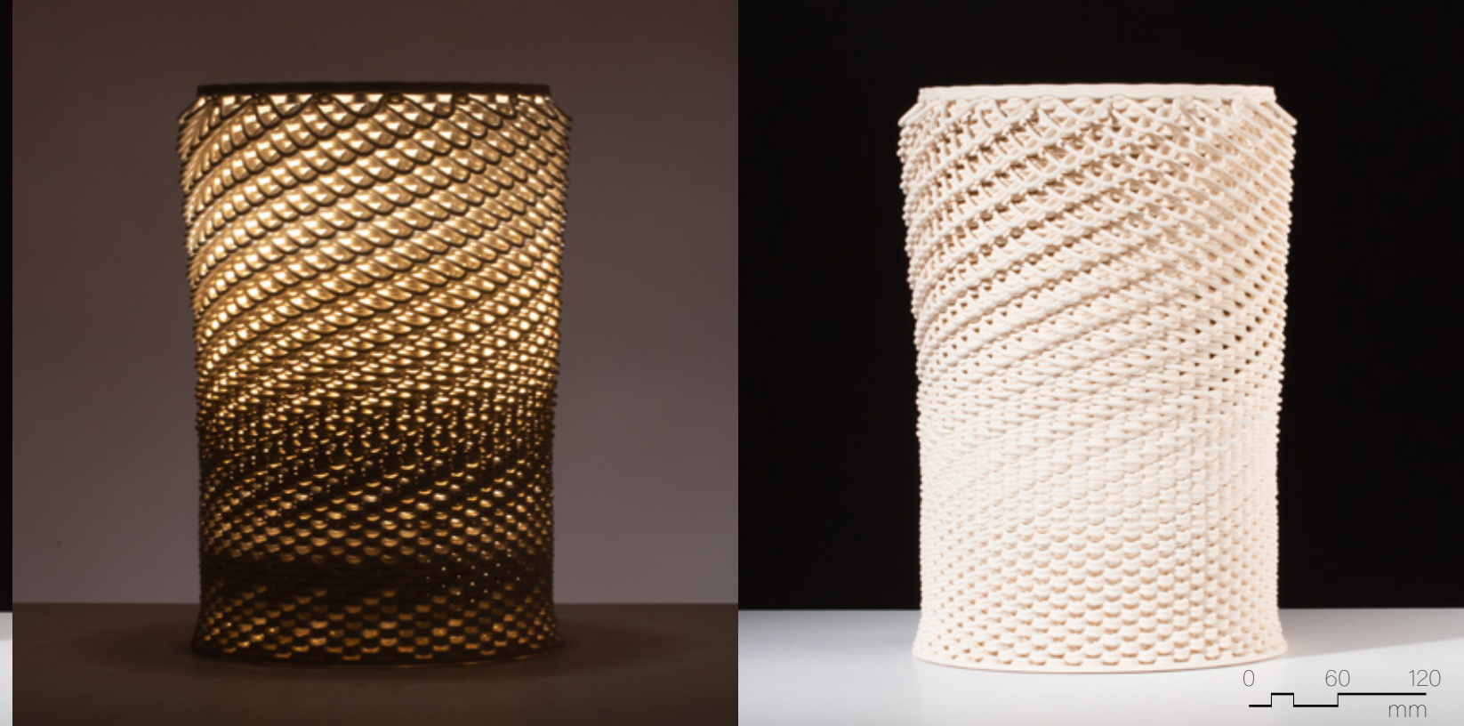
Figure 4.4.58 Unglazed PSH-516, fired to cone 04, 260mm x 260mm x 400mm, 3 layer sequence (x2).
