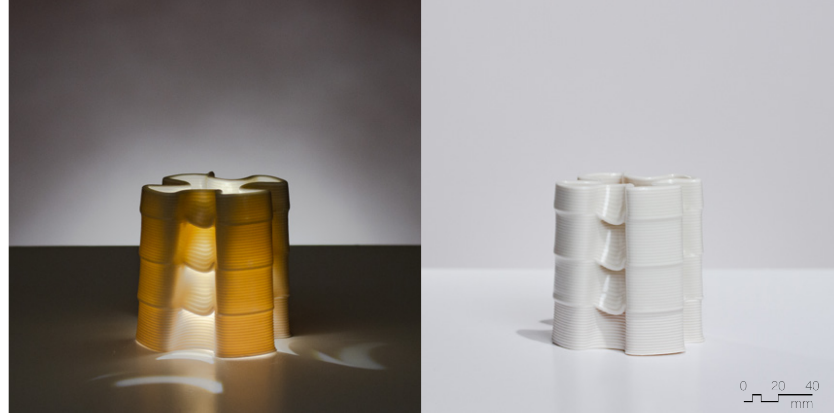
Figure 4.6.25 Clear Linear glaze on Polar Ice, fired to cone 6, 90mm x 90mm x 150mm, 21 layer sequence.
