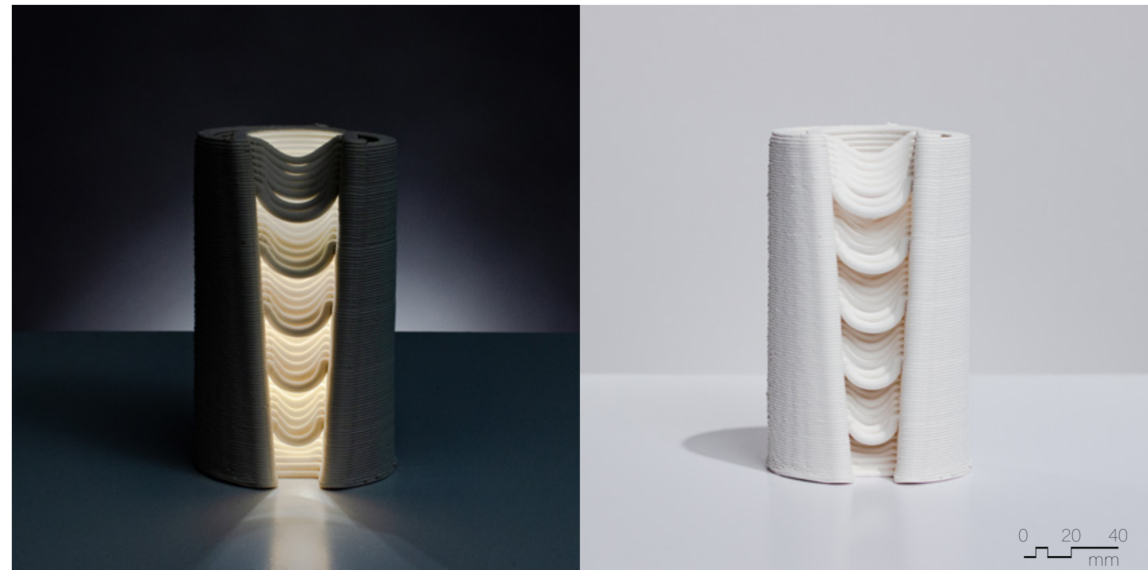
Figure 4.6.26 Unglazed PSH-515, fired to cone 04, 80mm x 80mm x 160mm, 18 layer sequence.
