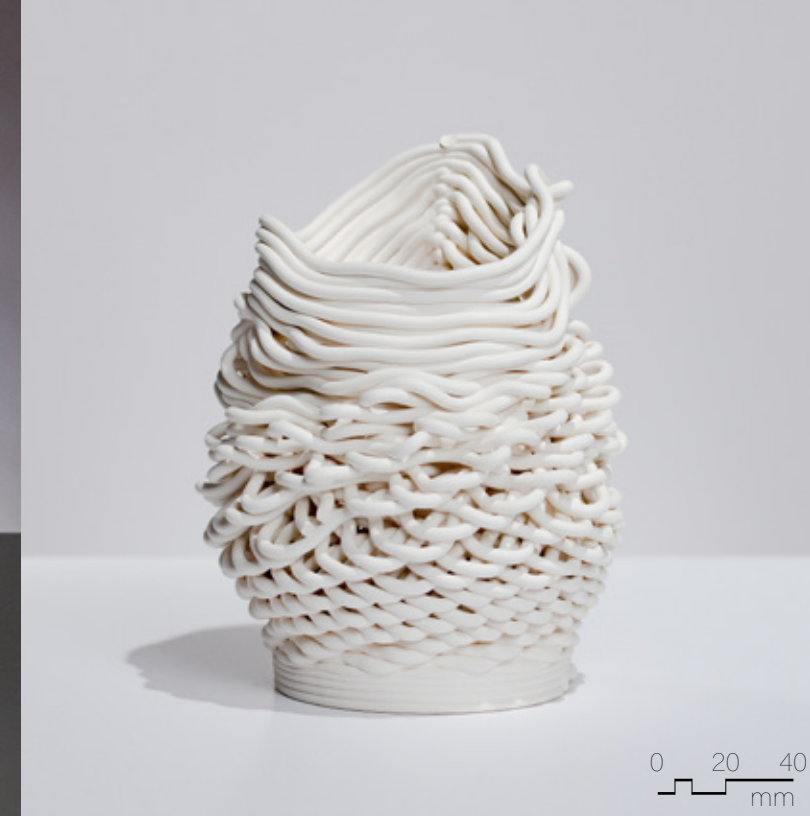
Figure 4.4.38 Unglazed PSH-515, fired to cone 04, 90mm x 90mm x 160mm, 3 layer sequence (x3), spiral pattern.
