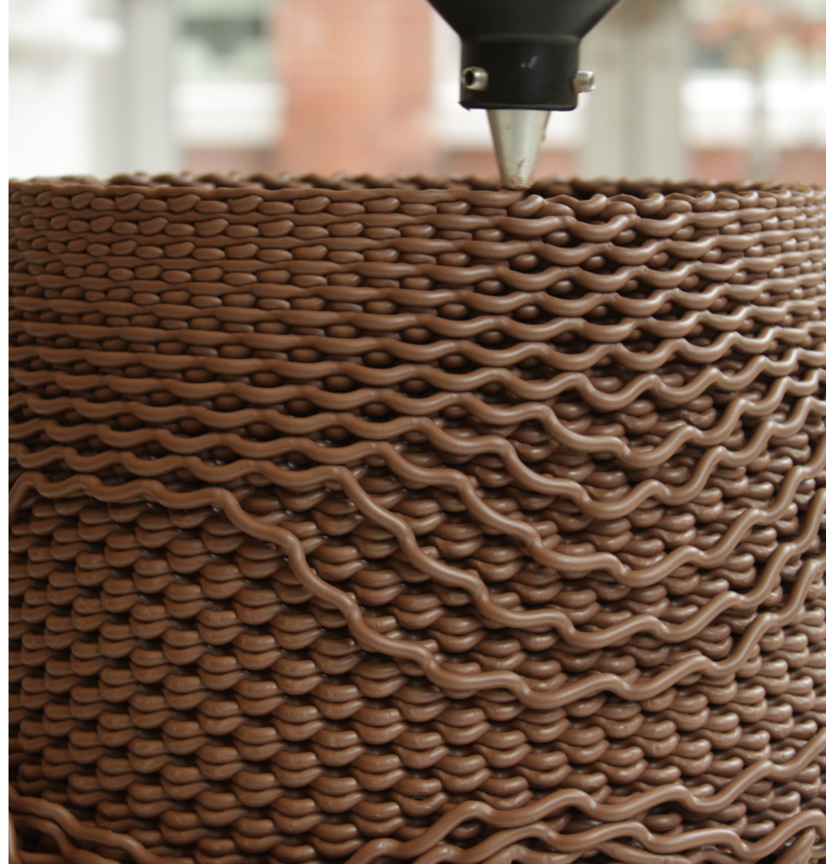
Figure 3.1.2 M prototype in terracotta, delaminating during printing.
