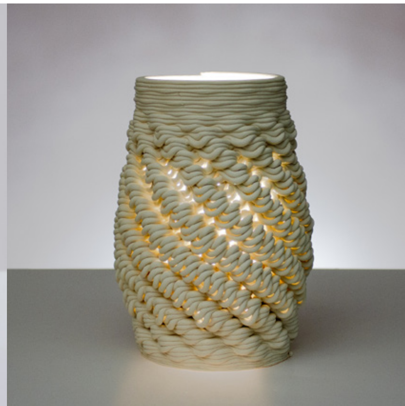
Figure 4.4.43 Unglazed PSH-515, fired to cone 04, 90mm x 90mm x 180mm, 3 layer sequence (x4), spiral pattern.
