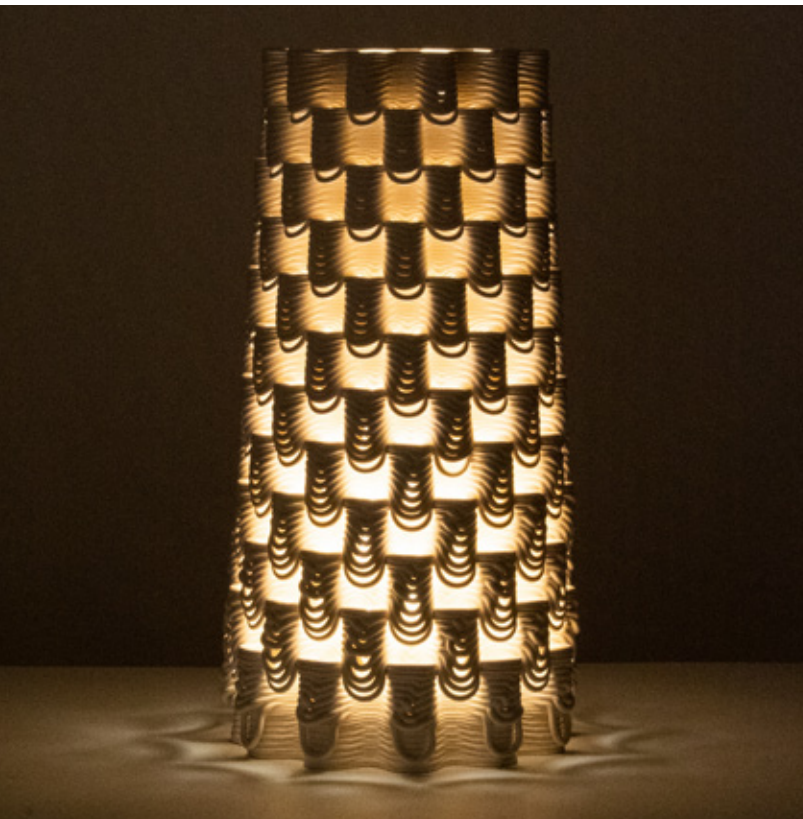
Figure 4.6.32 Unglazed PSH-515, fired to cone 04, 200mm x 200mm x 400mm, 20 layer sequence (x2).
