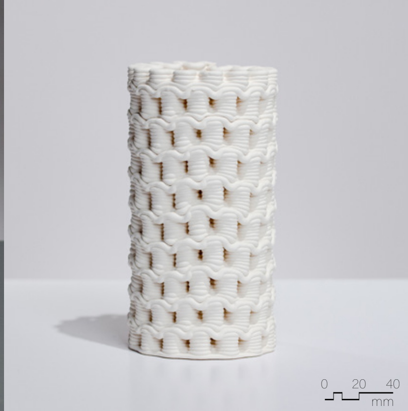
Figure 4.5.33 Unglazed PSH-515, fired to cone 04, 90mm x 90mm x 180mm, 8 layer sequence (x2), non-planar pattern.
