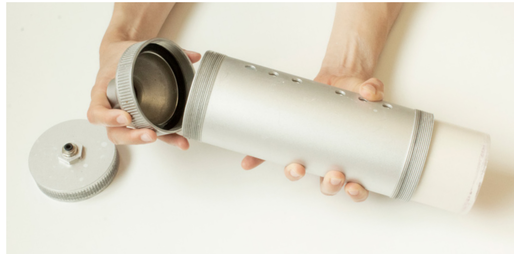
Figure 3.1.6 Prepping the clay cartridge for pressurization via. compressed air.
