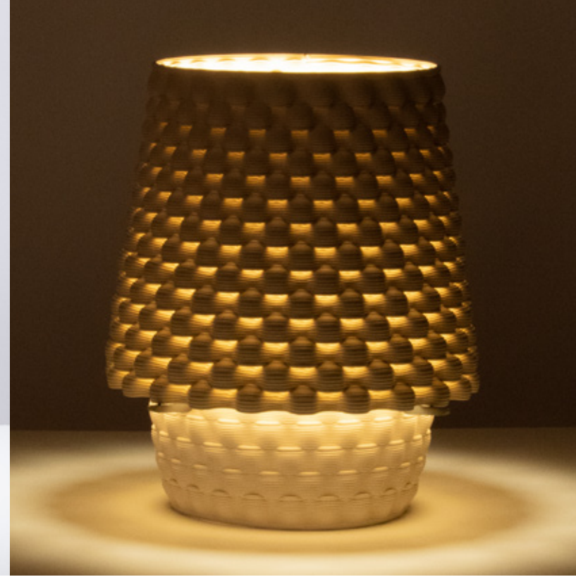
Figure 4.5.39 Unglazed PSH-516, fired to cone 6, 300mm x 300mm x 420mm, 11 layer sequence (x2).
