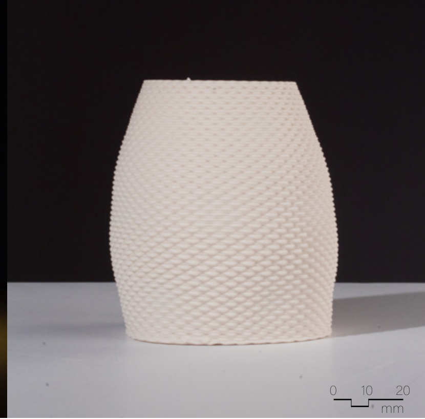
Figure 4.3.25 Unglazed Laguna Frost, fired to cone 6, 90mm x 90mm x 90mm, 2 layer sequence (x2), extrusion variability.
