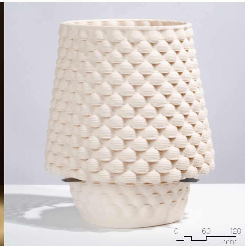
Figure 4.5.38 Unglazed PSH-516, fired to cone 6, 300mm x 300mm x 420mm, 11 layer sequence (x2).
