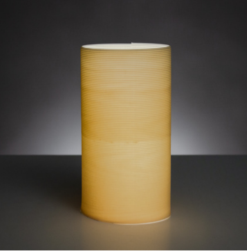
Figure 4.3.23 Unglazed Laguna Frost, fired to cone 6, 90mm x 90mm x 180mm, 2 layer sequence (x2), extrusion variability.
