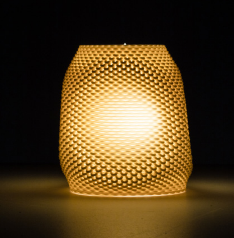
Figure 4.3.27 Unglazed Laguna Frost, fired to cone 6, 90mm x 90mm x 90mm, 2 layer sequence (x2), extrusion variability.
