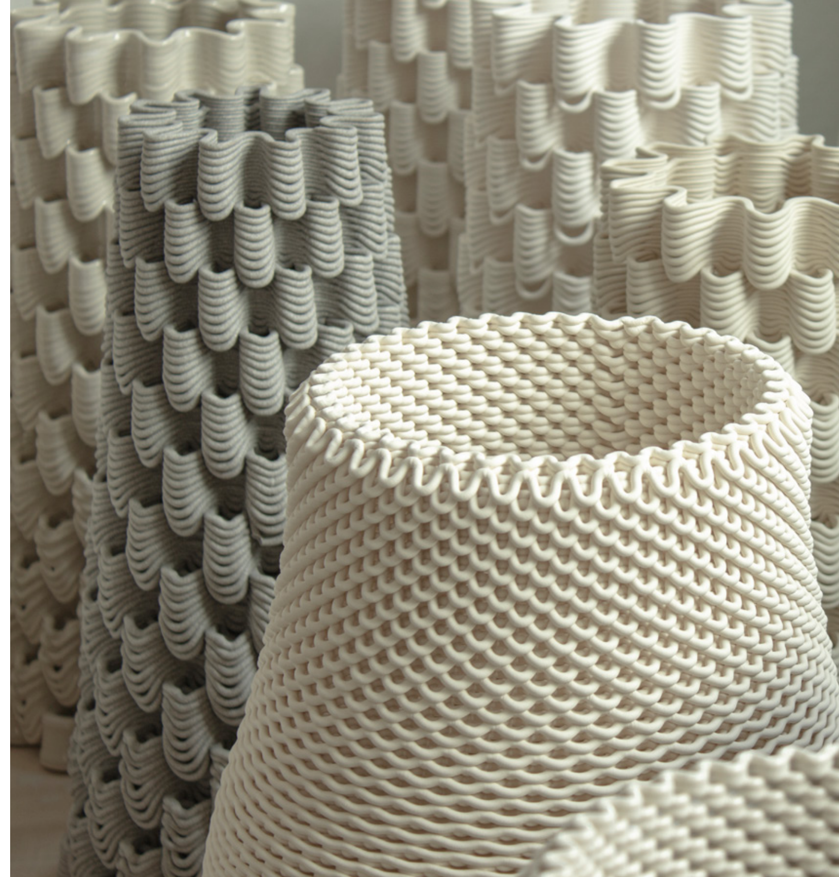
Figure 3.4.12 Full scale prototypes utilizing porous tool paths generated in grasshopper.
