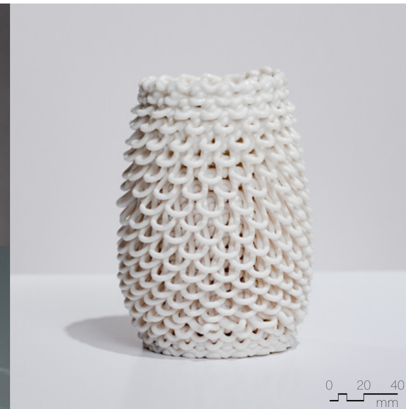
Figure 4.4.39 Clear Linear glaze on Polar Ice, fired to cone 6, 90mm x 90mm x 180mm, 3 layer sequence (x2).
