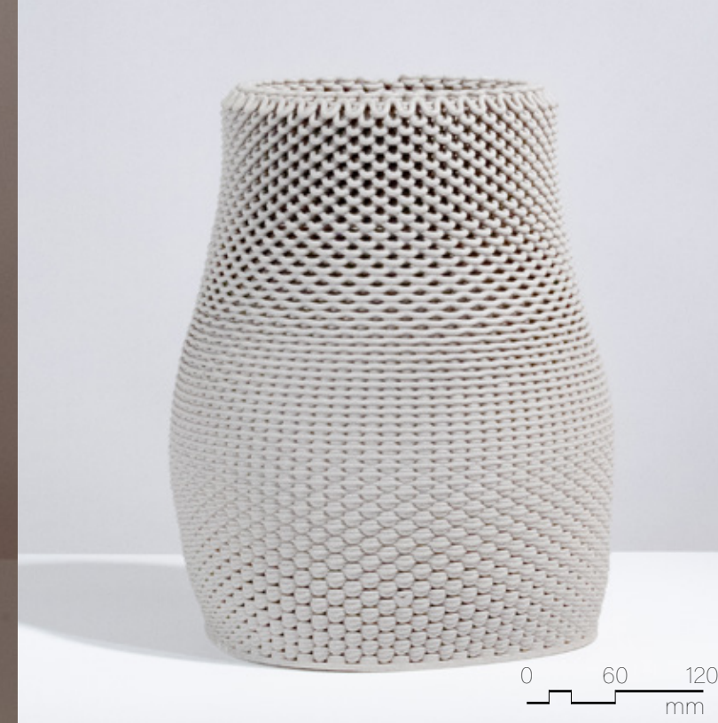
Figure 4.4.62 Unglazed PSH Dark Granite, fired to cone 6, 280mm x 280mm x 350mm, 3 layer sequence (x2).
