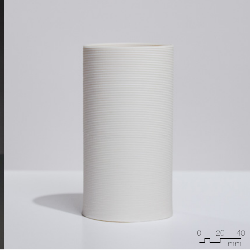
Figure 4.3.23 Unglazed Laguna Frost, fired to cone 6, 90mm x 90mm x 180mm, 2 layer sequence (x2), extrusion variability.
