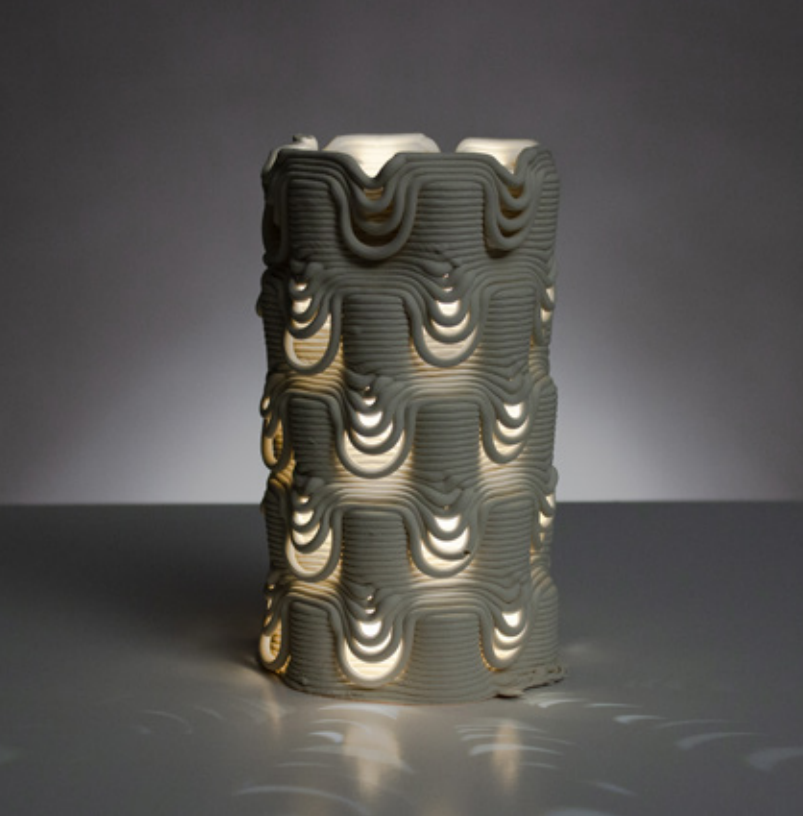
Figure 4.6.31 Unglazed PSH-515, fired to cone 04, 90mm x 90mm x 180mm, 20 layer sequence (x2).
