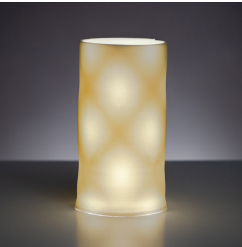
Figure 4.3.24 Clear liner glaze on Polar Ice, fired to cone 6, 90mm x 90mm x 80mm, extrusion variability.
