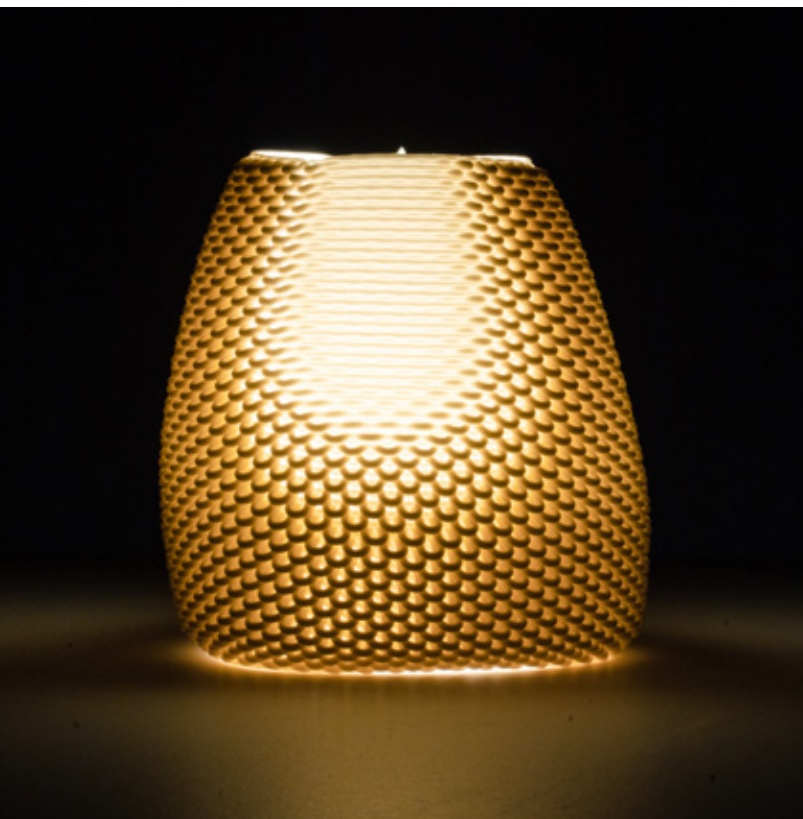
Figure 4.3.28 Unglazed Laguna Frost, fired to cone 6, 90mm x 90mm x 90mm, 2 layer sequence (x2), extrusion variability.
