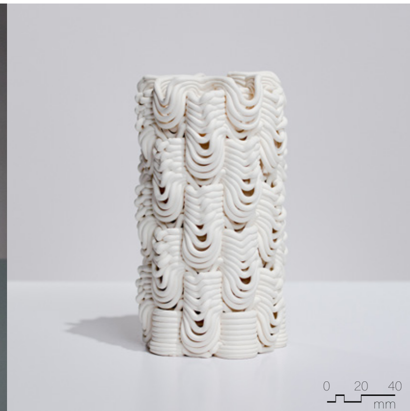
Figure 4.6.30 Unglazed PSH-515, fired to cone 04, 90mm x 90mm x 180mm, 16 layer sequence (x2).
