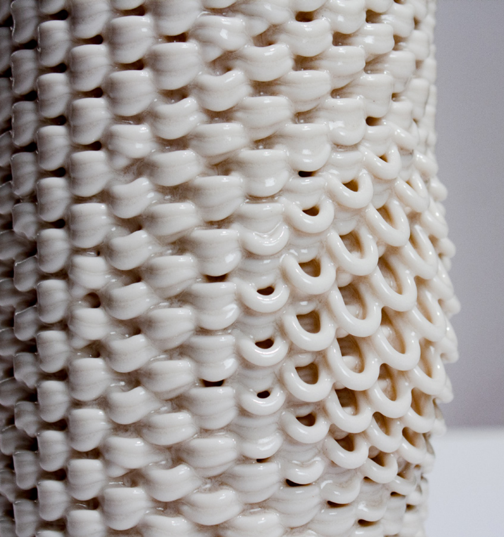
Figure 2.6.7 Porcelain light screen detail (100mm x 100mm x 200mm), extruded using the Lutum 4 using a 3mm diameter nozzle.
