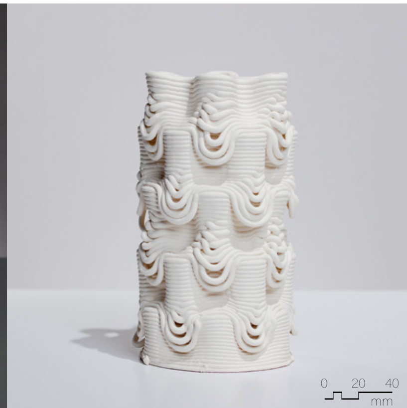
Figure 4.6.28 Unglazed PSH-515, fired to cone 04, 90mm x 90mm x 180mm, 16 layer sequence (x2).
