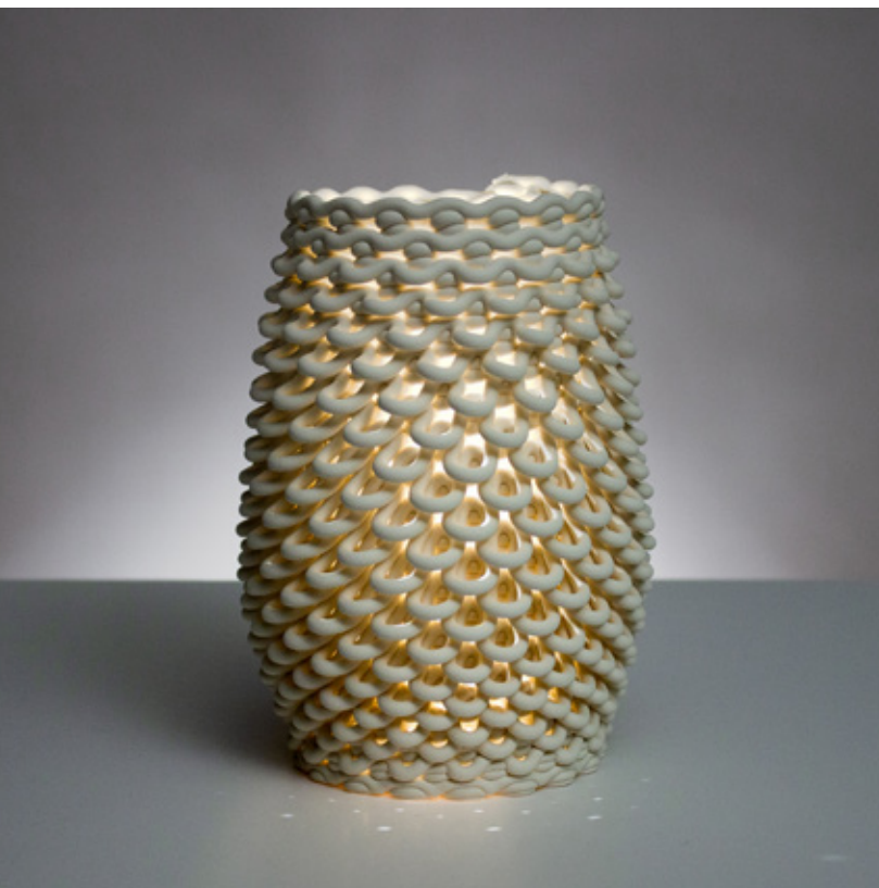
Figure 4.4.33 Unglazed PSH-515, fired to cone 04, 90mm x 90mm x 180mm, 3 layer sequence (x2).
