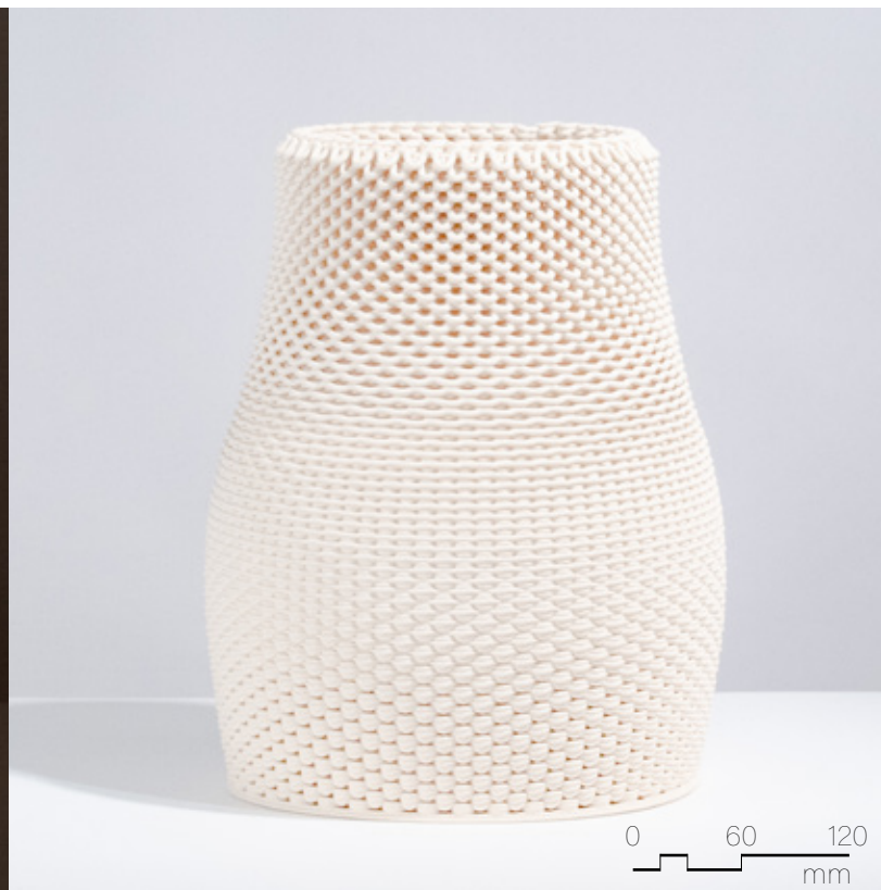
Figure 4.4.61 Unglazed PSH-516, fired to cone 04, 280mm x 280mm x 350mm, 3 layer sequence (x2).
