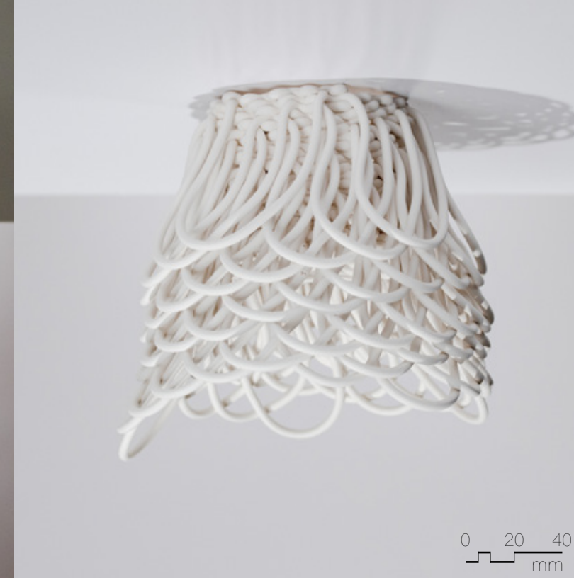
Figure 4.4.46 Unglazed PSH-515, fired to cone 04, 90mm x 90mm x 150mm, 3 layer sequence (x3), hanging loops, spiral pattern.
