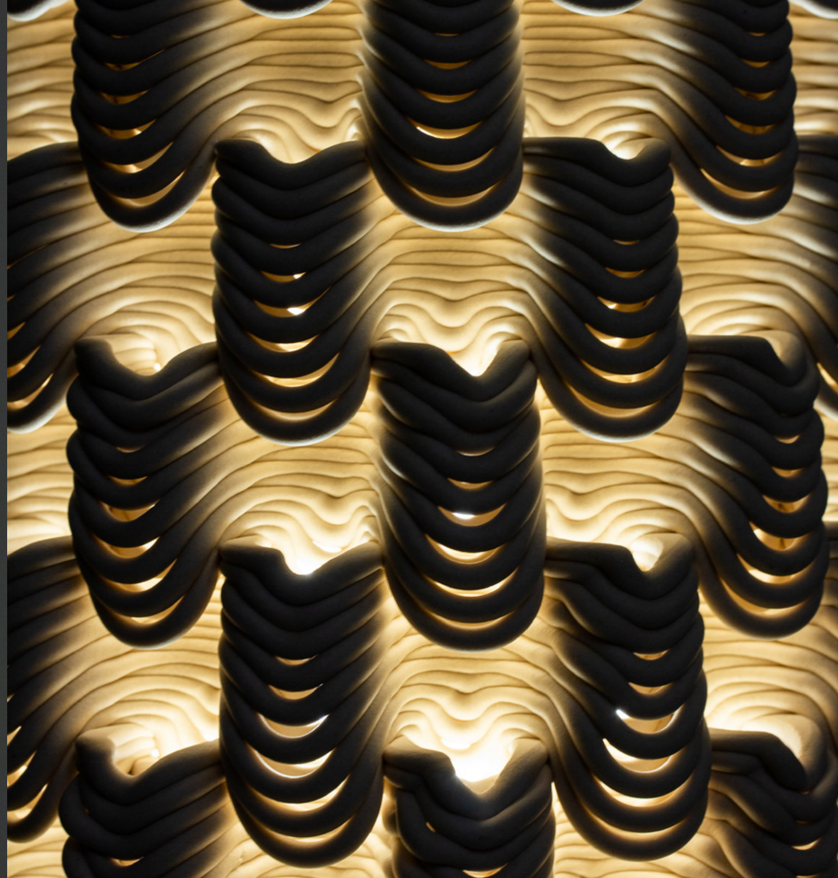
Figure 4.6.21 Illuminated 'XL' prototype, light shelf detail.
