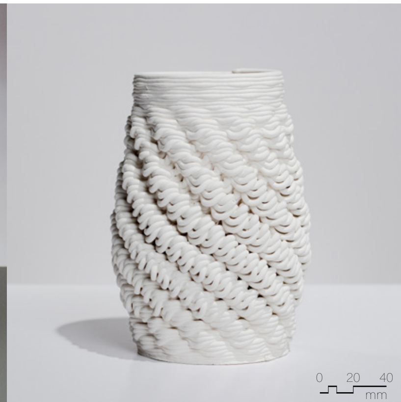
Figure 4.4.43 Unglazed PSH-515, fired to cone 04, 90mm x 90mm x 180mm, 3 layer sequence (x4), spiral pattern.
