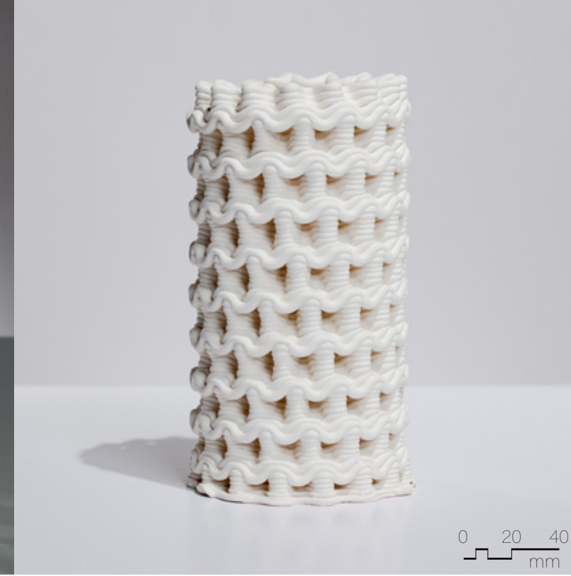
Figure 4.5.31 Unglazed PSH-515, fired to cone 04, 90mm x 90mm x 180mm, 8 layer sequence (x3), spiral scoop pattern.
