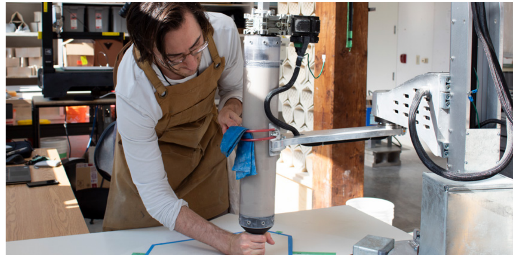
Figure 3.1.4 Attaching a loaded cartridge to the printer armature.
