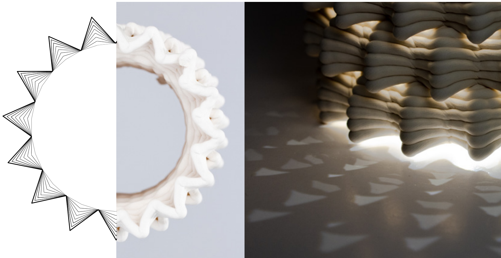
Figure 4.5.25 Angular scoop pattern (above) produces triangular light dappling effect. Angular inverted scoop pattern (below) produces reversed triangular light dappling effect.
