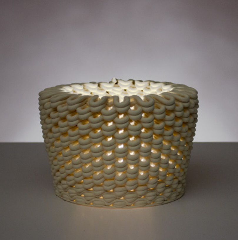
Figure 4.4.32 Unglazed PSH-515, fired to cone 04, 130mm x 130mm x 120mm, 2 layer sequence (x2).
