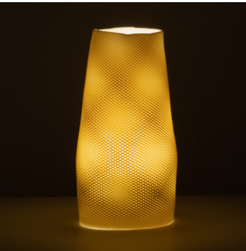
Figure 4.3.32 Unglazed Laguna Frost, fired to cone 6, 160mm x 160mm x 300mm, 2 layer sequence (x2), extrusion variability.
