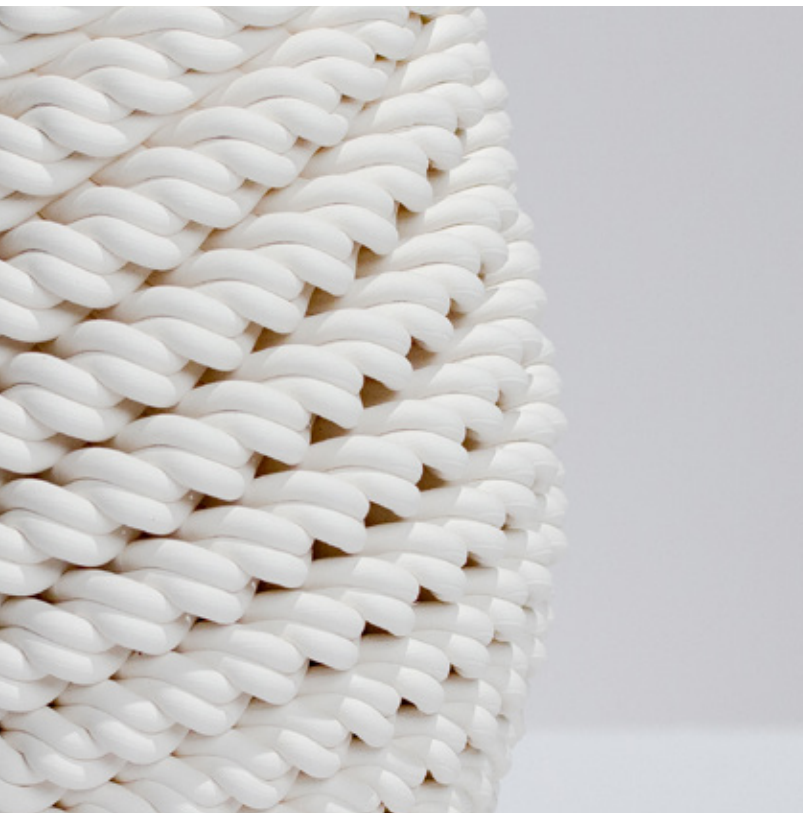
Figure 2.5.2 Tool path variability across a stoneware clay body (100mm x 100mm x 200mm).
