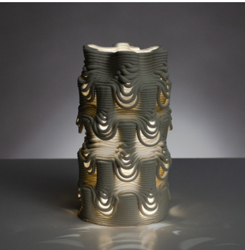
Figure 4.6.28 Unglazed PSH-515, fired to cone 04, 90mm x 90mm x 180mm, 16 layer sequence (x2).
