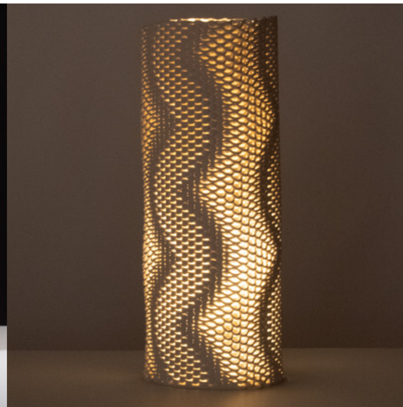
Figure 4.4.55 Unglazed PSH-516, fired to cone 04, 220mm x 220mm x mm, 3 layer sequence (x2).
