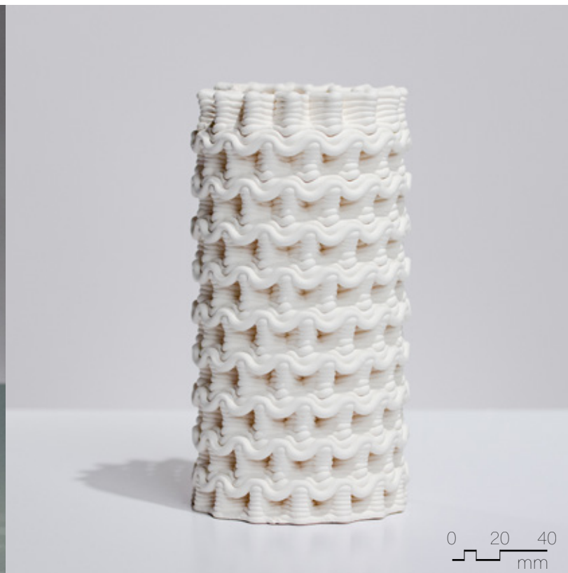
Figure 4.5.30 Unglazed PSH-515, fired to cone 04, 90mm x 90mm x 180mm, 8 layer sequence (x2).
