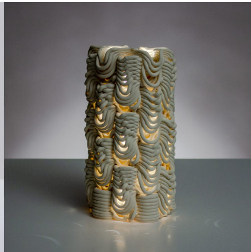
Figure 4.6.30 Unglazed PSH-515, fired to cone 04, 90mm x 90mm x 180mm, 16 layer sequence (x2).
