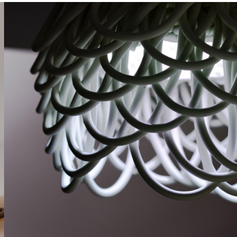
Figure 4.4.21 Oversized/Overhanging loop pattern print in progress (left) and illuminated (right).
