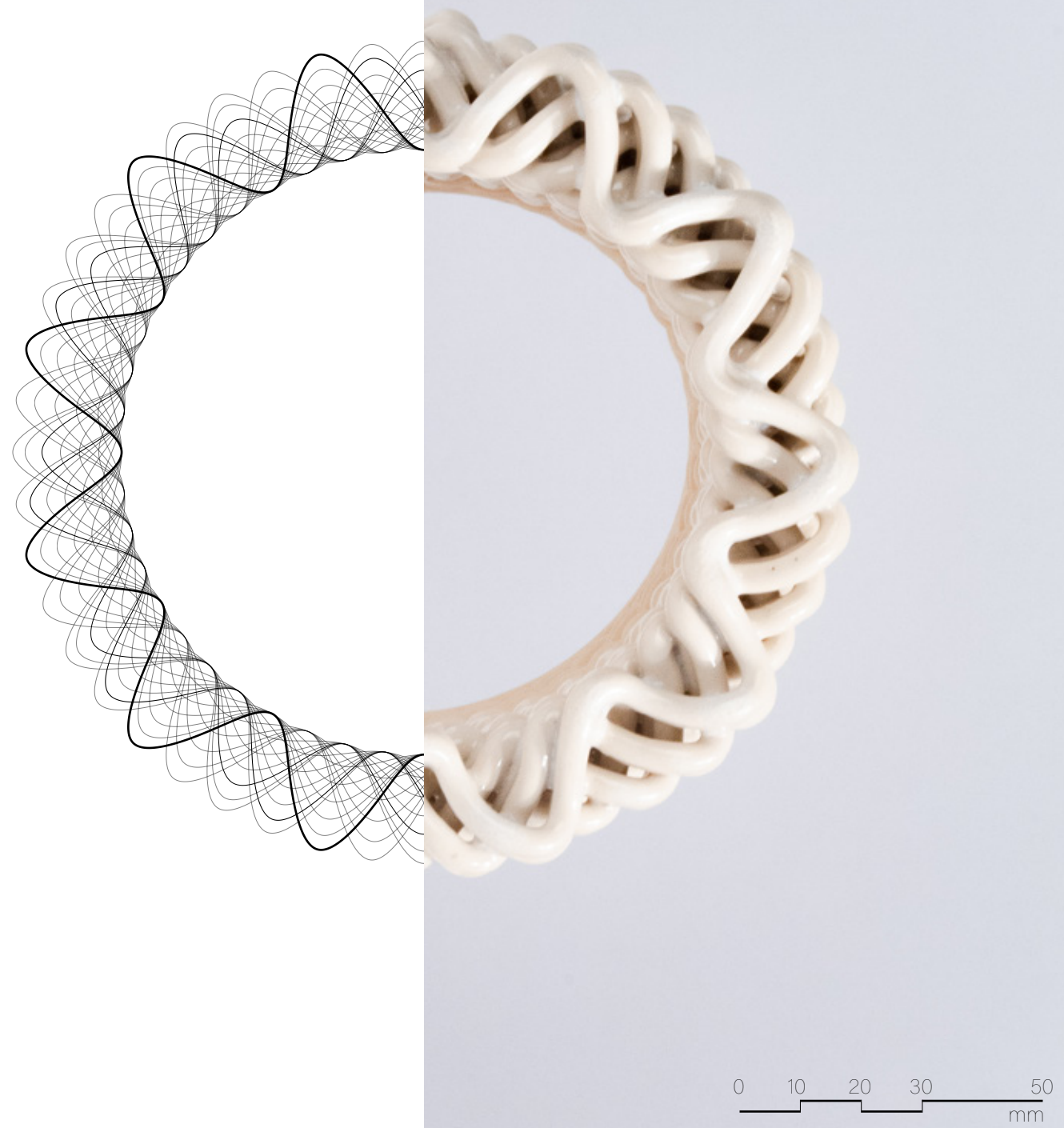
Figure 4.4.24 Spiral pattern tool path plan (left) and physical print plan (right).
