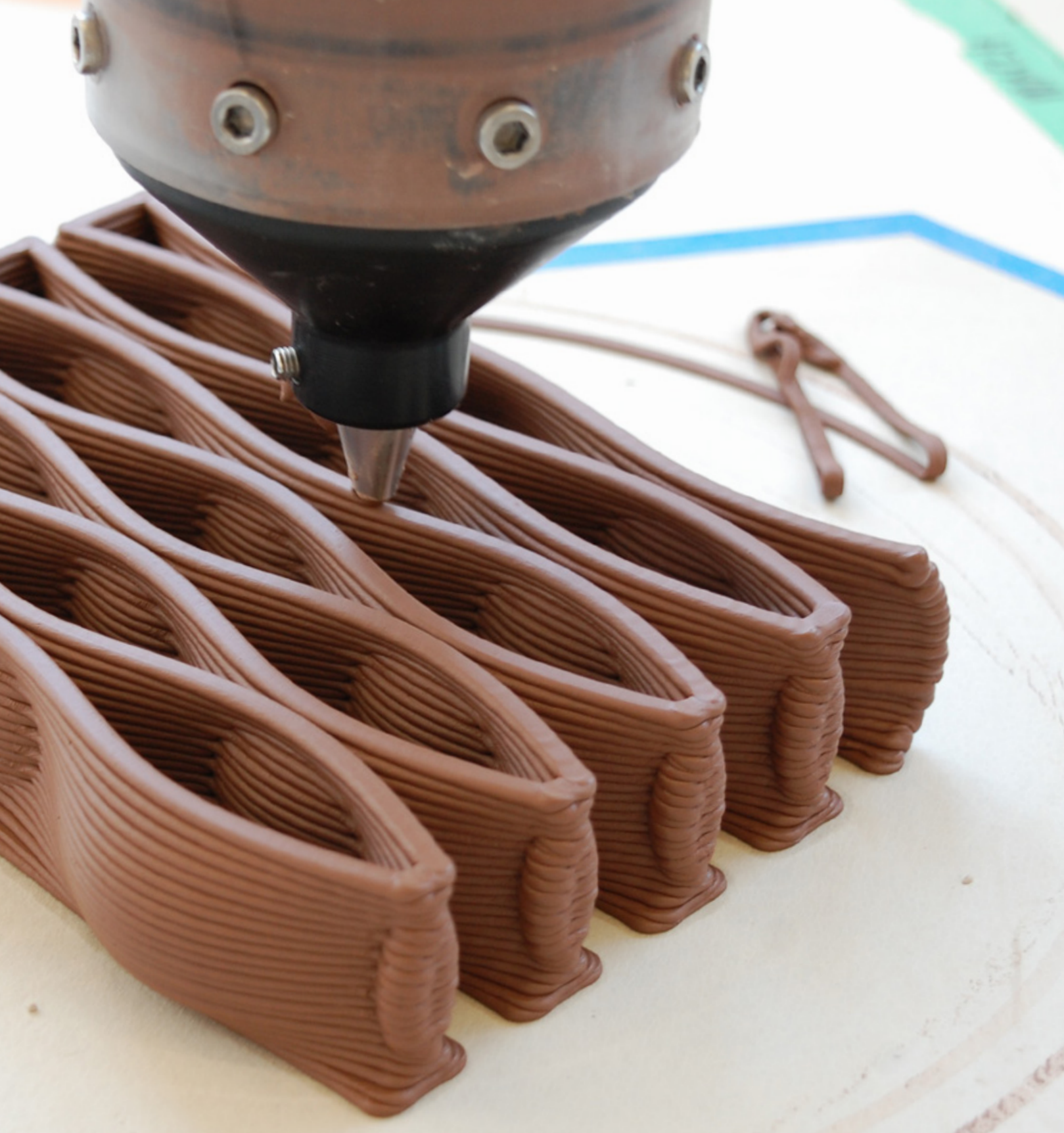
Figure 5.1.4 Bioinspired terracotta structural lattice print in progress, designed in collaboration with Randal Pope.
