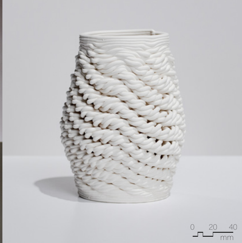
Figure 4.4.44 Unglazed PSH-515, fired to cone 04, 90mm x 90mm x 180mm, 2 layer sequence (x4), spiral patterning, non-planar pattern.
