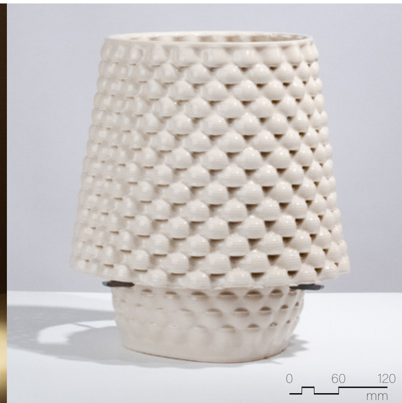
Figure 4.5.40 Clear liner glaze on PSH-516, fired to cone 6, 300mm x 300mm x 420mm, 11 layer sequence (x2).
