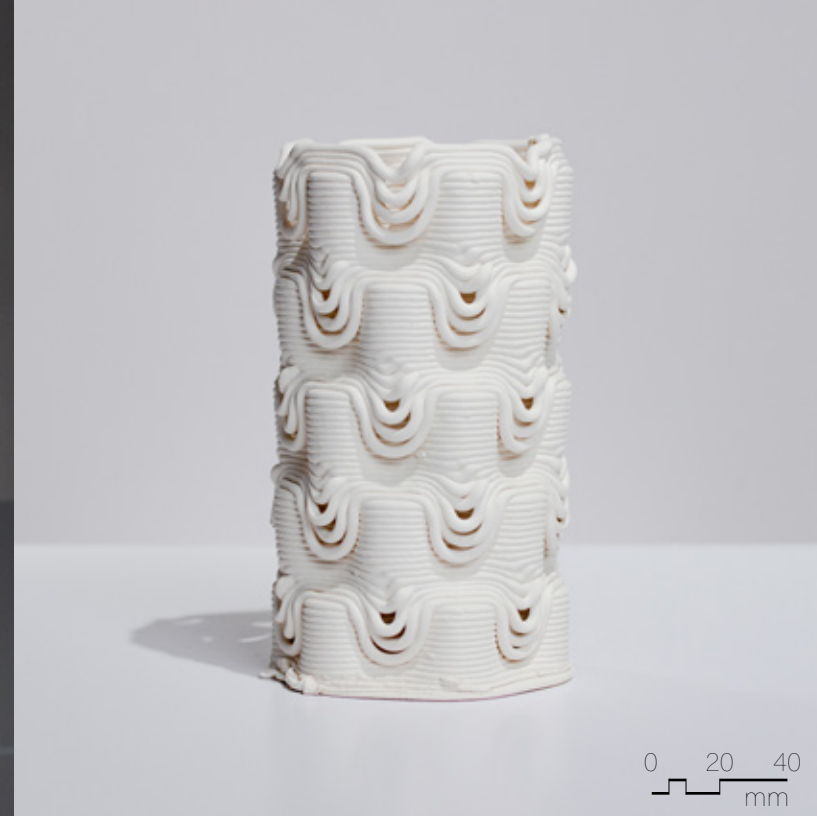
Figure 4.6.31 Unglazed PSH-515, fired to cone 04, 90mm x 90mm x 180mm, 20 layer sequence (x2).
