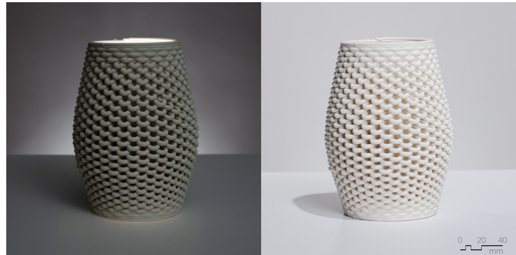
Figure 4.4.31 Unglazed PSH-515, fired to cone 04, 90mm x 90mm x 180mm, 2 layer sequence (x2).
