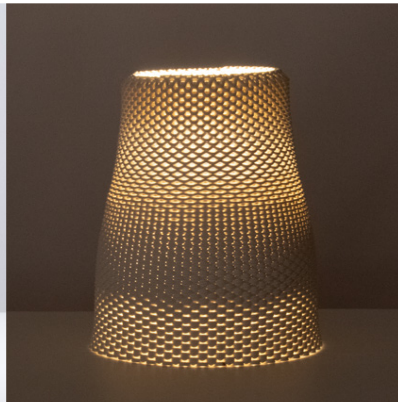
Figure 4.4.63 Unglazed PSH-516, fired to cone 04, 280mm x 280mm x 350mm, 3 layer sequence (x2).
