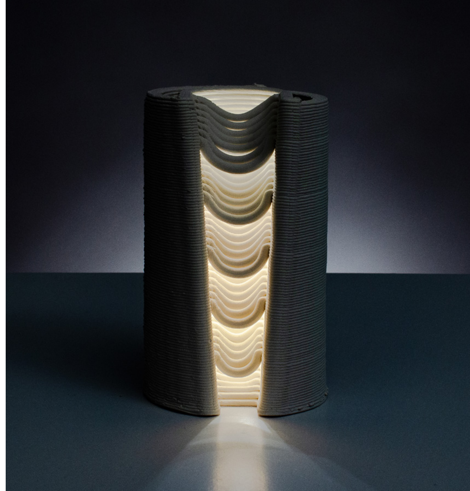
Figure 2.5.8 Stoneware light screen (70mm x 70mm x 150mm), extruded using the Potterbot XLS using a 5mm nozzle.
