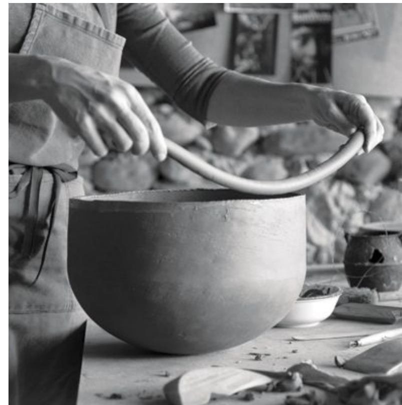
Figure 2.2.1 Traditional coil potting by Sylvie Enjalbert.
