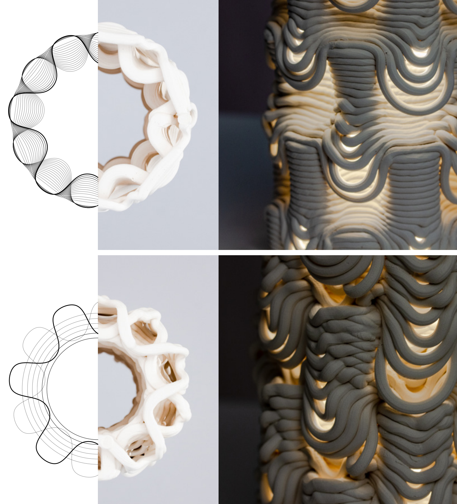
Figure 4.6.24 The scoop pattern (above) is transformed into light shelves (below) by staggering wave print layers with circular print layers.
