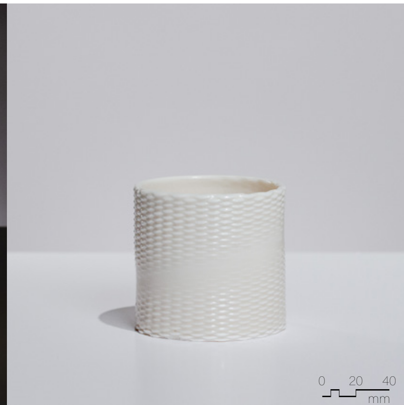
Figure 4.3.20 Clear liner glaze on Polar Ice, fired to cone 6, 90mm x 90mm x 80mm, 2 layer sequence (x2), extrusion variability.
