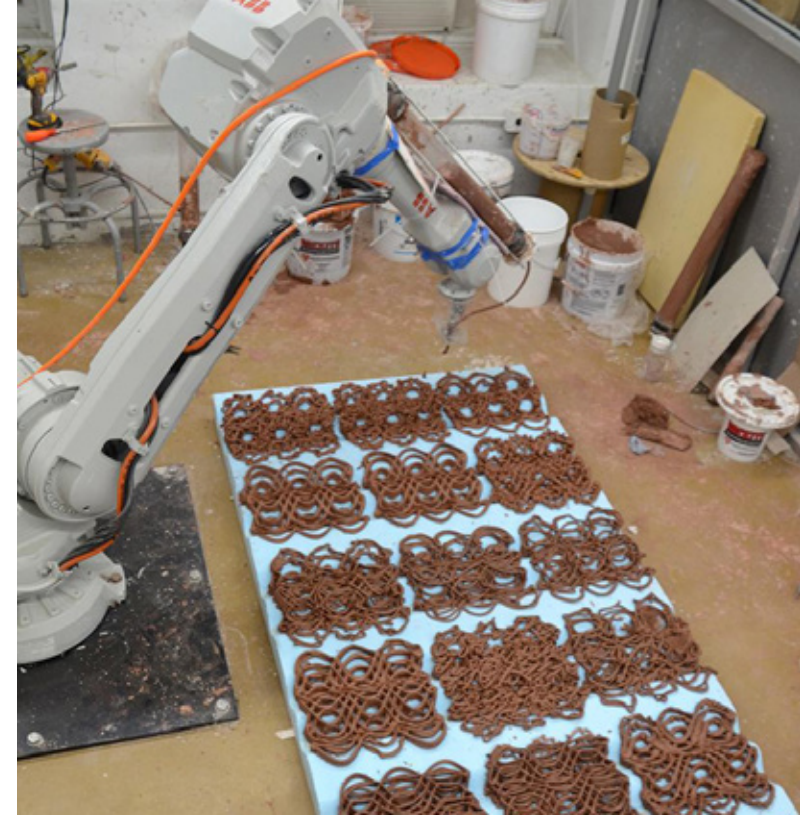
Figure 3.4.13 Non-woven clay prints in progress.
