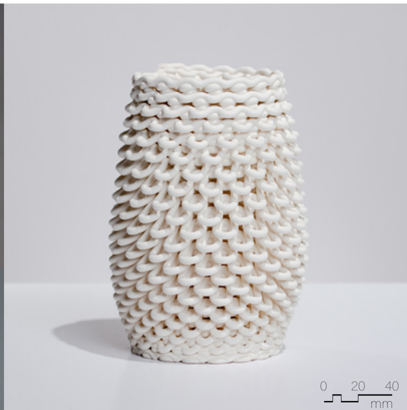
Figure 4.4.33 Unglazed PSH-515, fired to cone 04, 90mm x 90mm x 180mm, 3 layer sequence (x2).
