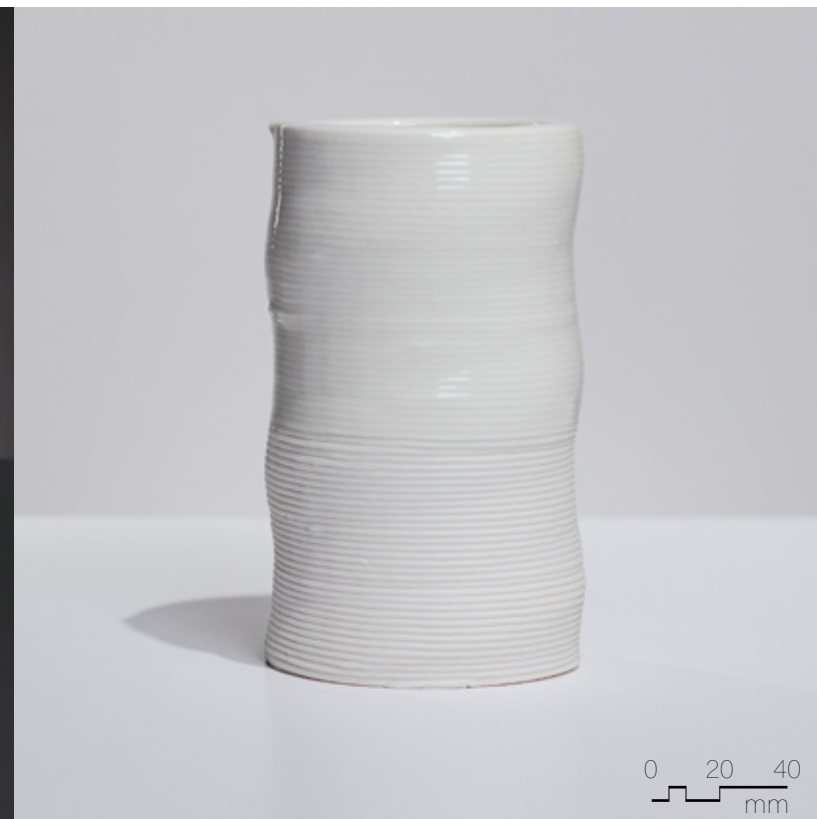
Figure 4.3.22 Clear liner glaze on Laguna Frost, fired to cone 6, 90mm x 90mm x 180mm, extrusion variability.
