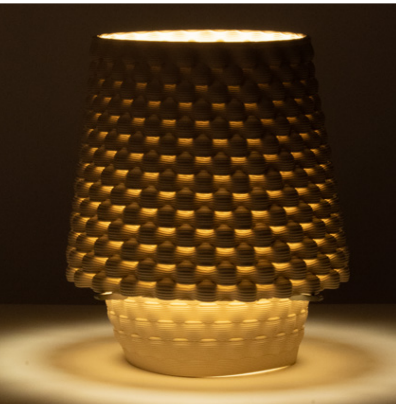
Figure 4.5.38 Unglazed PSH-516, fired to cone 6, 300mm x 300mm x 420mm, 11 layer sequence (x2).
