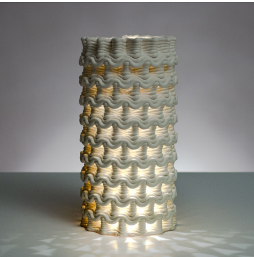
Figure 4.5.30 Unglazed PSH-515, fired to cone 04, 90mm x 90mm x 180mm, 8 layer sequence (x2).
