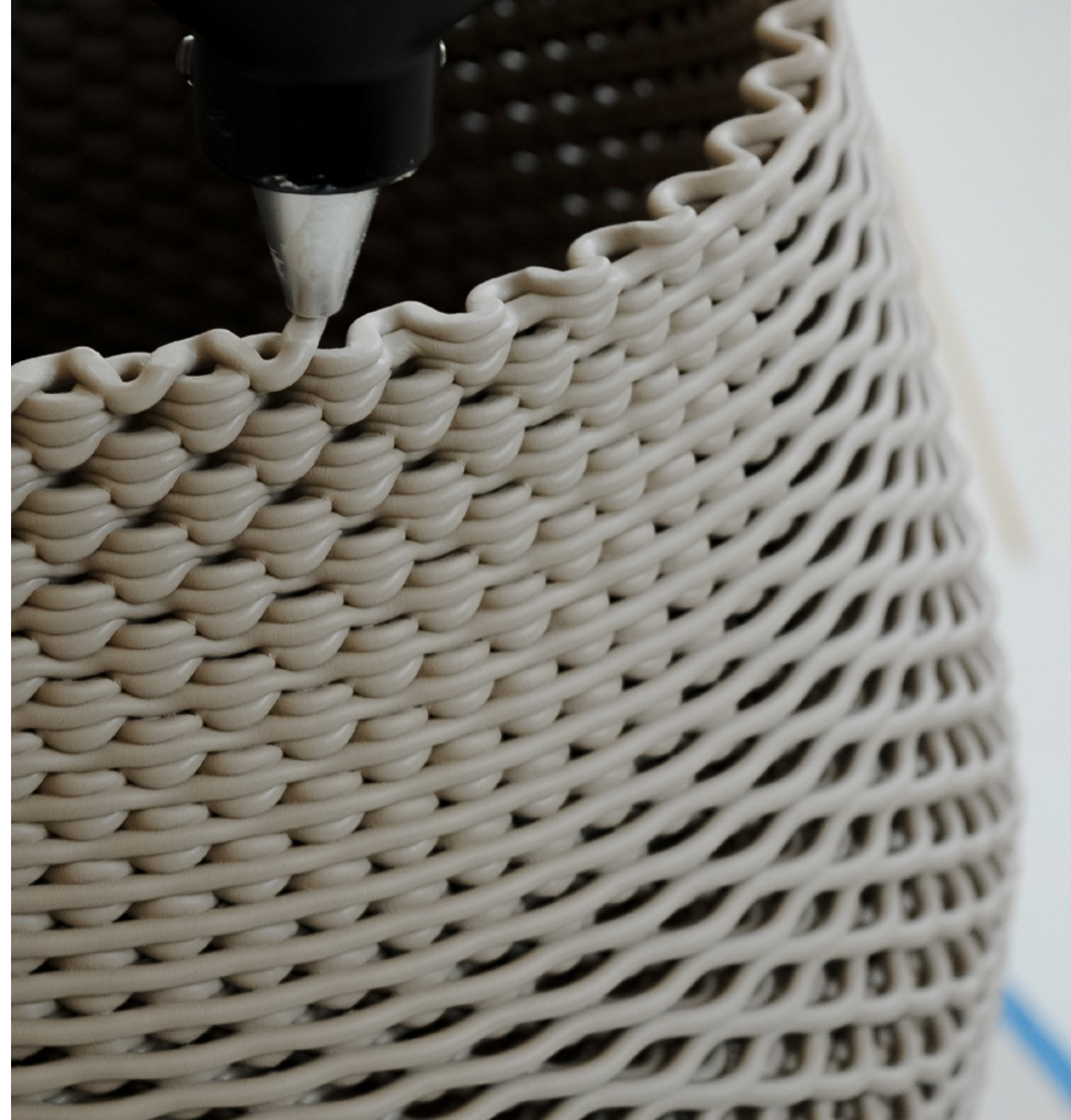
Figure 2.5.1 Wet processing a stoneware light screen (320mm x 320mm x 400mm).
