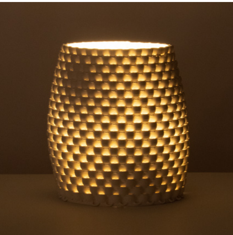
Figure 4.5.34 Unglazed PSH-516, fired to cone 04, 230mm x 230mm x 340mm, 11 layer sequence (x2).
