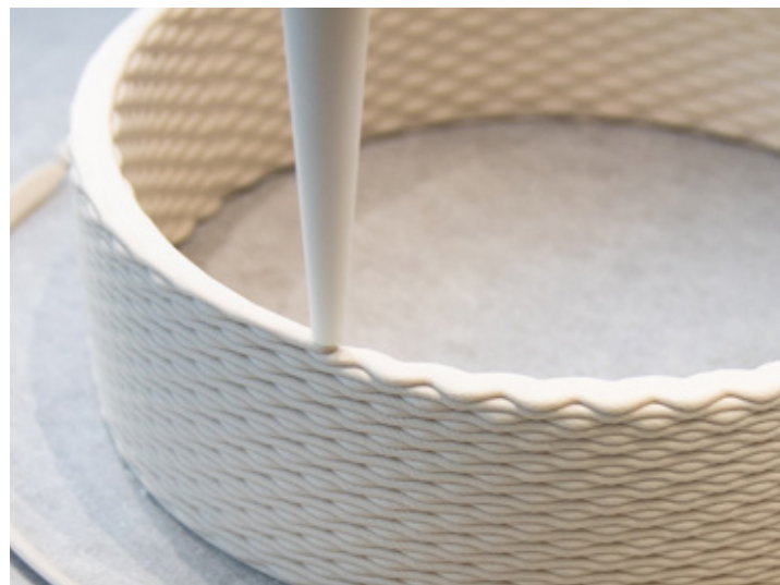
Figure 4.3.10 Variable extrusion print layers 01, 02, 03.
