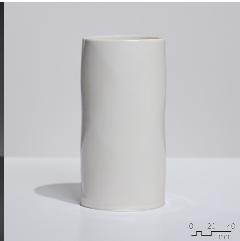
Figure 4.3.24 Clear liner glaze on Polar Ice, fired to cone 6, 90mm x 90mm x 80mm, extrusion variability.
