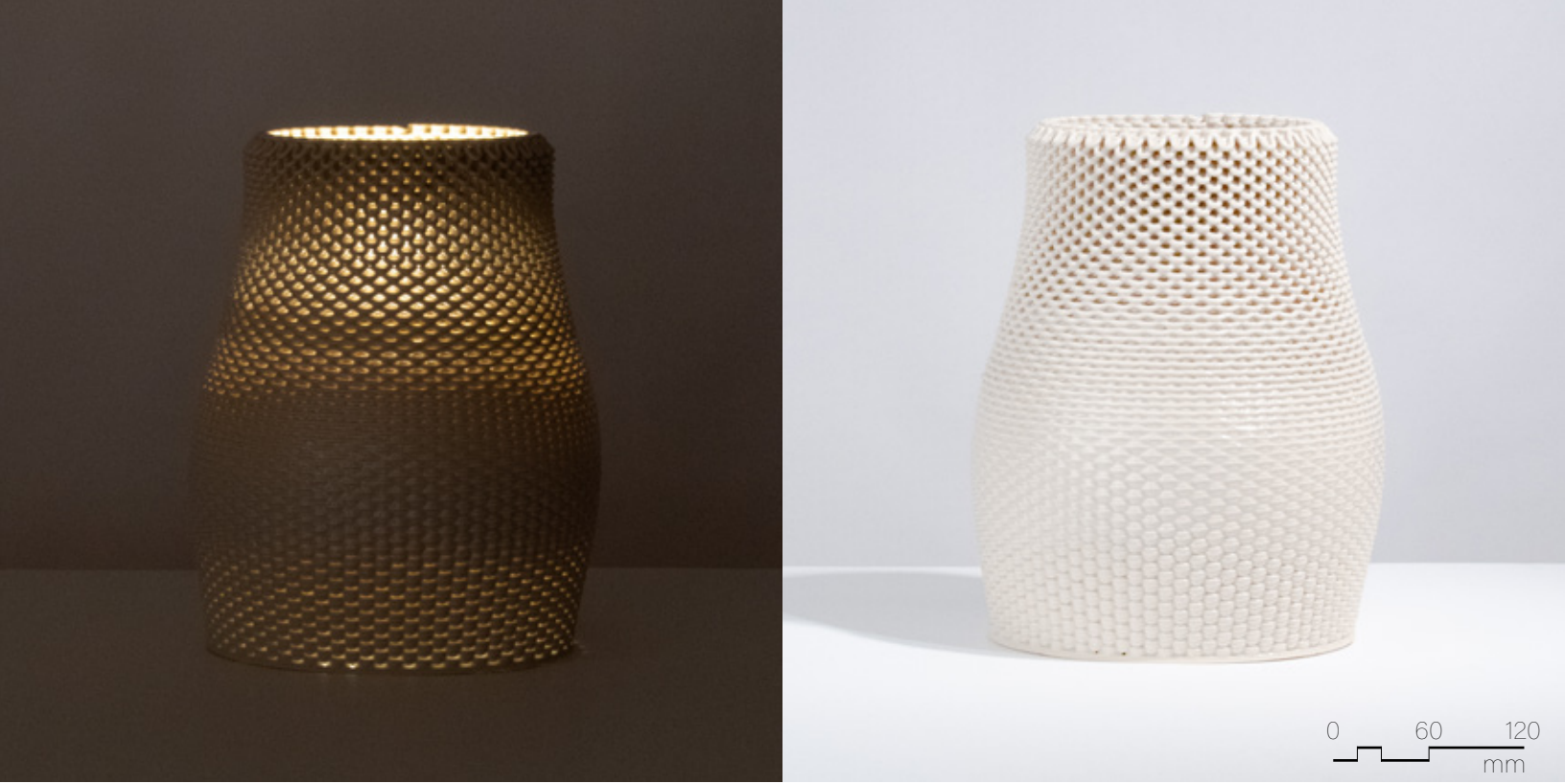
Figure 4.4.64 Clear liner glaze on PSH-516, fired to cone 6, 280mm x 280mm x 350mm, 3 layer sequence (x2).
