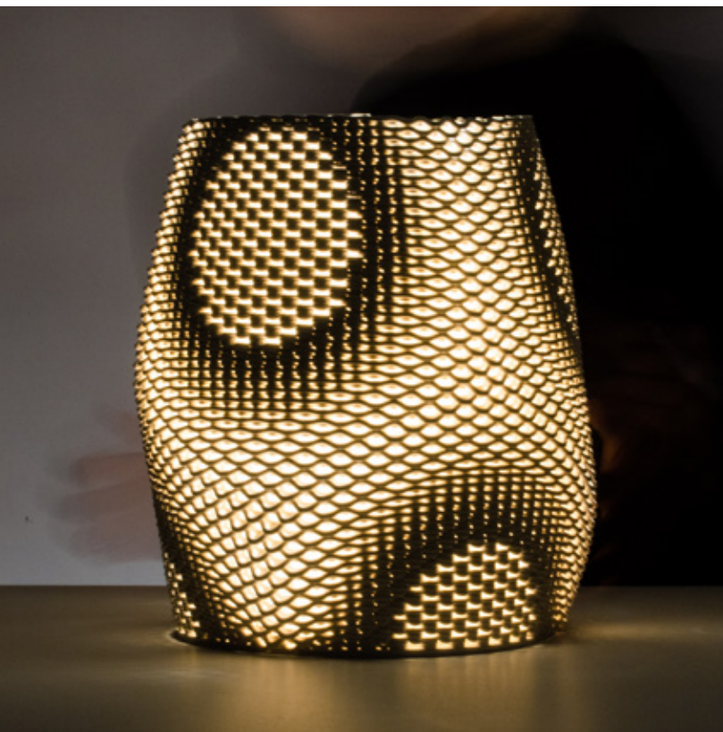
Figure 4.4.53 Unglazed PSH-516, fired to cone 04, 230mm x 230mm x 340mm, 3 layer sequence (x2).
