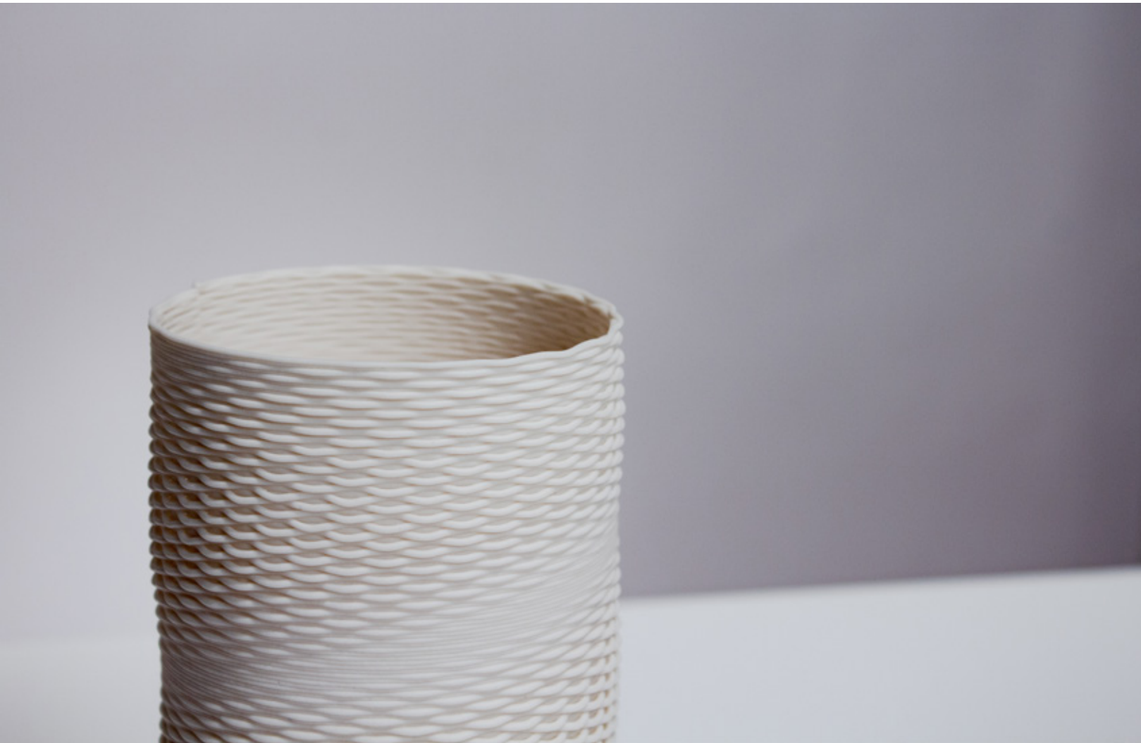
Figure 2.5.9 1mm porcelain wall detail (100mm x 100mm x 200mm), extruded using the Lutum 4.
