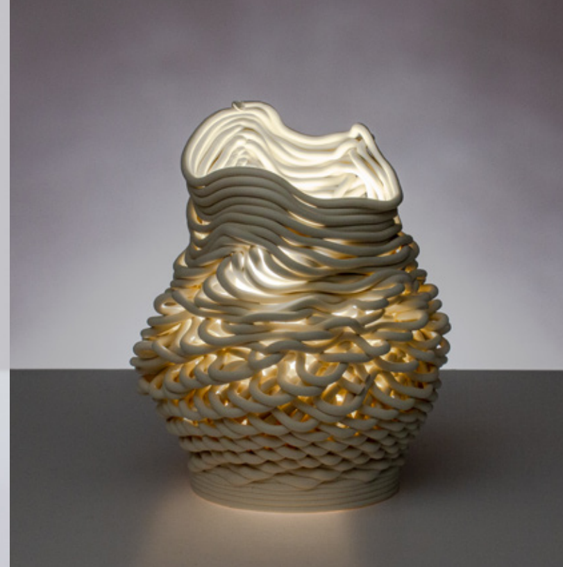
Figure 4.4.38 Unglazed PSH-515, fired to cone 04, 90mm x 90mm x 160mm, 3 layer sequence (x3), spiral pattern.
