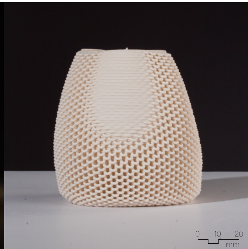
Figure 4.3.28 Unglazed Laguna Frost, fired to cone 6, 90mm x 90mm x 90mm, 2 layer sequence (x2), extrusion variability.
