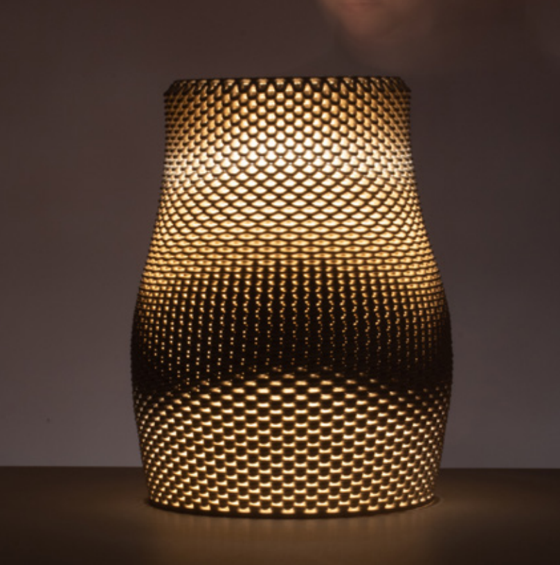
Figure 4.4.60 Unglazed PSH-516, fired to cone 04, 280mm x 280mm x 350mm, 3 layer sequence (x2).
