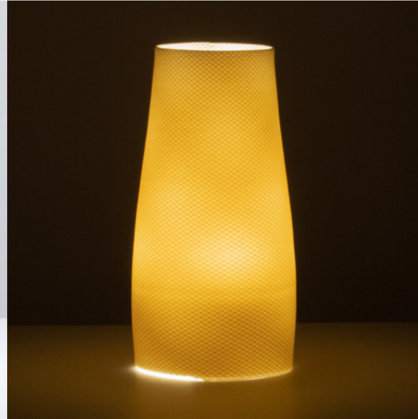
Figure 4.3.33 Unglazed Laguna Frost, fired to cone 6, 160mm x 160mm x 300mm, 2 layer sequence (x2), extrusion variability.
