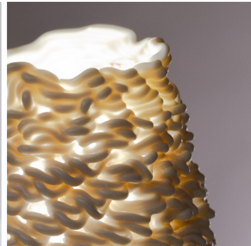
Figure 2.5.3 Tool path variability across a porcelain clay body (100mm x 100mm x 200mm).
