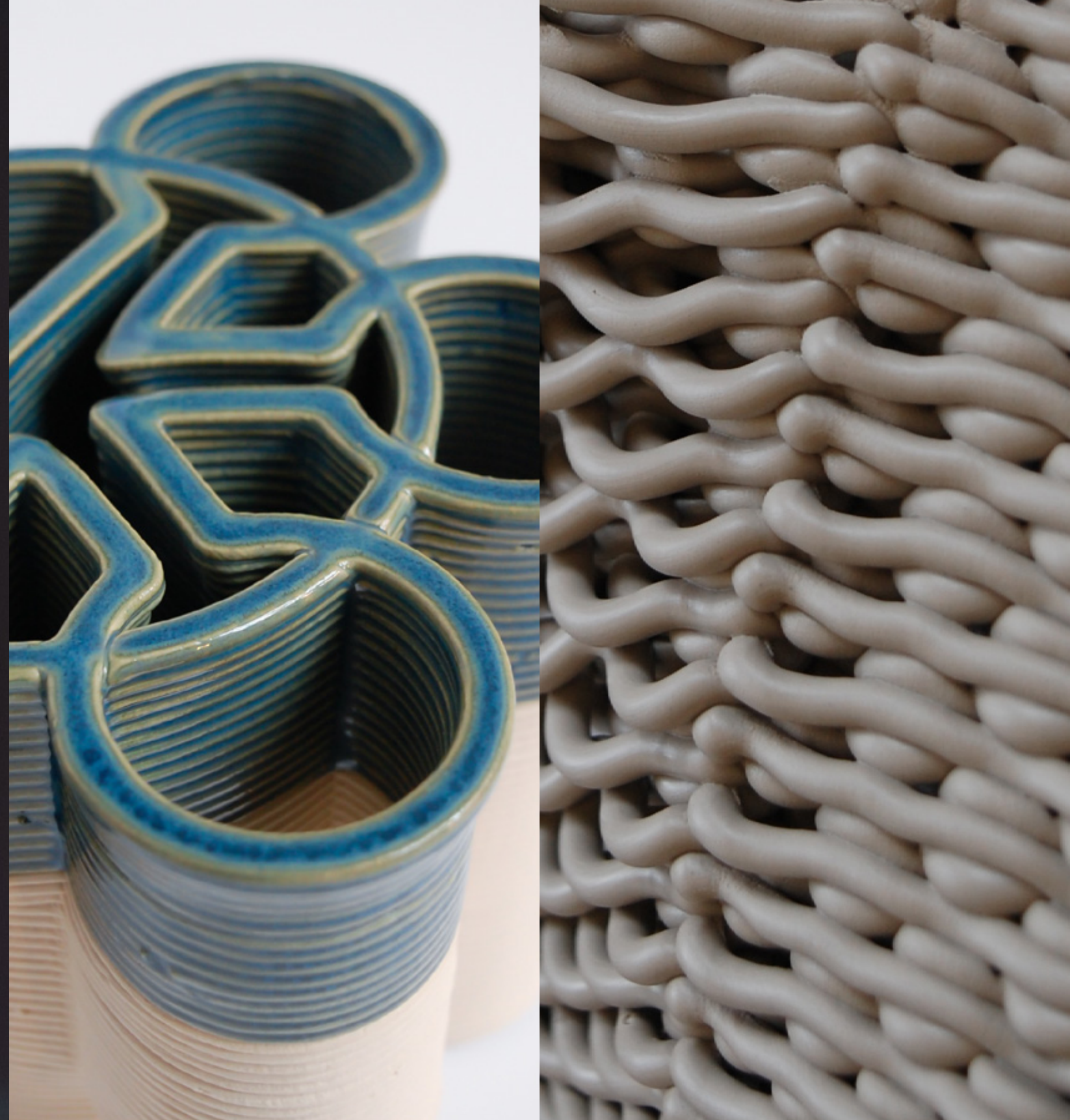
Figure 3.3.5 Examples of geometry intersection (left) and seam generation (right).
