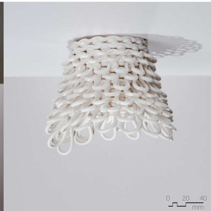
Figure 4.4.51 Unglazed PSH-515, fired to cone 04, 90mm x 90mm x 150mm, 3 layer sequence (x2), hanging loops.
