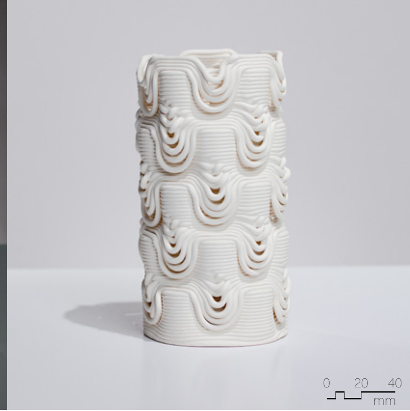
Figure 4.6.27 Unglazed PSH-515, fired to cone 04, 90mm x 90mm x 180mm, 22 layer sequence (x2).
