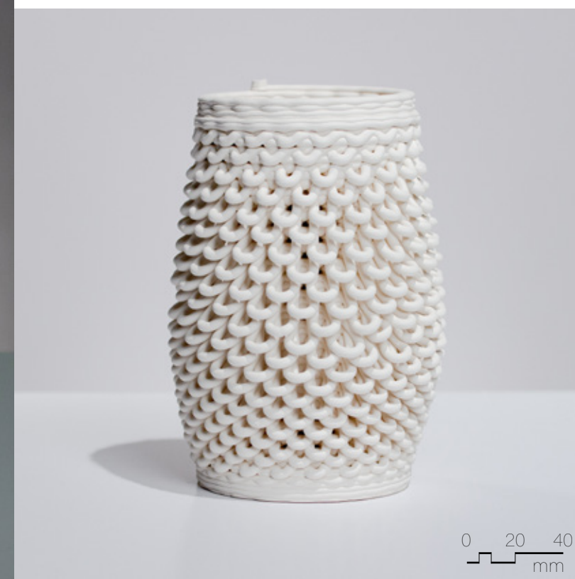
Figure 4.4.34 Unglazed PSH-515, fired to cone 04, 90mm x 90mm x 180mm, 3 layer sequence (x2).
