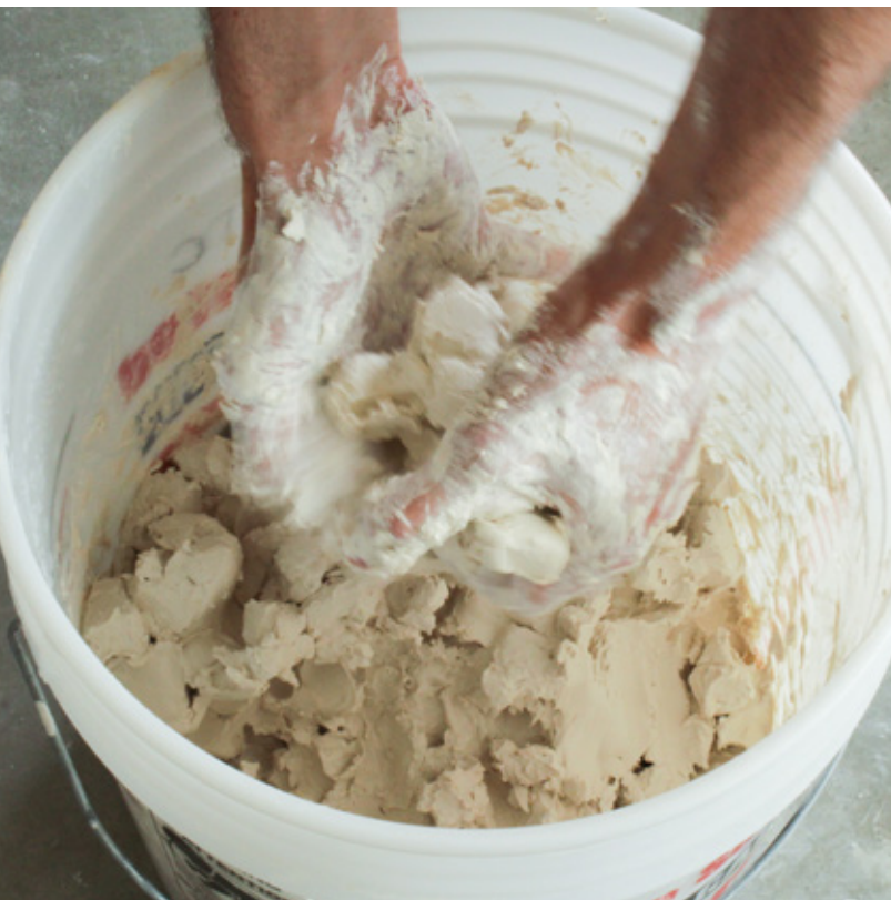
Figure 2.1.2 Examples of clay's working properties- plasticity and the ability of the material to retain its given shape.
