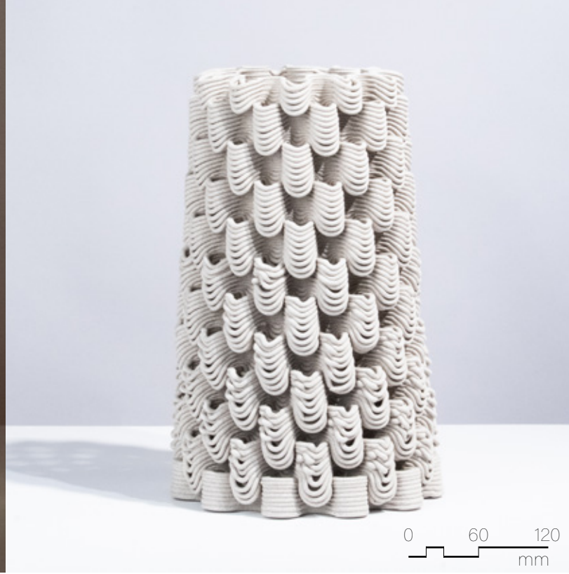
Figure 4.6.35 Unglazed PSH Dark Granite, fired to cone 04, 200mm x 200mm x 340mm, 20 layer sequence (x2).
