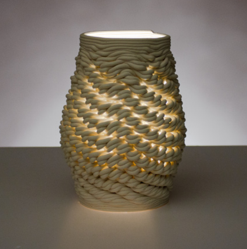
Figure 4.4.44 Unglazed PSH-515, fired to cone 04, 90mm x 90mm x 180mm, 2 layer sequence (x4), spiral patterning, non-planar pattern.
