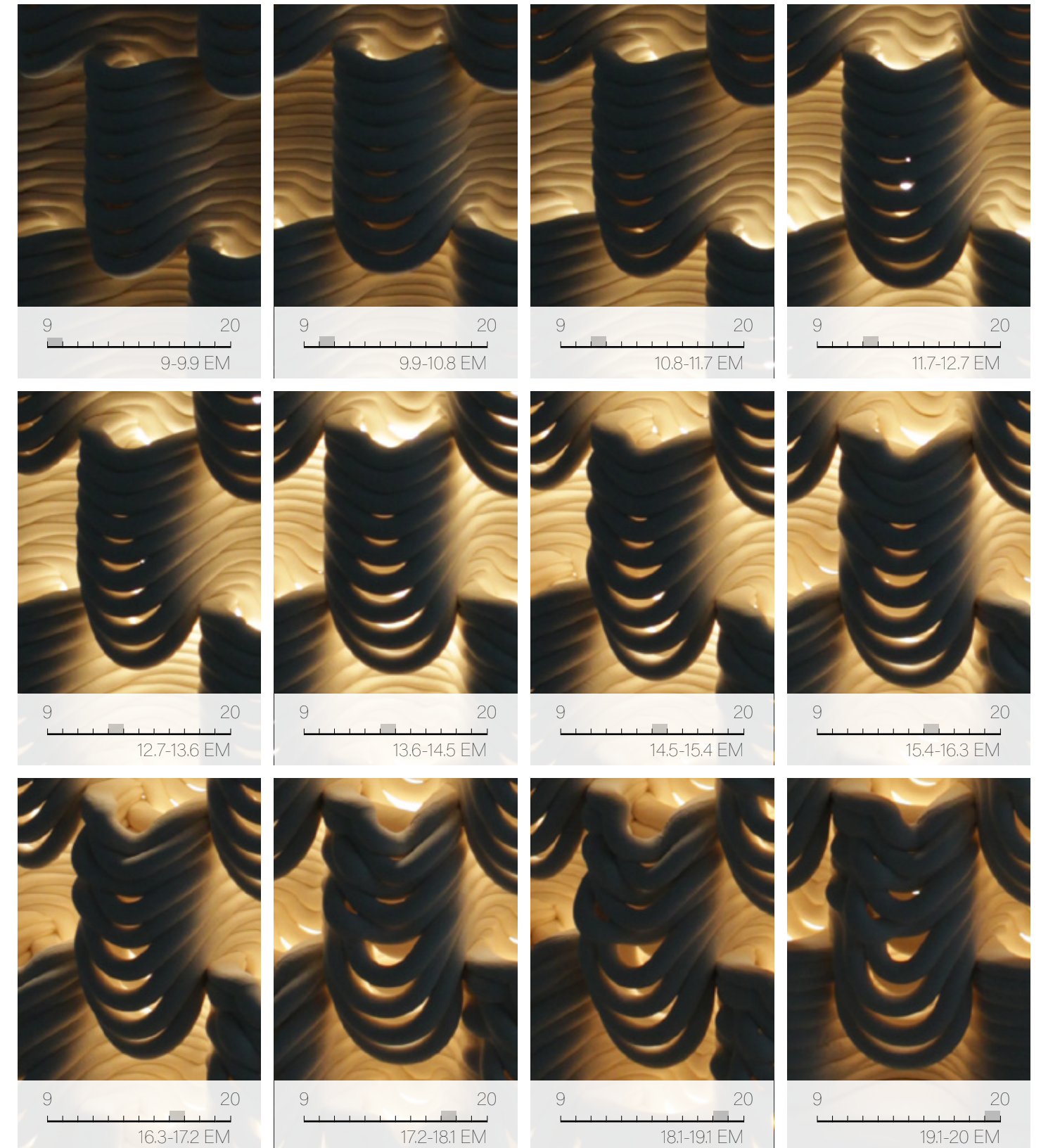
Figure 4.6.22 Extrusion Multiplier (EM) ranging from 9 to 20 in the final 'XL' prototype.
