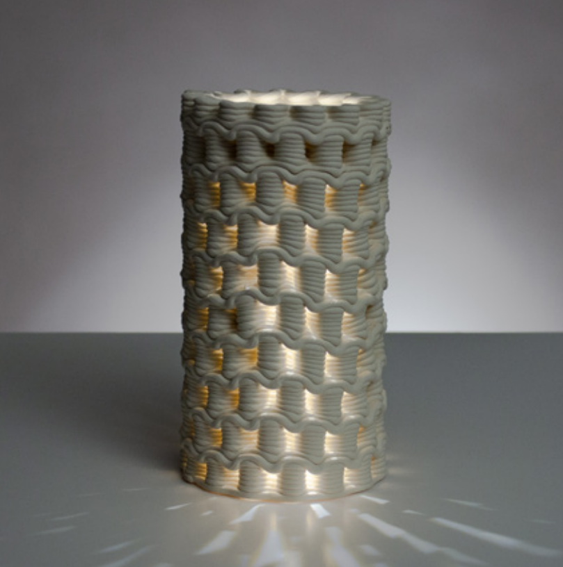
Figure 4.5.33 Unglazed PSH-515, fired to cone 04, 90mm x 90mm x 180mm, 8 layer sequence (x2), non-planar pattern.
