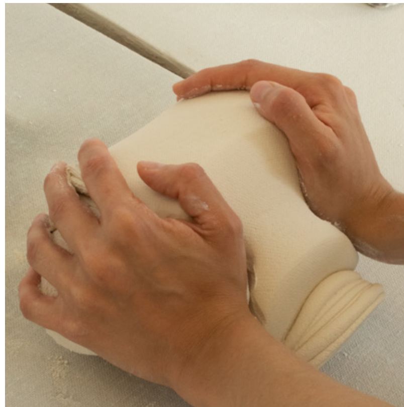
Figure 2.1.2 Examples of clay's working properties- plasticity and the ability of the material to retain its given shape.
