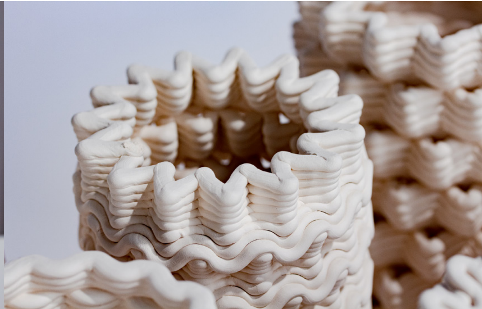
Figure 2.5.10 5mm stoneware wall detail (100mm x 100mm x 200mm), extruded using the Potterbot XLS-1.
