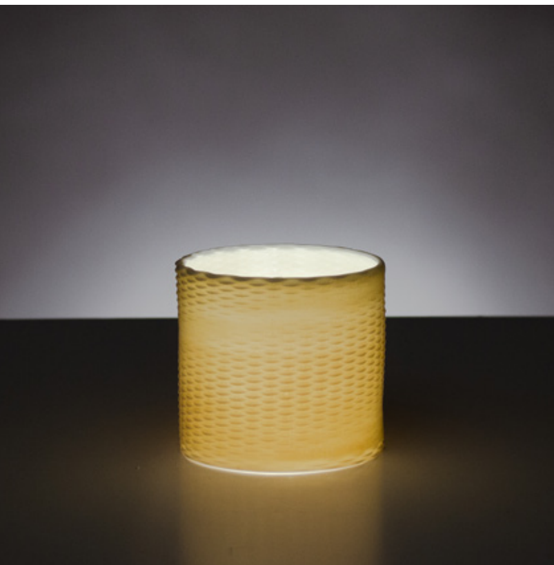
Figure 4.3.20 Clear liner glaze on Polar Ice, fired to cone 6, 90mm x 90mm x 80mm, 2 layer sequence (x2), extrusion variability.
