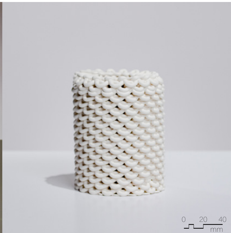
Figure 4.4.37 Unglazed PSH-515, fired to cone 04, 90mm x 90mm x 150mm, 3 layer sequence (x2), inverted loop pattern.
