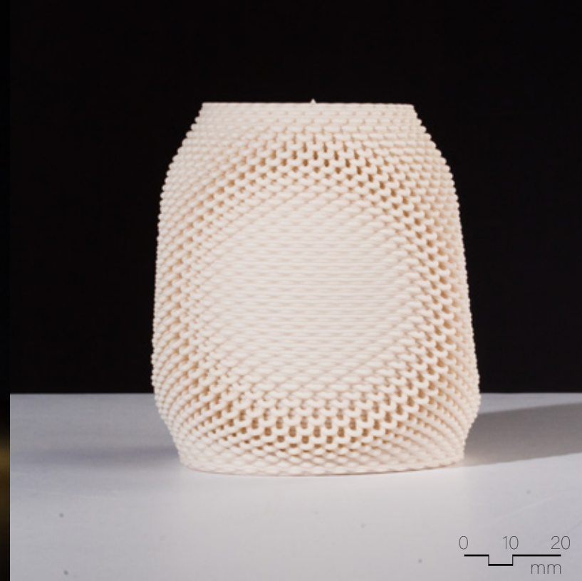
Figure 4.3.27 Unglazed Laguna Frost, fired to cone 6, 90mm x 90mm x 90mm, 2 layer sequence (x2), extrusion variability.
