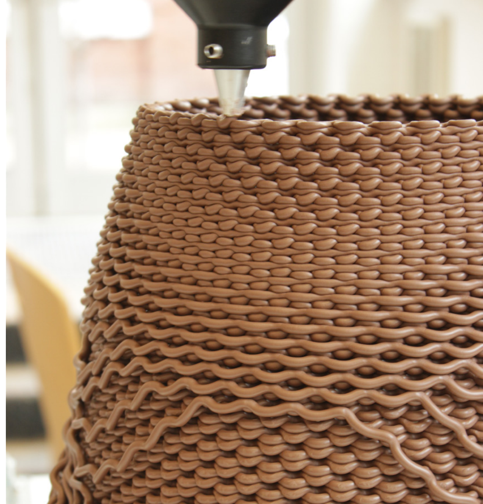
Figure 1.2.1 'M' prototype in terracotta, delaminating during printing.
