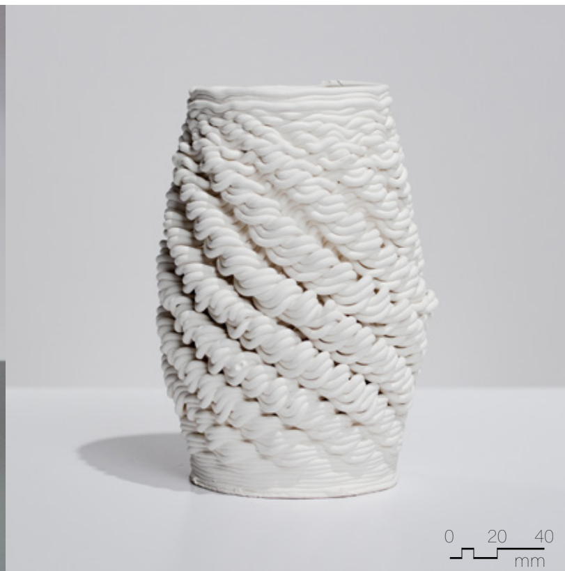
Figure 4.4.45 Unglazed PSH-515, fired to cone 04, 90mm x 90mm x 180mm, 3 layer sequence (x4), spiral pattern.
