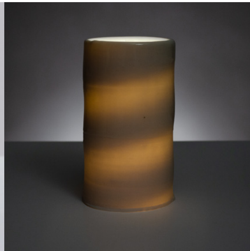
Figure 4.3.22 Clear liner glaze on Laguna Frost, fired to cone 6, 90mm x 90mm x 180mm, extrusion variability.
