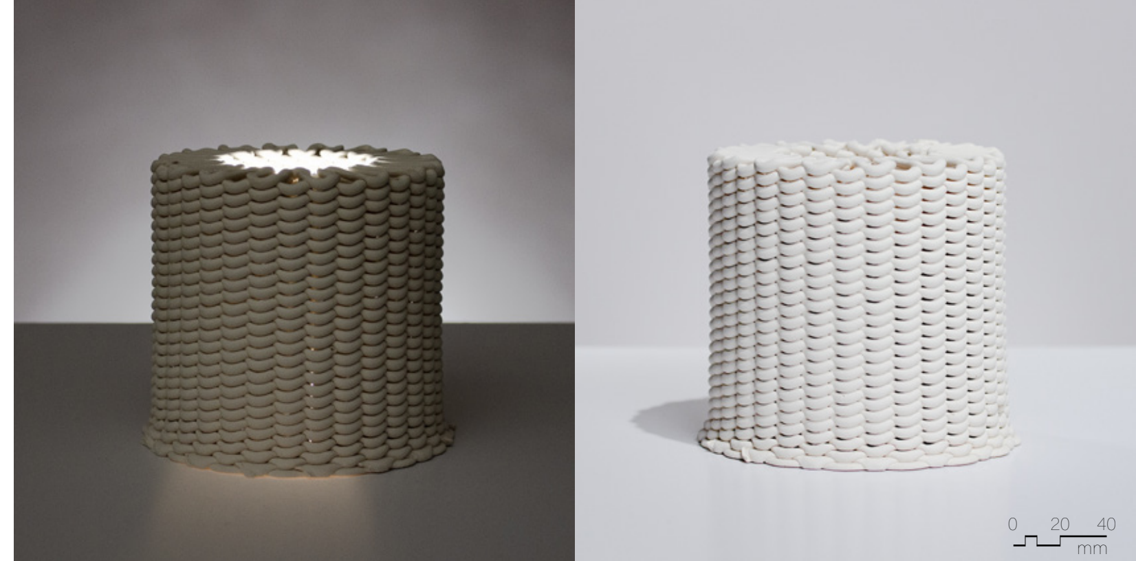
Figure 4.4.30 Unglazed PSH-515, fired to cone 04, 120mm x 120mm x 150mm, 2 layer sequence (x2).
