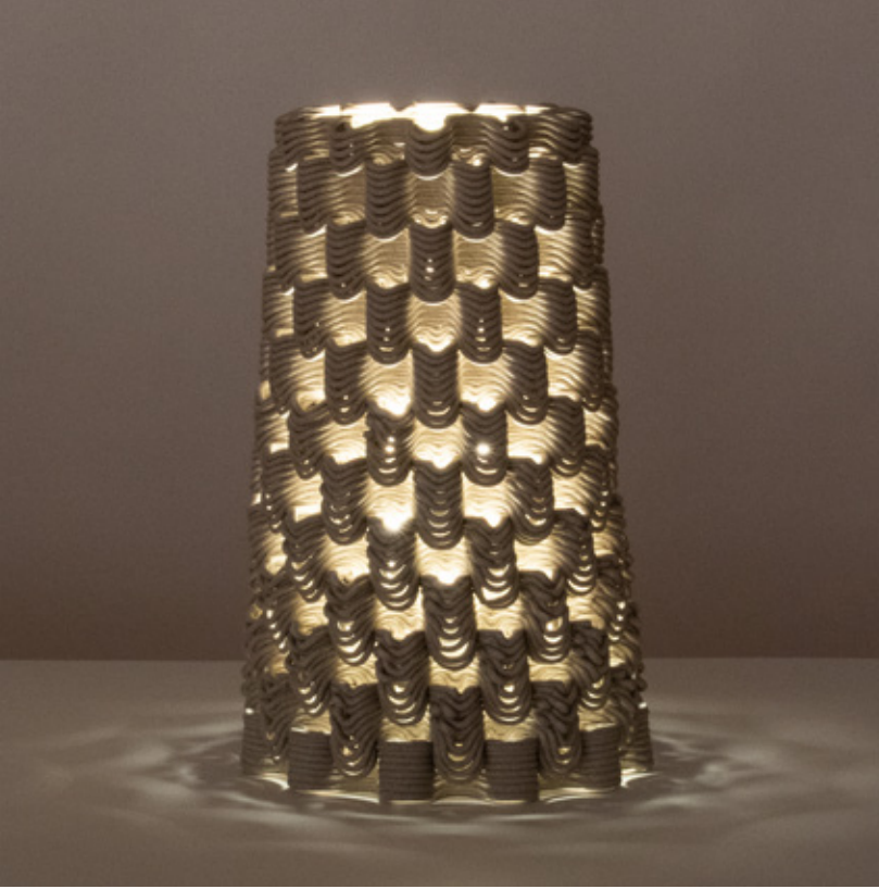
Figure 4.6.35 Unglazed PSH Dark Granite, fired to cone 04, 200mm x 200mm x 340mm, 20 layer sequence (x2).
