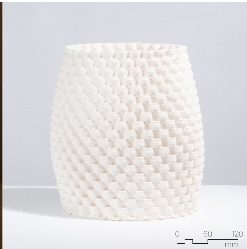
Figure 4.5.34 Unglazed PSH-516, fired to cone 04, 230mm x 230mm x 340mm, 11 layer sequence (x2).
