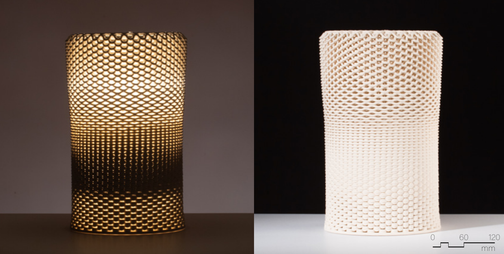
Figure 4.4.56 Unglazed PSH-516, fired to cone 04, 260mm x 260mm x 400mm, 3 layer sequence (x2).
