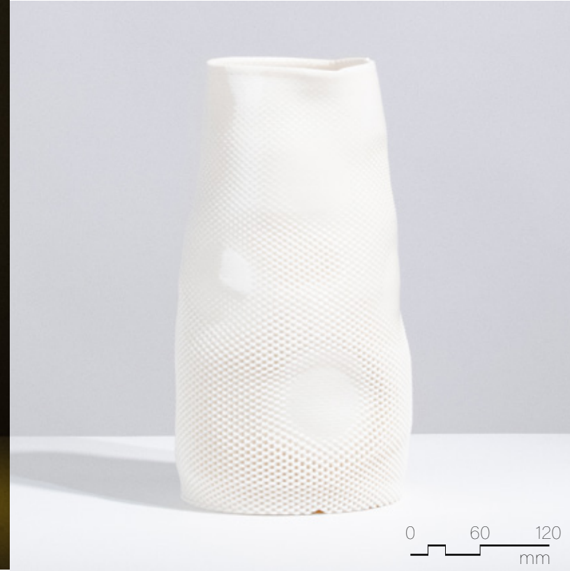
Figure 4.3.31 Clear liner glaze on Polar Ice, fired to cone 6, 160mm x 160mm x 300mm, 2 layer sequence (x2), extrusion variability.
