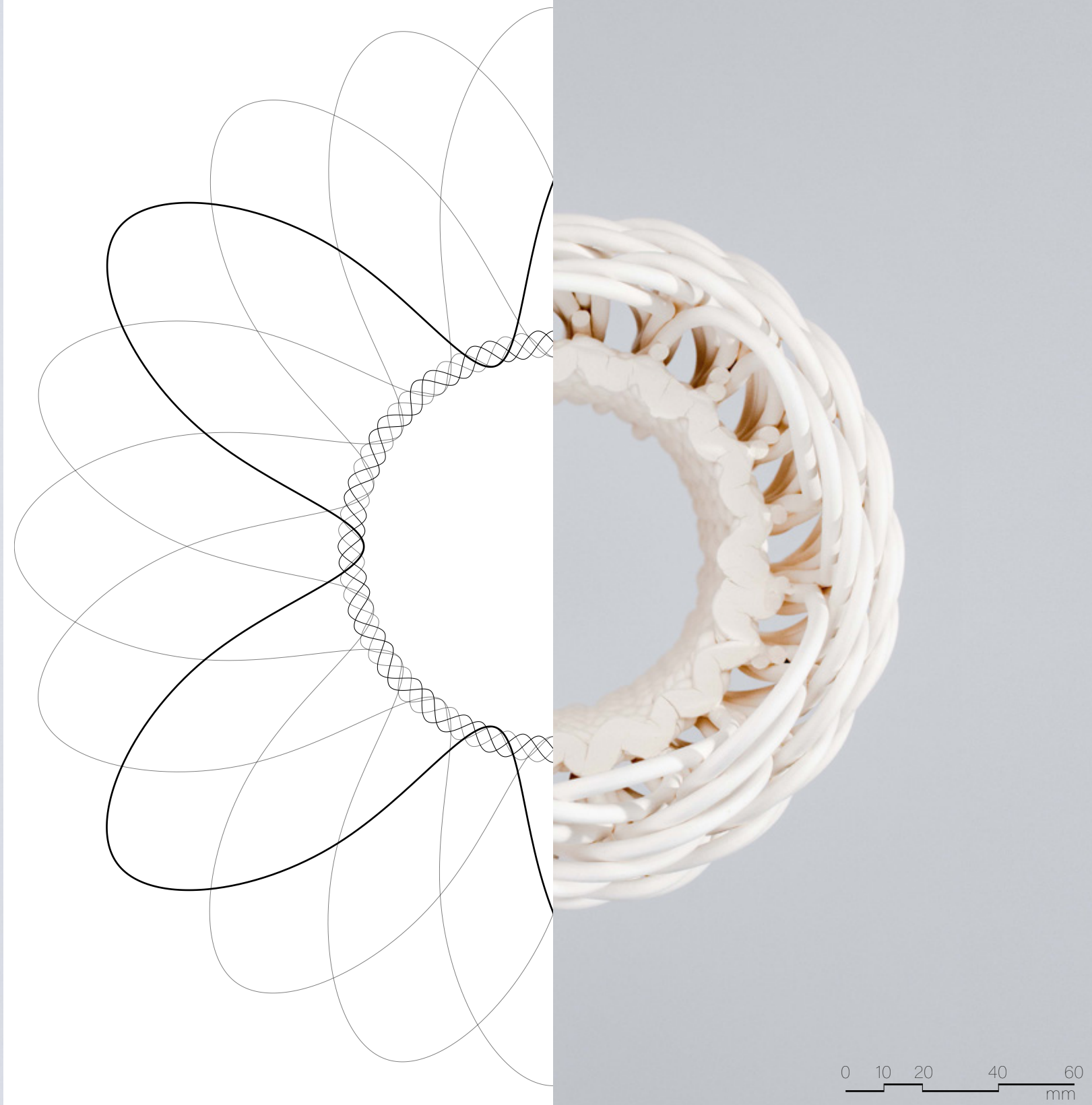
Figure 4.4.25 Oversized/Overhanging loop pattern tool path plan (left) and physical print plan (right).
