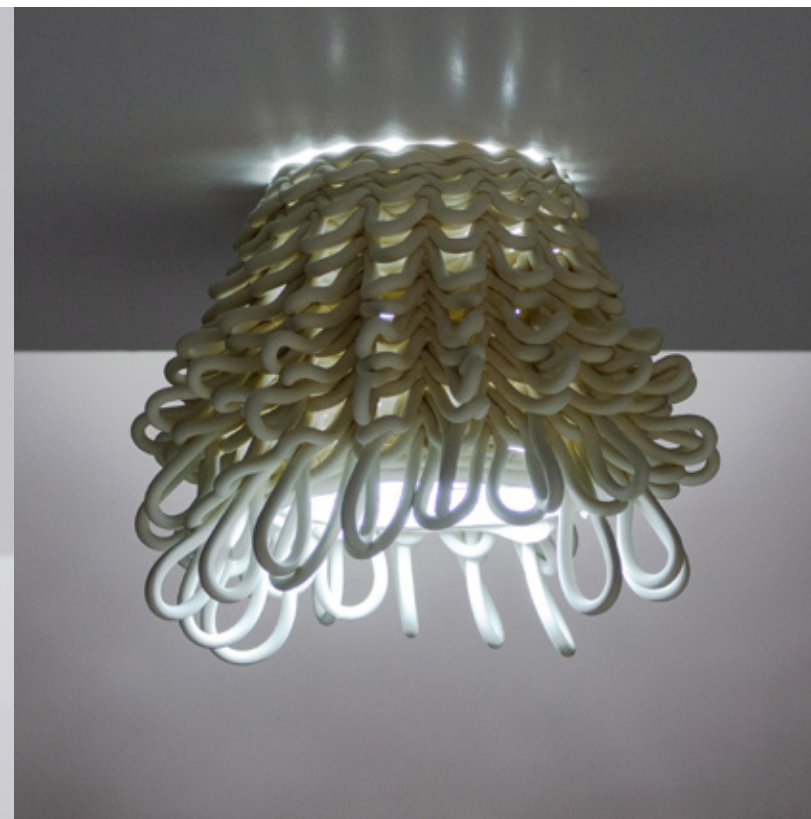
Figure 4.4.47 Unglazed PSH-515, fired to cone 04, 90mm x 90mm x 150mm, 3 layer sequence (x2), hanging loops.
