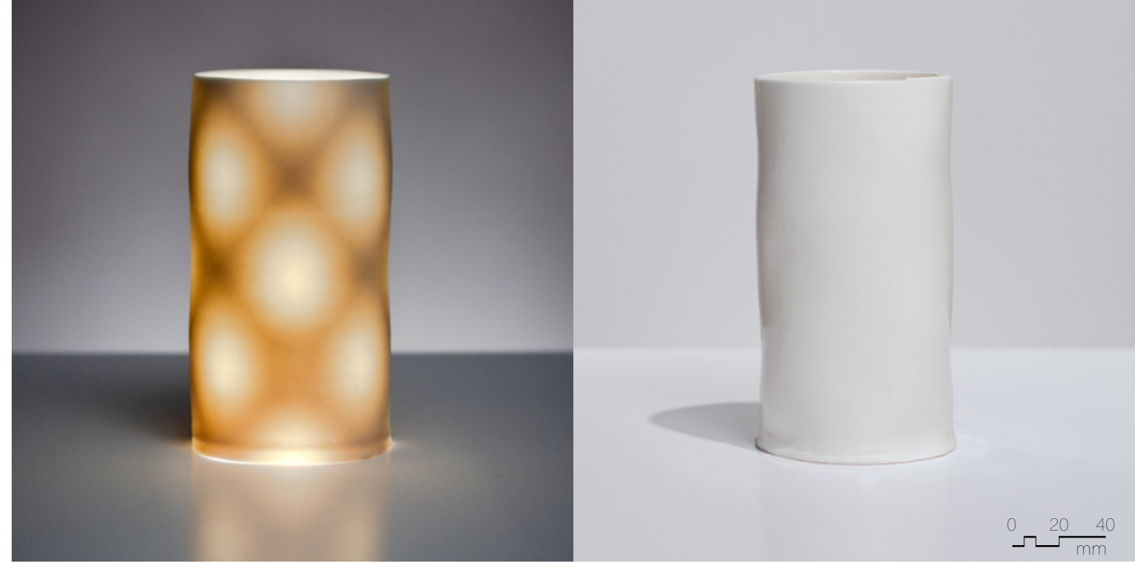
Figure 4.3.17 Clear liner glaze on Laguna Frost, fired to cone 6, 90mm x 90mm x 180mm, extrusion variability.
