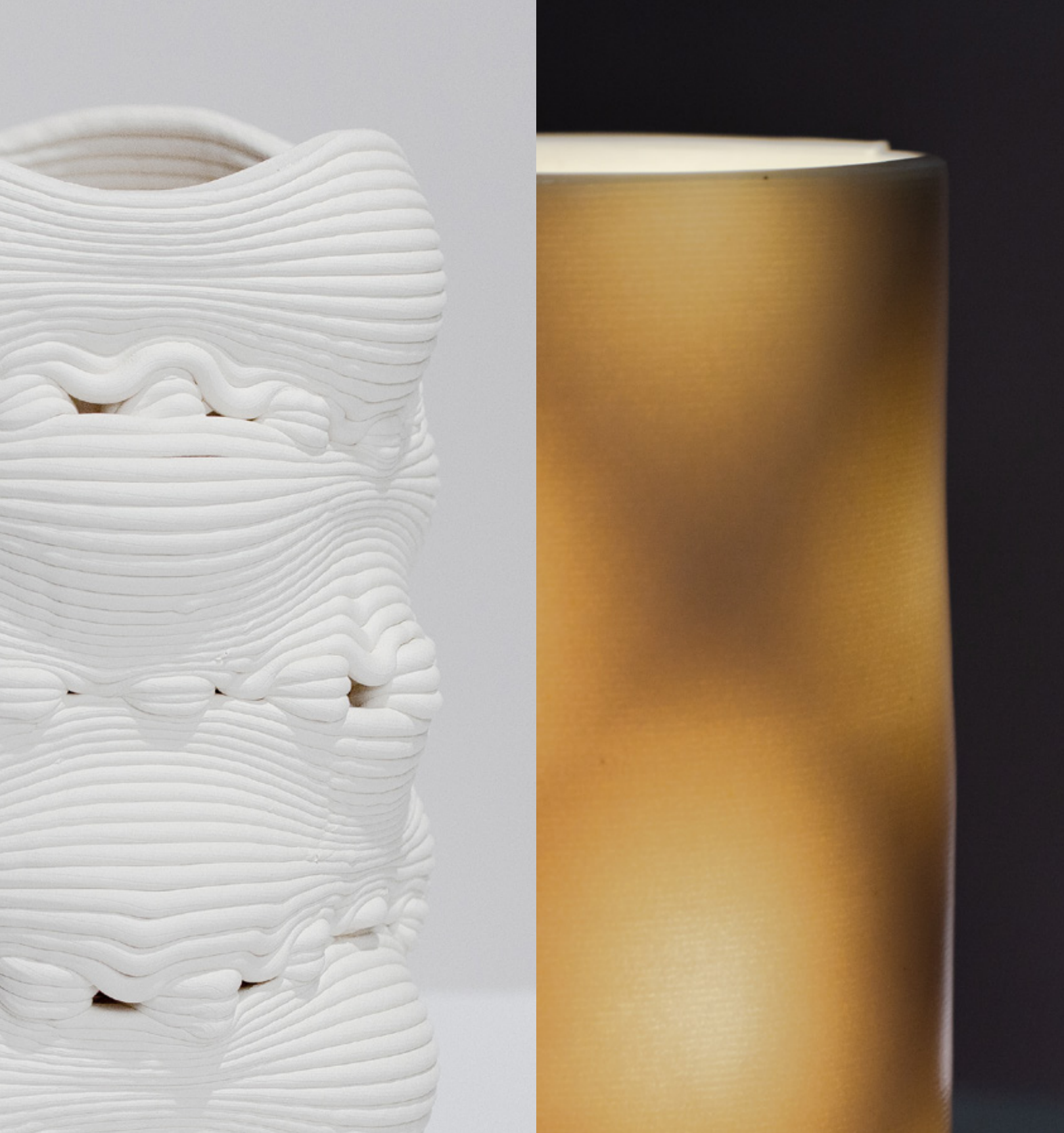
Figure 3.3.4 Examples of non-planar printing (left) and extrusion variability (right).
