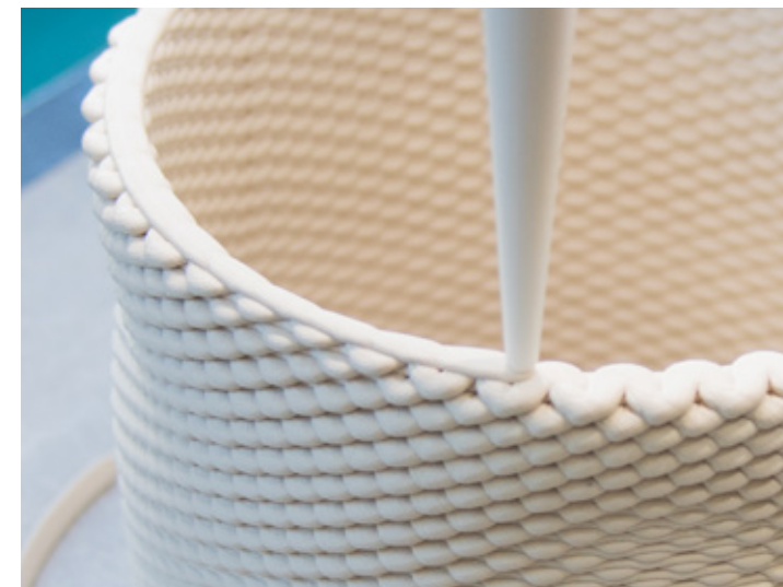
Figure 4.3.11 Variable extrusion print layers 04, 05, 06.
