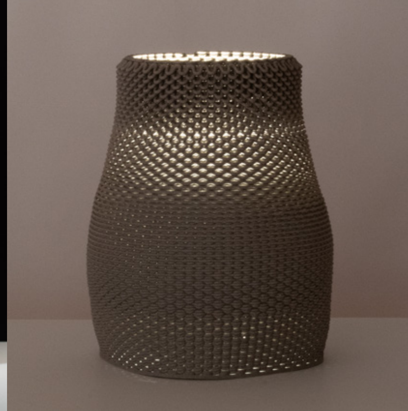
Figure 4.4.62 Unglazed PSH Dark Granite, fired to cone 6, 280mm x 280mm x 350mm, 3 layer sequence (x2).
