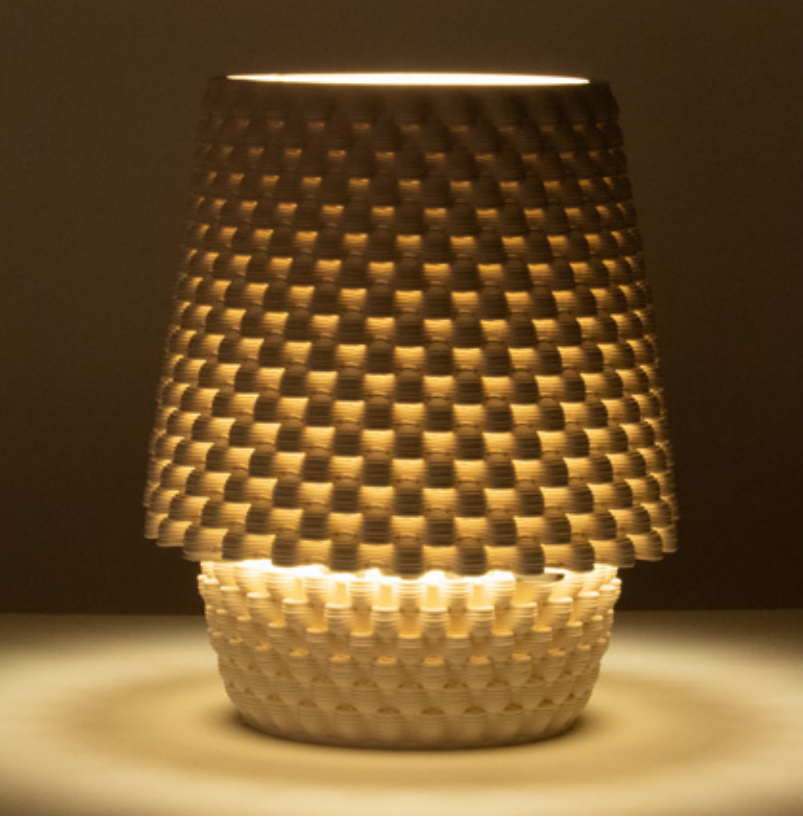
Figure 4.5.37 Unglazed PSH-516, fired to cone 04, 300mm x 300mm x 420mm, 11 layer sequence (x2).
