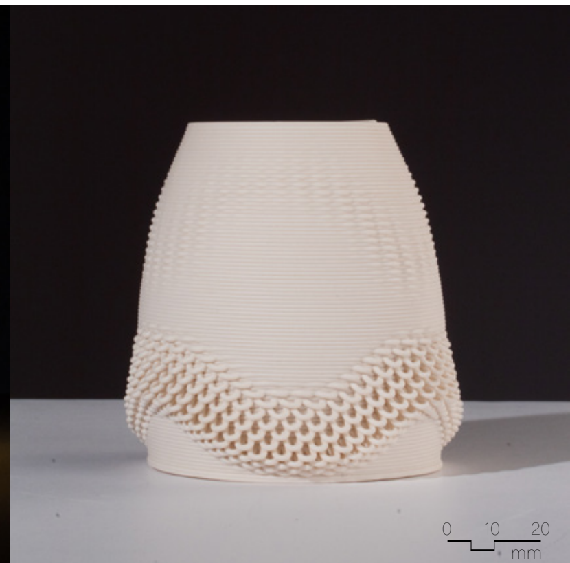
Figure 4.3.26 Unglazed Laguna Frost, fired to cone 6, 90mm x 90mm x 90mm, 2 layer sequence (x2), extrusion variability.
