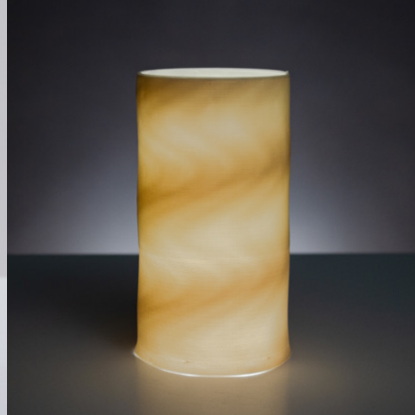
Figure 4.3.21 Clear liner glaze on Laguna Frost, fired to cone 6, 90mm x 90mm x 180mm, extrusion variability.
