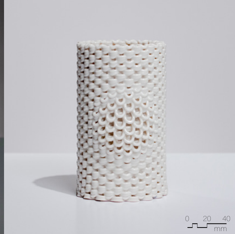
Figure 4.4.40 Clear liner glaze on Polar Ice, fired to cone 6, 90mm x 90mm x 180mm, 2 layer sequence (x2), inverted loop pattern.
