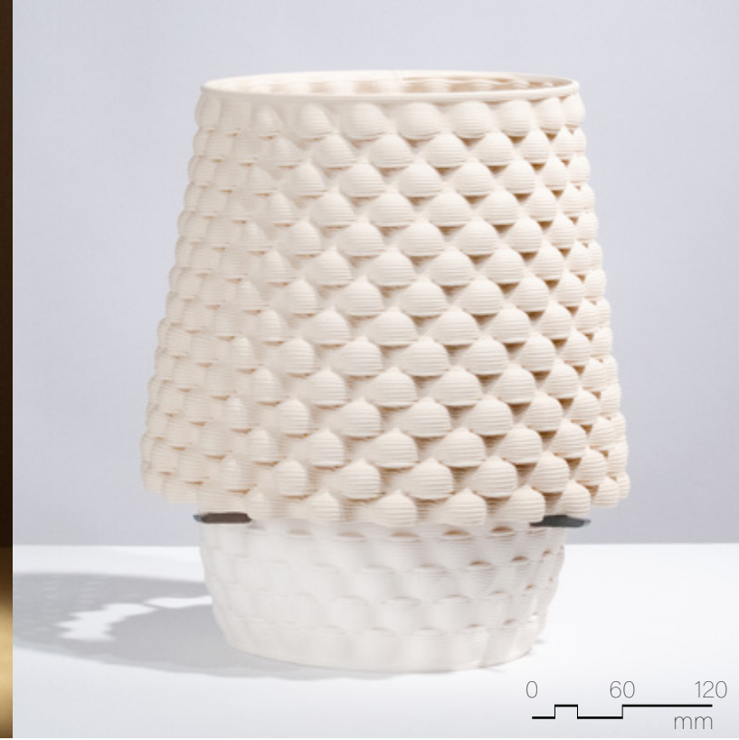
Figure 4.5.39 Unglazed PSH-516, fired to cone 6, 300mm x 300mm x 420mm, 11 layer sequence (x2).
