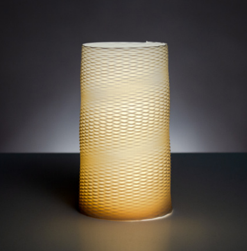
Figure 4.3.19 Clear liner glaze on Laguna Frost, fired to cone 6, 90mm x 90mm x 180mm, 2 layer sequence (x2), extrusion variability.
