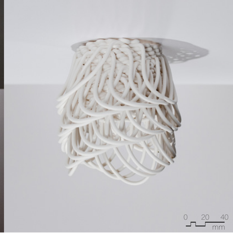
Figure 4.4.48 Unglazed PSH-515, fired to cone 04, 90mm x 90mm x 150mm, 3 layer sequence (x3), hanging loops, spiral pattern.
