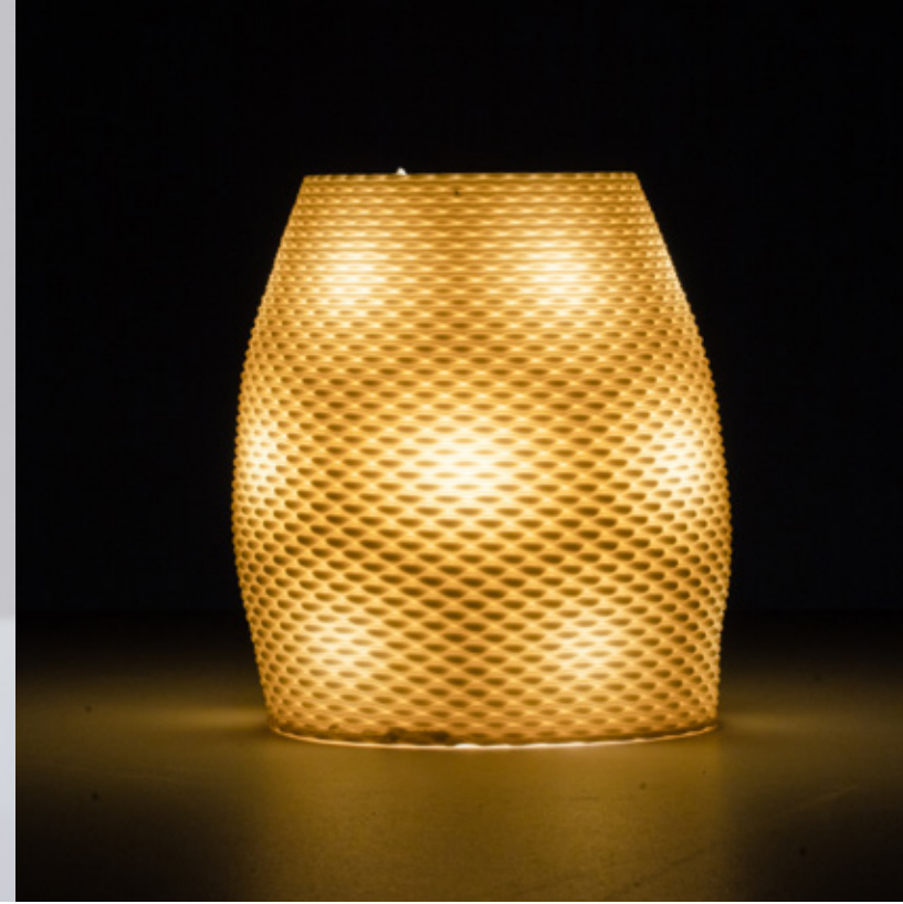
Figure 4.3.25 Unglazed Laguna Frost, fired to cone 6, 90mm x 90mm x 90mm, 2 layer sequence (x2), extrusion variability.
