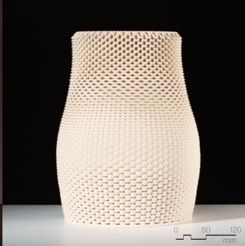
Figure 4.4.60 Unglazed PSH-516, fired to cone 04, 280mm x 280mm x 350mm, 3 layer sequence (x2).
