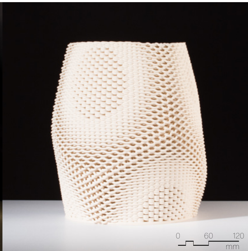
Figure 4.4.53 Unglazed PSH-516, fired to cone 04, 230mm x 230mm x 340mm, 3 layer sequence (x2).
