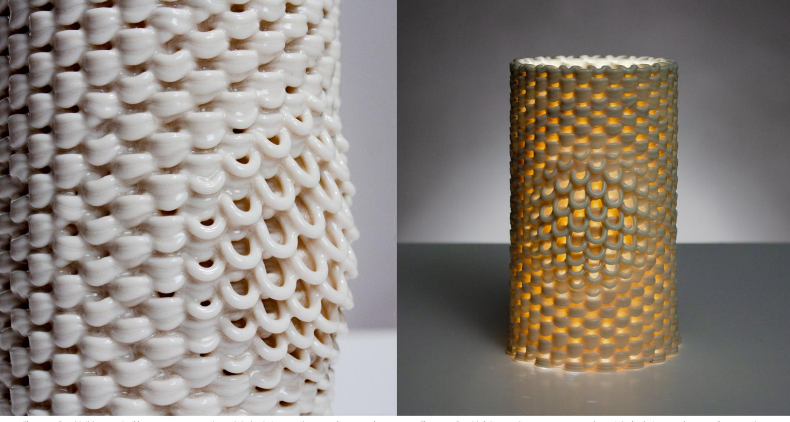
Figure 2.6.7 Porcelain light screen detail (100mm x 100mm x 200mm), extruded using the Lutum 4 using a 3mm diameter nozzle.
