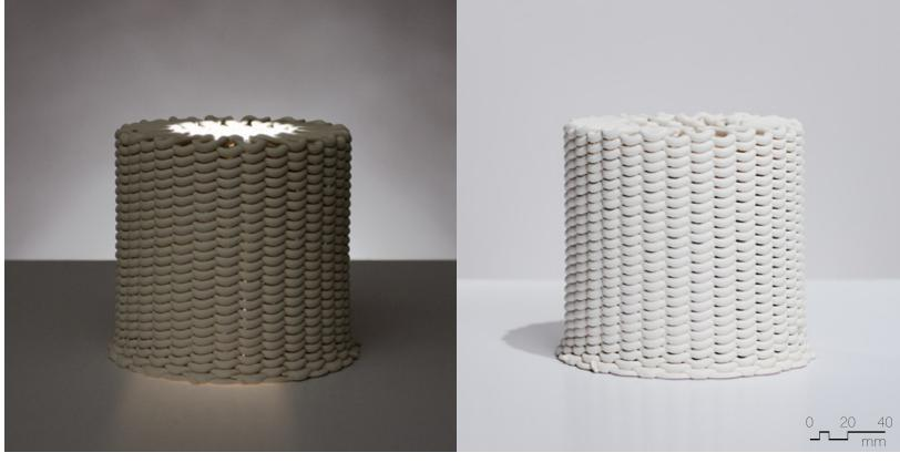
Figure 4.4.30 Unglazed PSH-515, fired to cone 04, 120mm x 120mm x 150mm, 2 layer sequence (x2).
