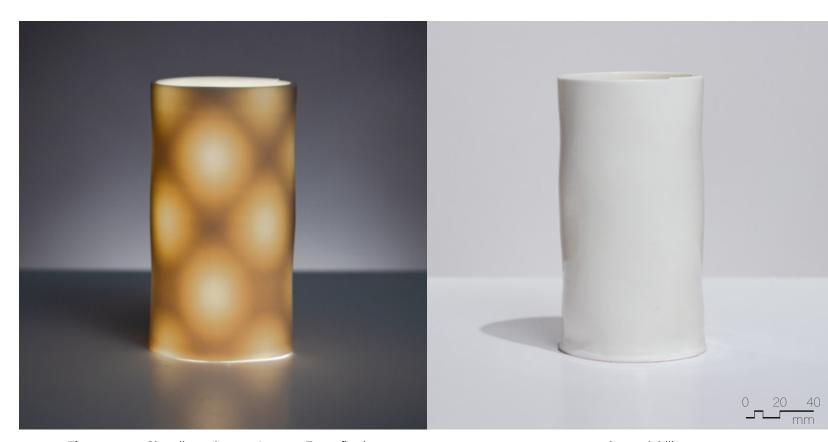
Figure 4.3.18 Clear liner glaze on Laguna Frost, fired to cone 6, 90mm x 90mm x 180mm, extrusion variability.
