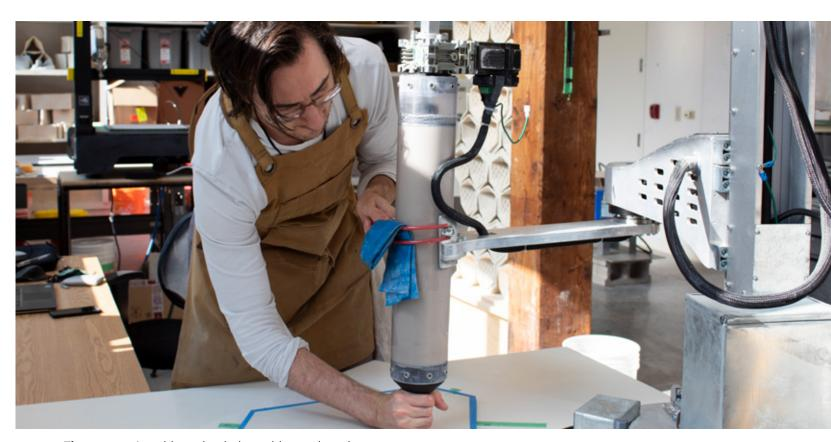
Figure 3.1.4 Attaching a loaded cartridge to the printer armature.
