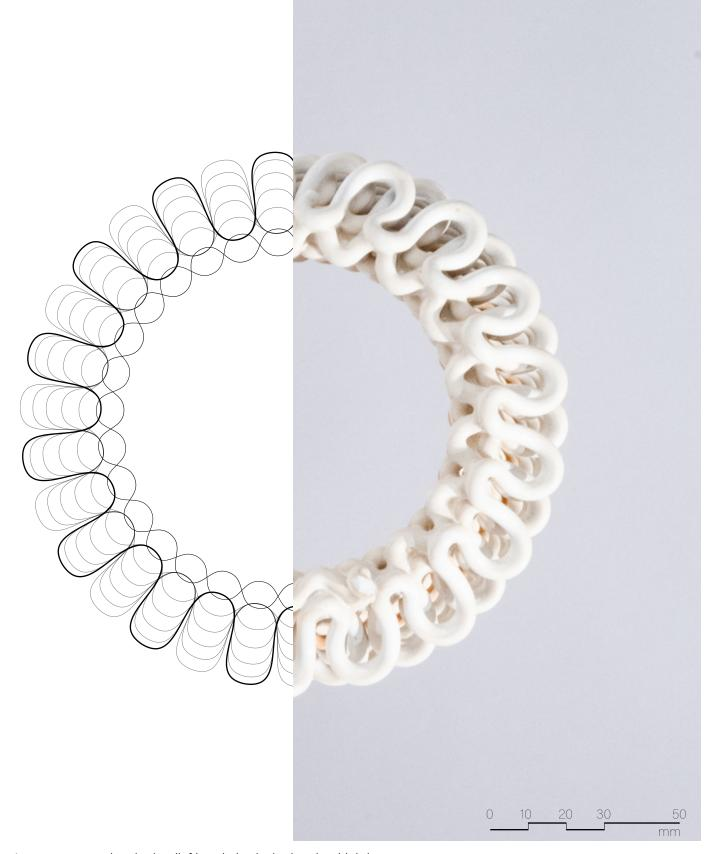
Figure 4.4.26 Loop pattern tool path plan (left) and physical print plan (right).
