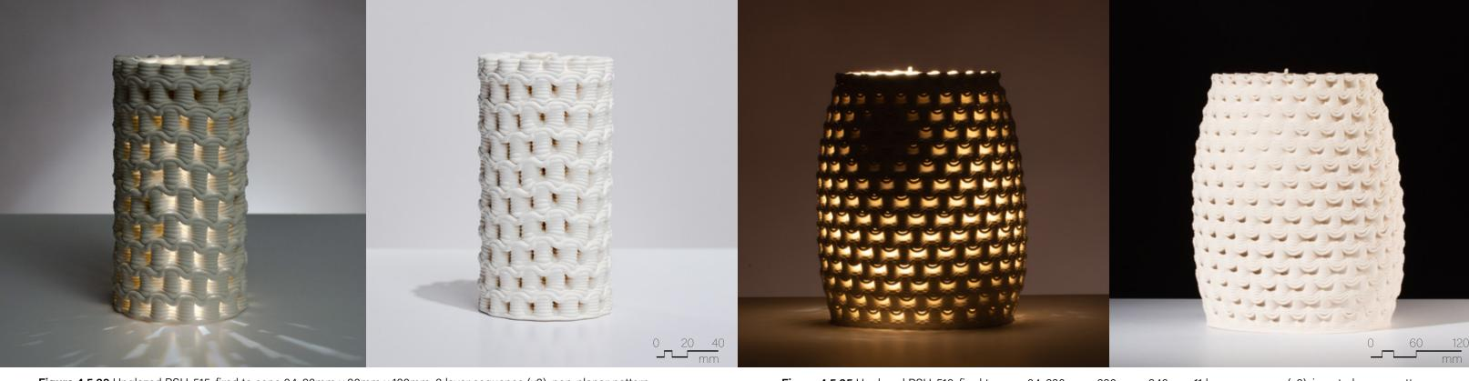
Figure 4.5.33 Unglazed PSH-515, fired to cone 04, 90mm x 90mm x 180mm, 8 layer sequence (x2), non-planar pattern.
