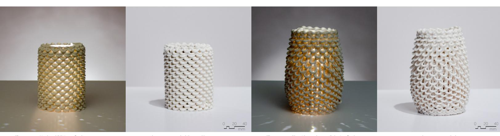
Figure 4.4.37 Unglazed PSH-515, fired to cone 04, 90mm x 90mm x 150mm, 3 layer sequence (x2), inverted loop pattern.
