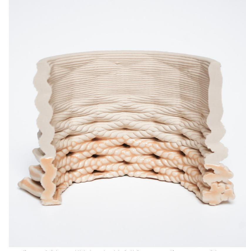
Figure 3.4.7 Preliminary material behaviour study, exploring 'braided' patterns generated from non-porous tessellations.
