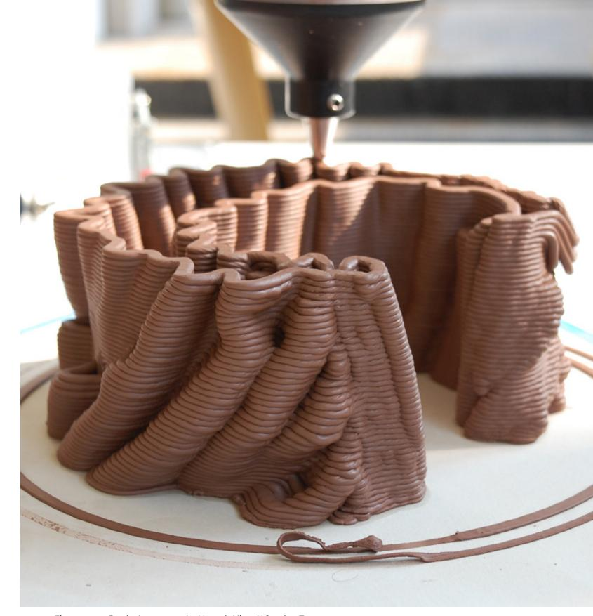
Figure 5.4.1 3D print in progress by Hannah Ni and Yingying Zeng.
