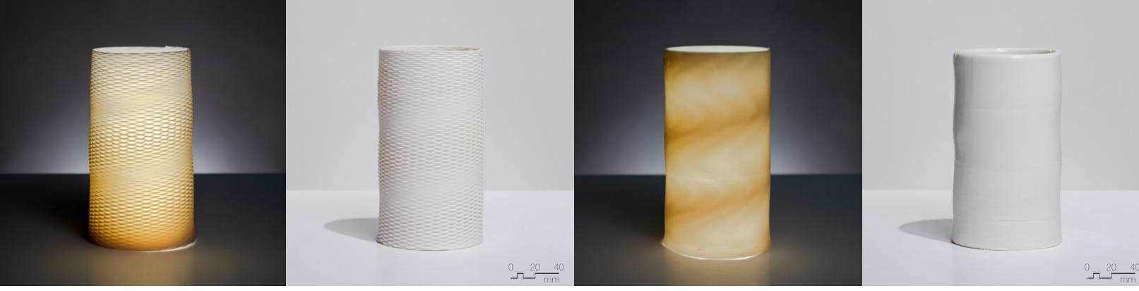
Figure 4.3.19 Clear liner glaze on Laguna Frost, fired to cone 6, 90mm x 90mm x 180mm, 2 layer sequence (x2), extrusion variability.
