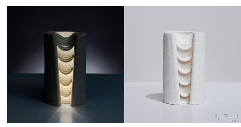
Figure 4.6.26 Unglazed PSH-515, fired to cone 04, 80mm x 80mm x 160mm, 18 layer sequence.
