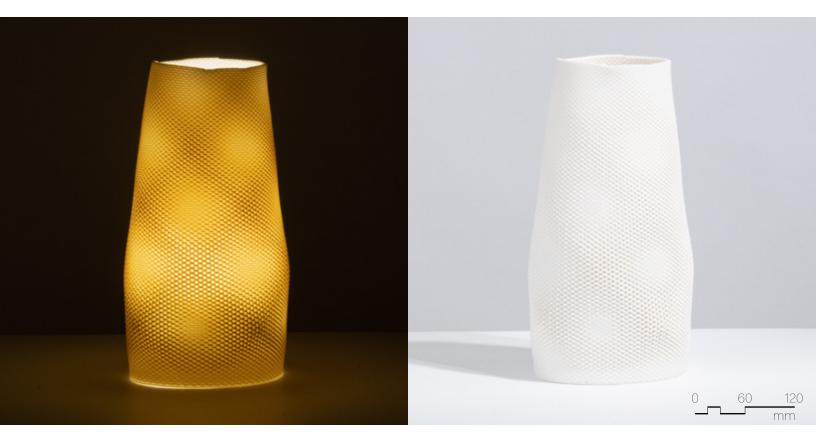
Figure 4.3.32 Unglazed Laguna Frost, fired to cone 6, 160mm x 160mm x 300mm, 2 layer sequence (x2), extrusion variability.
