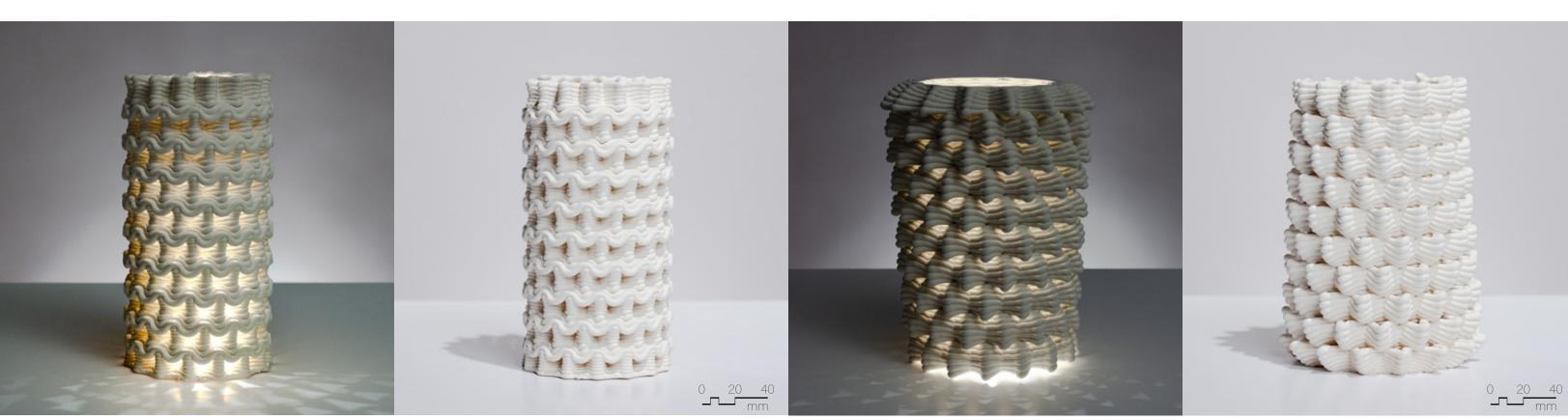
Figure 4.5.30 Unglazed PSH-515, fired to cone 04, 90mm x 90mm x 180mm, 8 layer sequence (x2).
