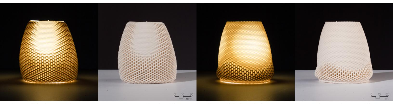
Figure 4.3.28 Unglazed Laguna Frost, fired to cone 6, 90mm x 90mm x 90mm, 2 layer sequence (x2), extrusion variability.
