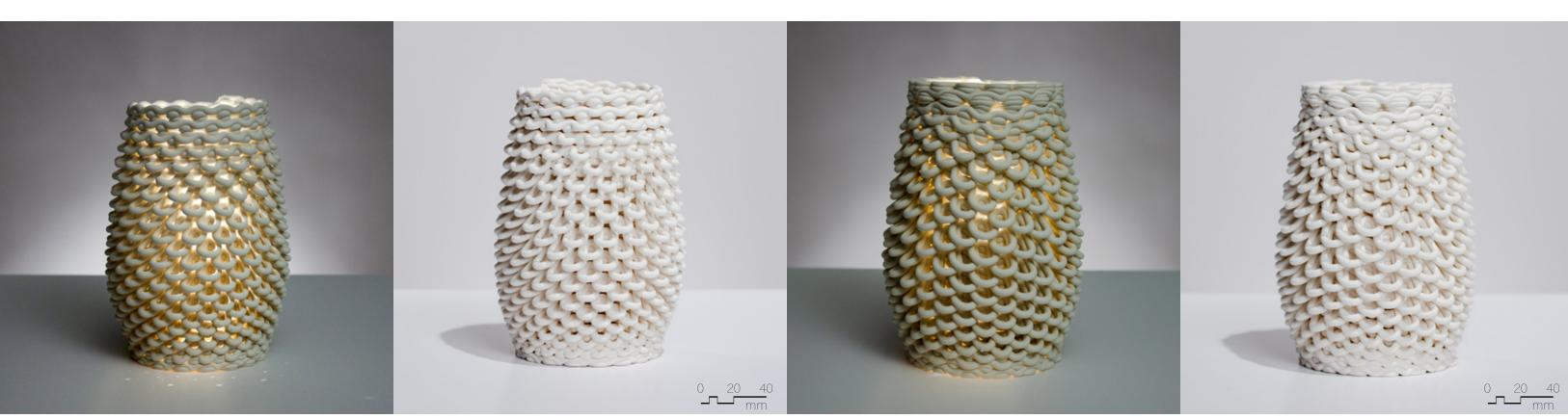
Figure 4.4.33 Unglazed PSH-515, fired to cone 04, 90mm x 90mm x 180mm, 3 layer sequence (x2).
