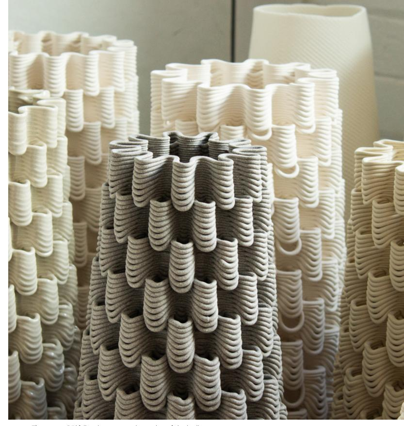
**Figure 4.6.2** 'XL' full scale prototypes in a variety of clay bodies.
