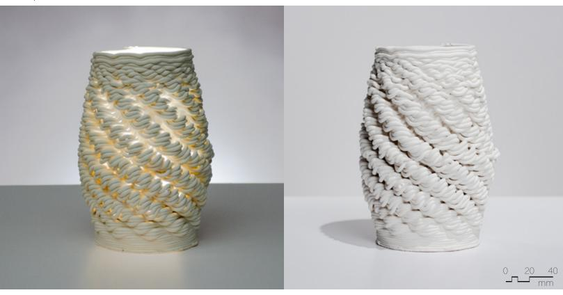
Figure 4.4.45 Unglazed PSH-515, fired to cone 04, 90mm x 90mm x 180mm, 3 layer sequence (x4), spiral pattern.
