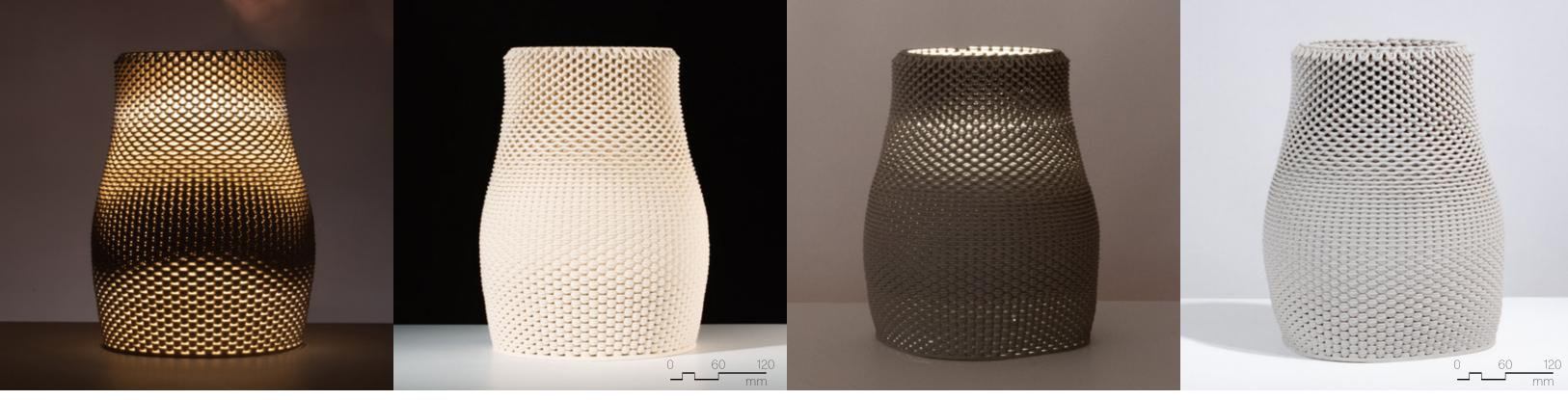
Figure 4.4.60 Unglazed PSH-516, fired to cone 04, 280mm x 280mm x 350mm, 3 layer sequence (x2).
