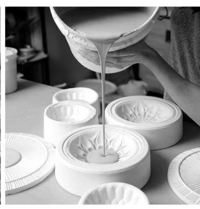
Figure 2.2.2 Inlaid slip casting moulds by Kelly Justice.
