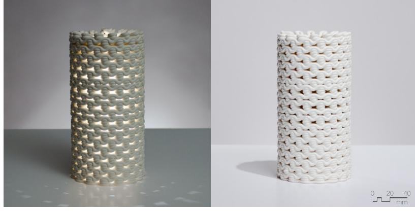
Figure 4.5.27 Unglazed PSH-515, fired to cone 04, 90mm x 90mm x 180mm, 4 layer sequence (x2).
