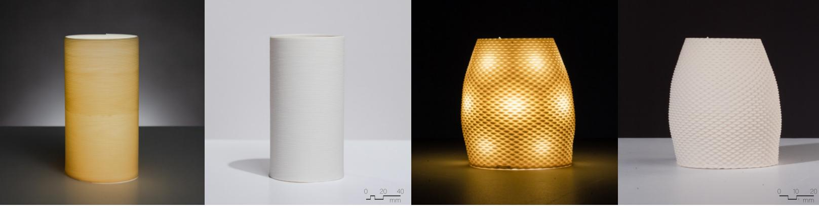
Figure 4.3.23 Unglazed Laguna Frost, fired to cone 6, 90mm x 90mm x 180mm, 2 layer sequence (x2), extrusion variability.
