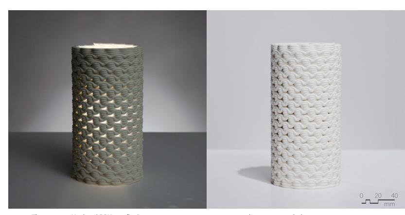
Figure 4.5.28 Unglazed PSH-515, fired to cone 04, 90mm x 90mm x 180mm, 4 layer sequence (x2).
