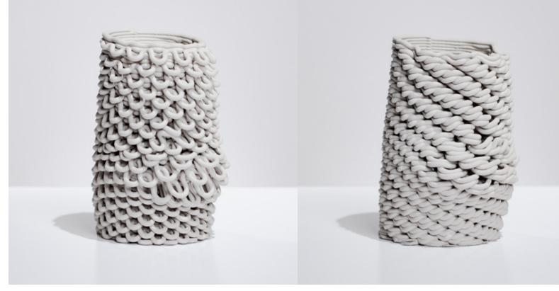
Figure 4.4.28 Non-planar looping print studies displaying deformation and reformation.
