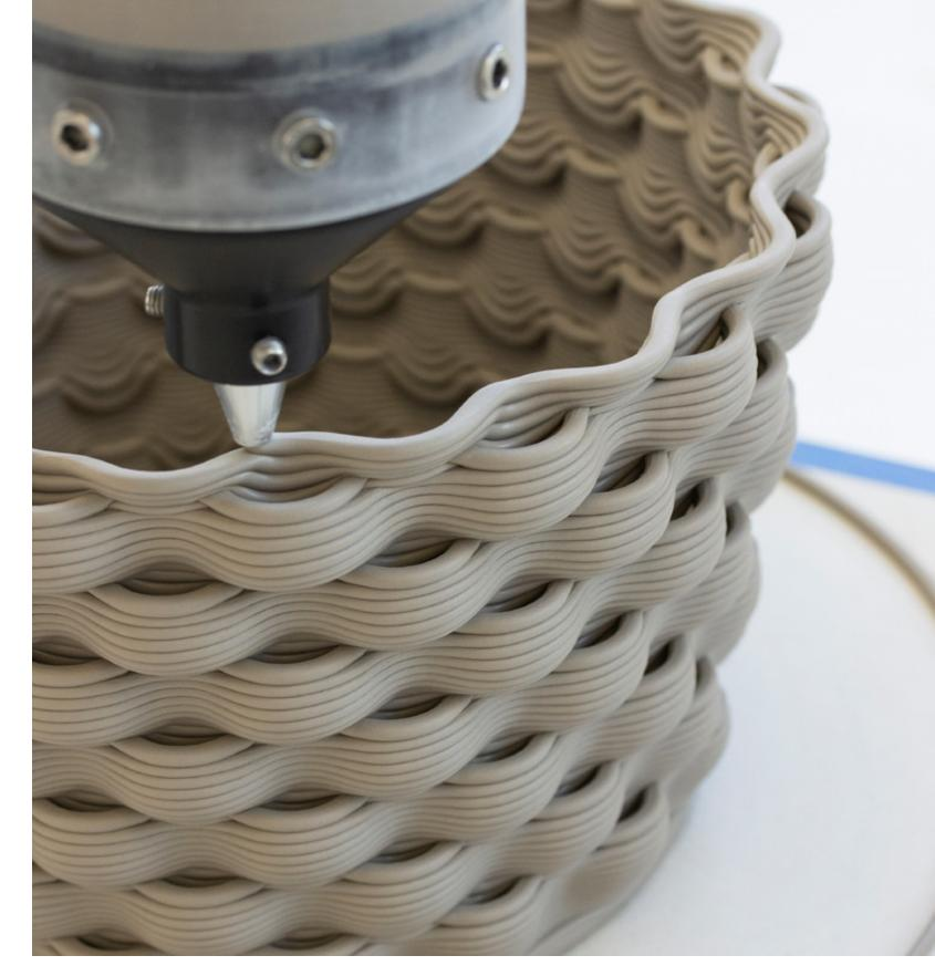
Figure 3.1.1 'L' prototype print in progress.
