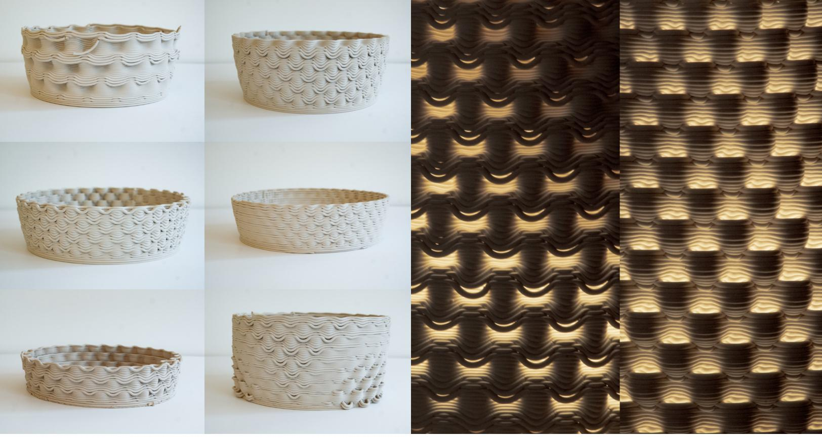
**Figure 4.5.23** Rapid iteration of aperture sizes and scoop profiles. The final iteration in the sequence incorporates both inward and outward-facing scoops.
