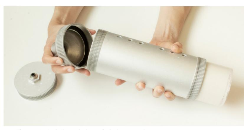
Figure 3.1.6 Prepping the clay cartridge for pressurization via. compressed air.
