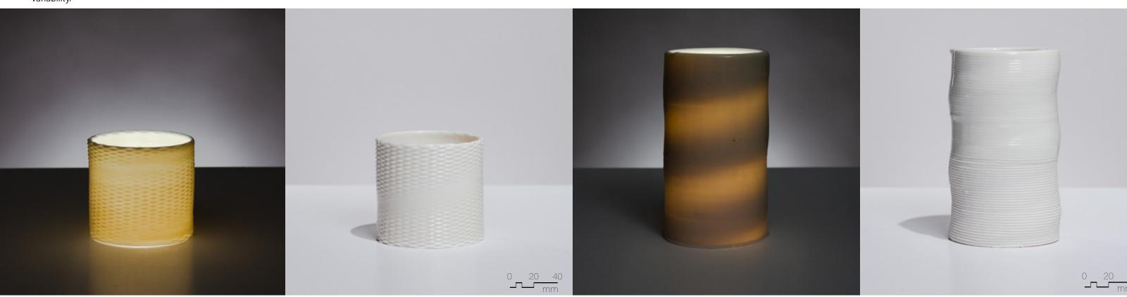
Figure 4.3.20 Clear liner glaze on Polar Ice, fired to cone 6, 90mm x 90mm x 80mm, 2 layer sequence (x2), extrusion variability.
