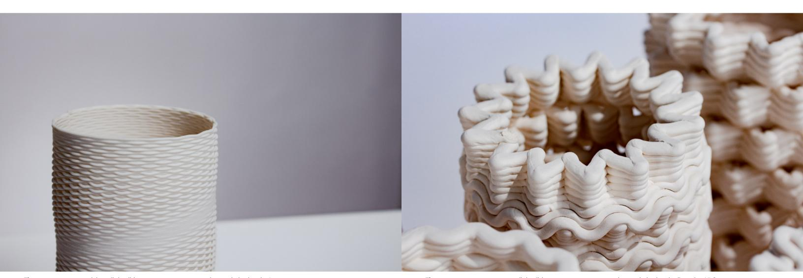
Figure 2.5.9 1mm porcelain wall detail (100mm x 100mm x 200mm), extruded using the Lutum 4.
