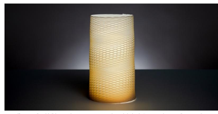
Figure 2.6.6 Porcelain light screen (100mm x 100mm x 200mm), extruded using the Lutum 4.5 using a 1mm diameter nozzle.
