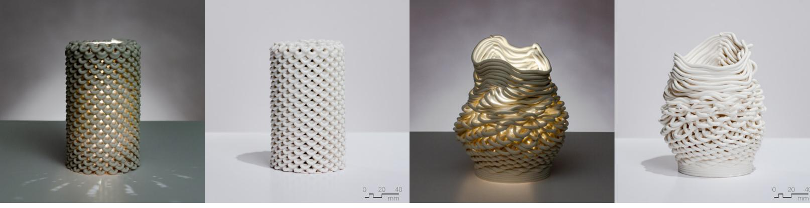
Figure 4.4.36 Unglazed PSH-515, fired to cone 04, 90mm x 90mm x 180mm, 3 layer sequence (x2), inverted loop pattern.
