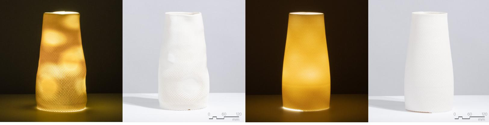
Figure 4.3.31 Clear liner glaze on Polar Ice, fired to cone 6, 160mm x 160mm x 300mm, 2 layer sequence (x2), extrusion variability.
