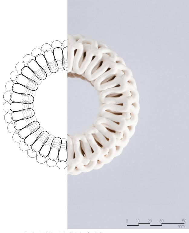
Figure 4.4.27 Inverted loop pattern tool path plan (left) and physical print plan (right).
