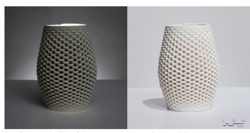
Figure 4.4.31 Unglazed PSH-515, fired to cone 04, 90mm x 90mm x 180mm, 2 layer sequence (x2).
