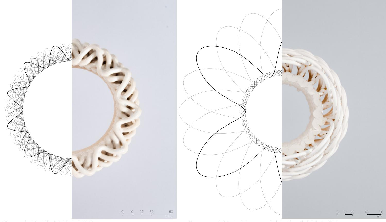
Figure 4.4.24 Spiral pattern tool path plan (left) and physical print plan (right).
