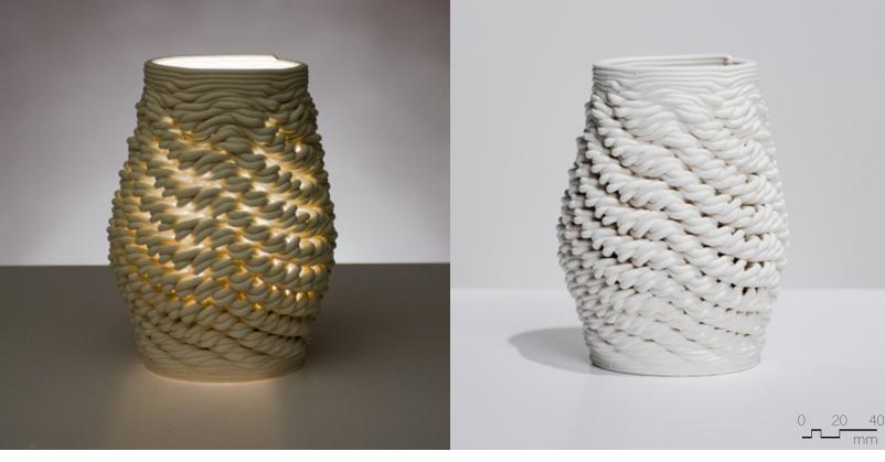
**Figure 4.4.44** Unglazed PSH-515, fired to cone 04, 90mm x 90mm x 180mm, 2 layer sequence (x4), spiral patterning, non-planar pattern.
