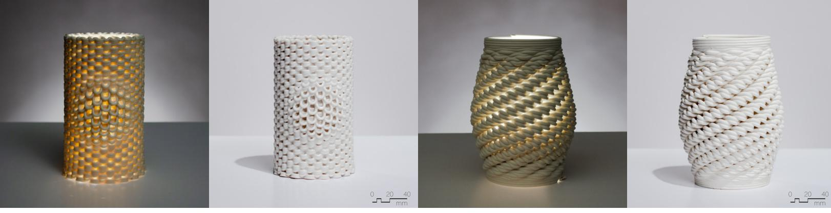
**Figure 4.4.40** Clear liner glaze on Polar Ice, fired to cone 6, 90mm x 90mm x 180mm, 2 layer sequence (x2), inverted loop pattern.
