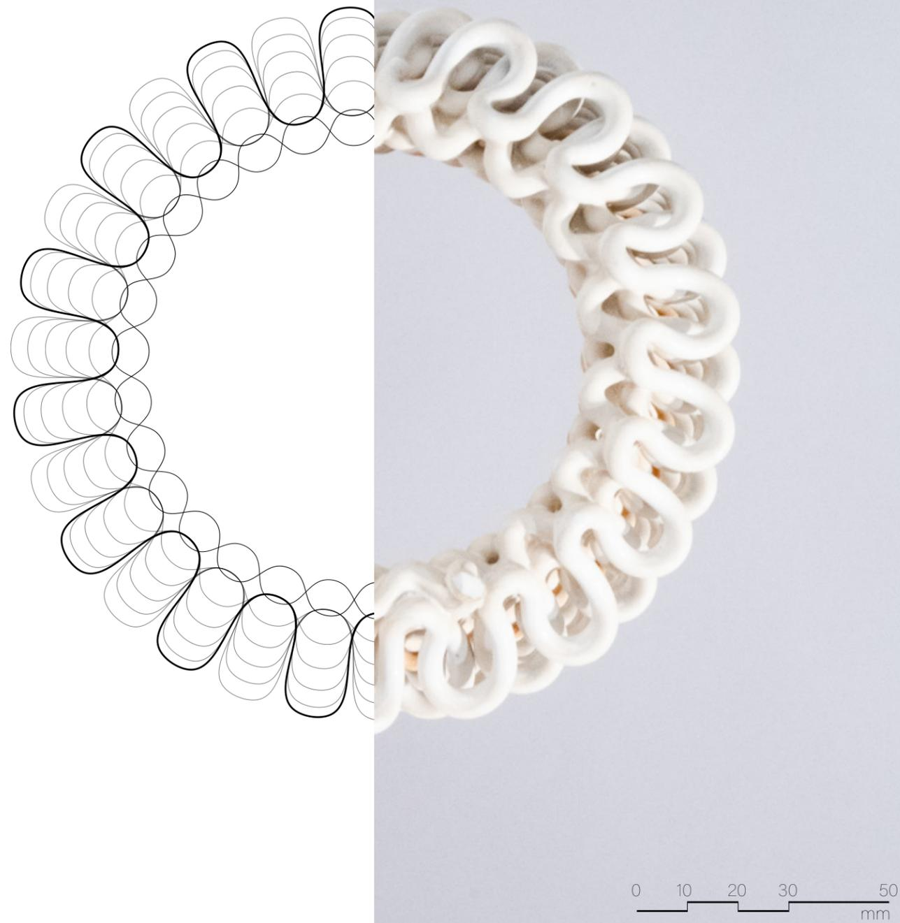
**Figure 4.4.26** Loop pattern tool path plan (left) and physical print plan (right).
