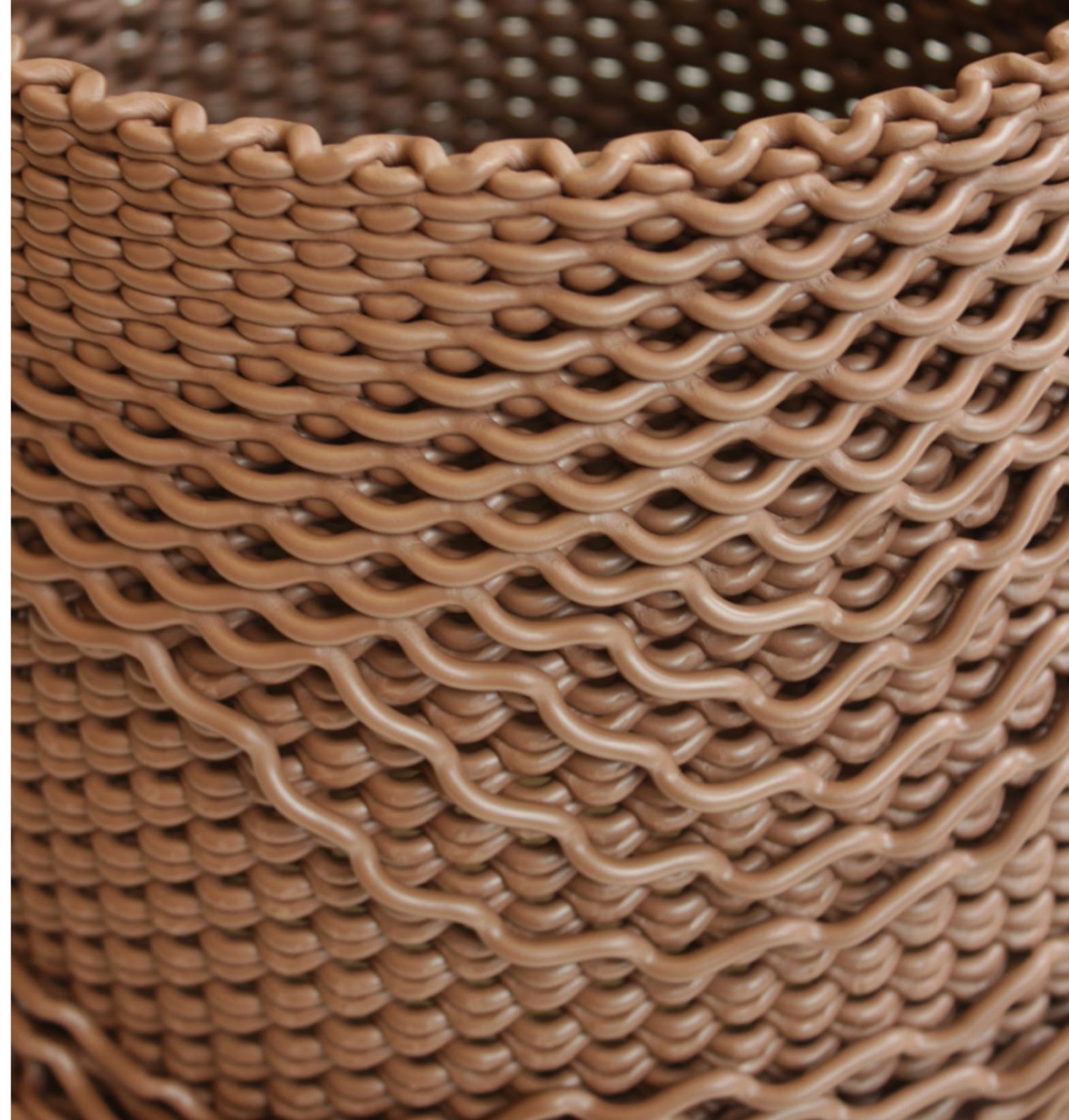
**Figure 1.3.1** Terracotta undergoing plastic deformation and subsequent delamination during 3D printing.
