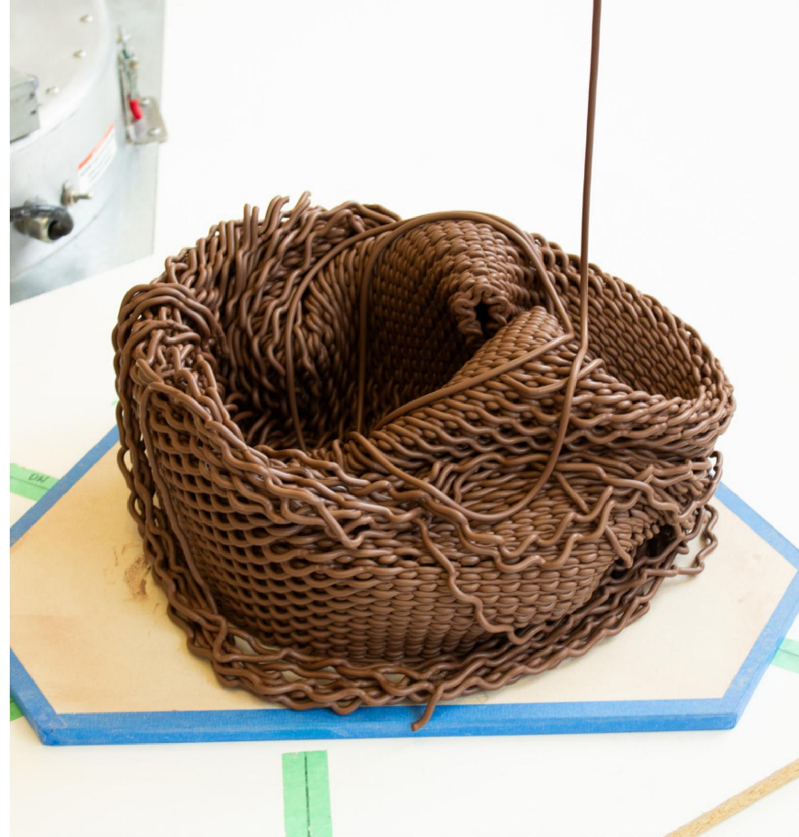
**Figure 4.4.2** Structural collapse of 'M' prototype during print.
