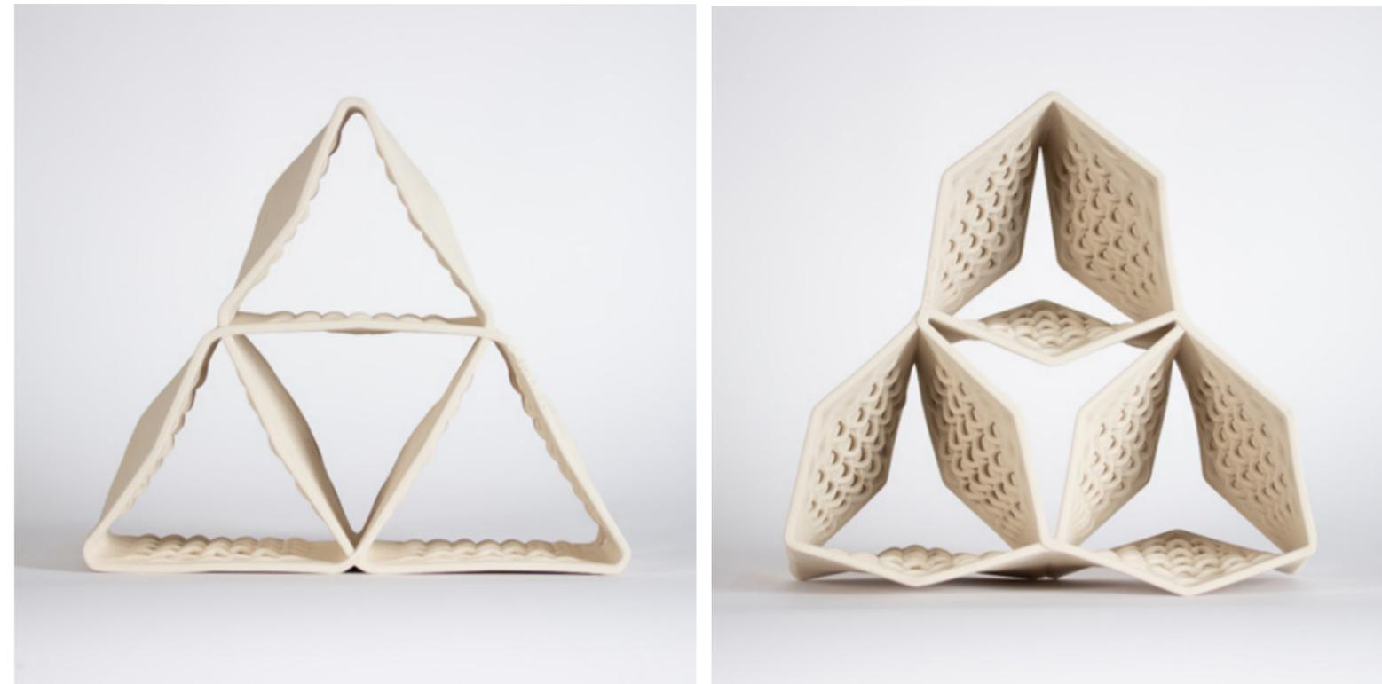
**Figure 5.3.1** Final units in HIVE showing apertures that selectively open and close along the wall.
