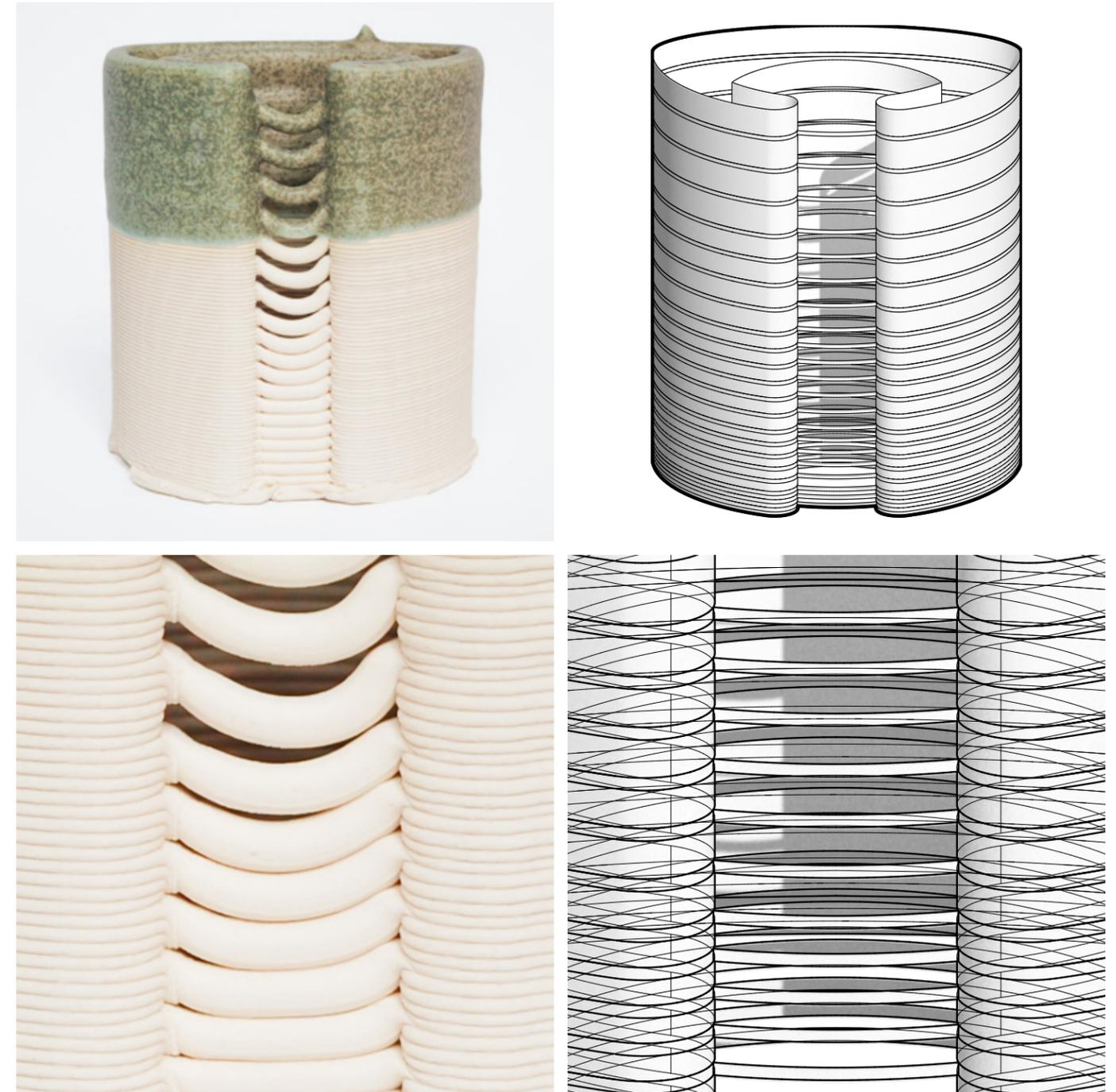
Figure 4.2.11 Porous hung coil pattern, ASM1 glaze on PSH-516.
