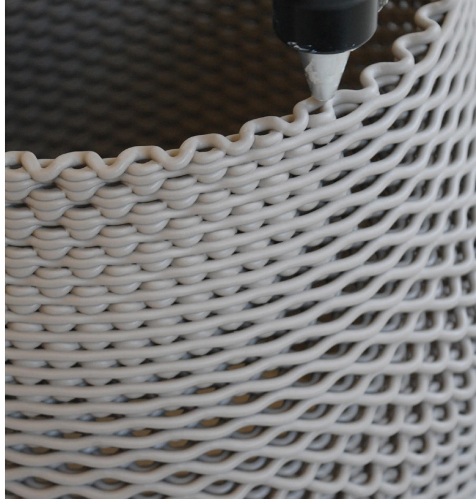
**Figure 5.1.1** Stoneware undergoing plastic deformation during 3D printing.
