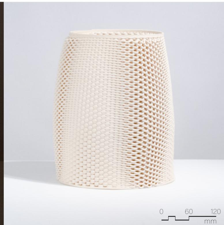
**Figure 4.4.65** Unglazed PSH-516, fired to cone 04, 300mm x 300mm x 350mm, 3 layer sequence (x2).
