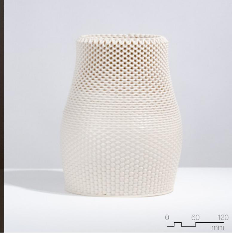
**Figure 4.4.64** Clear liner glaze on PSH-516, fired to cone 6, 280mm x 280mm x 350mm, 3 layer sequence (x2).
