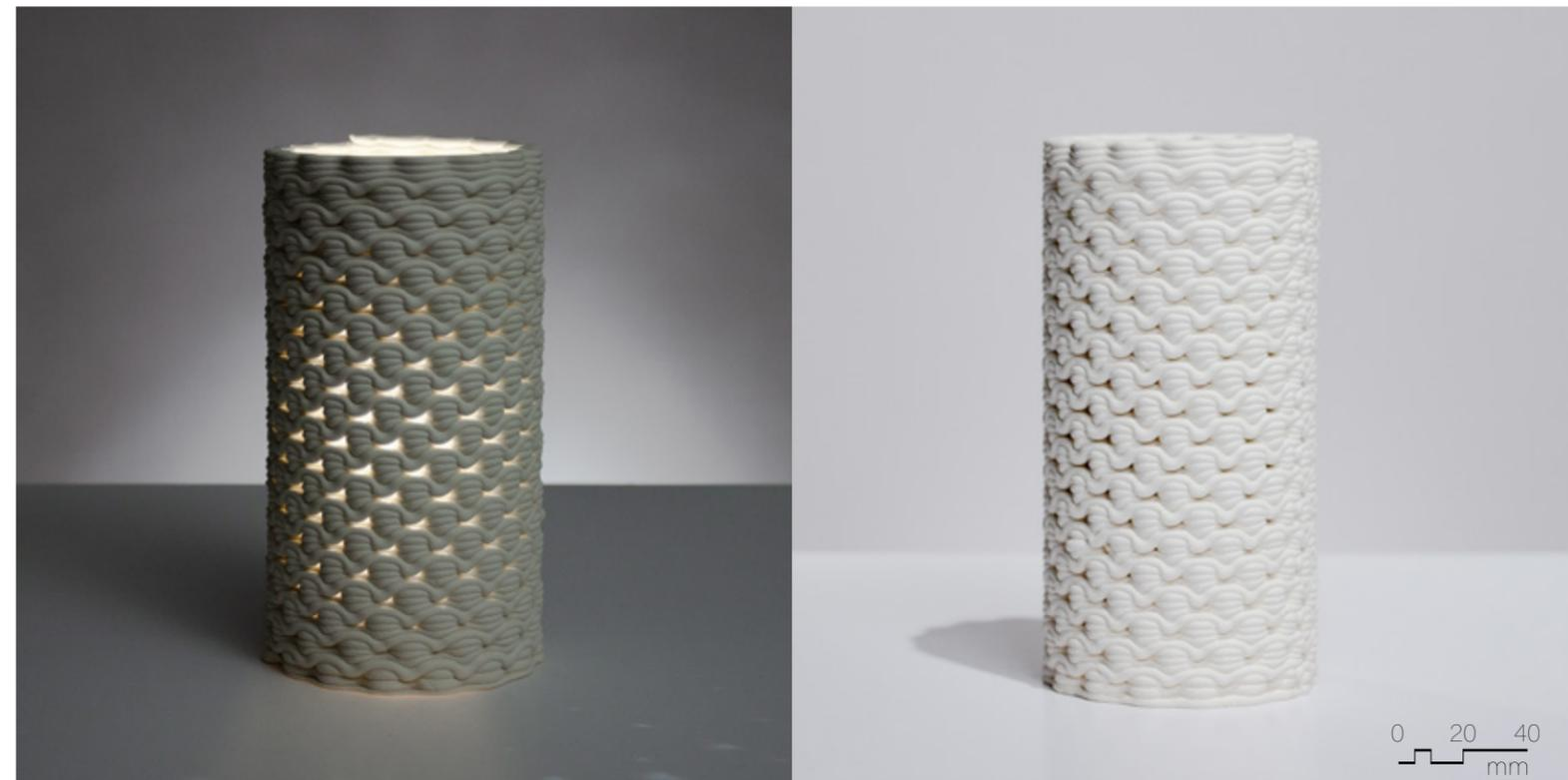
**Figure 4.5.28** Unglazed PSH-515, fired to cone 04, 90mm x 90mm x 180mm, 4 layer sequence (x2).
