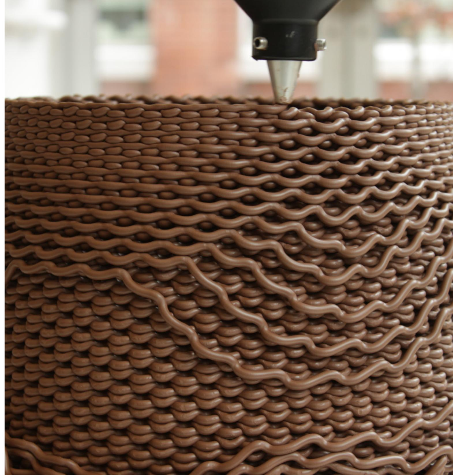
Figure 3.1.2 M prototype in terracotta, delaminating during printing.
