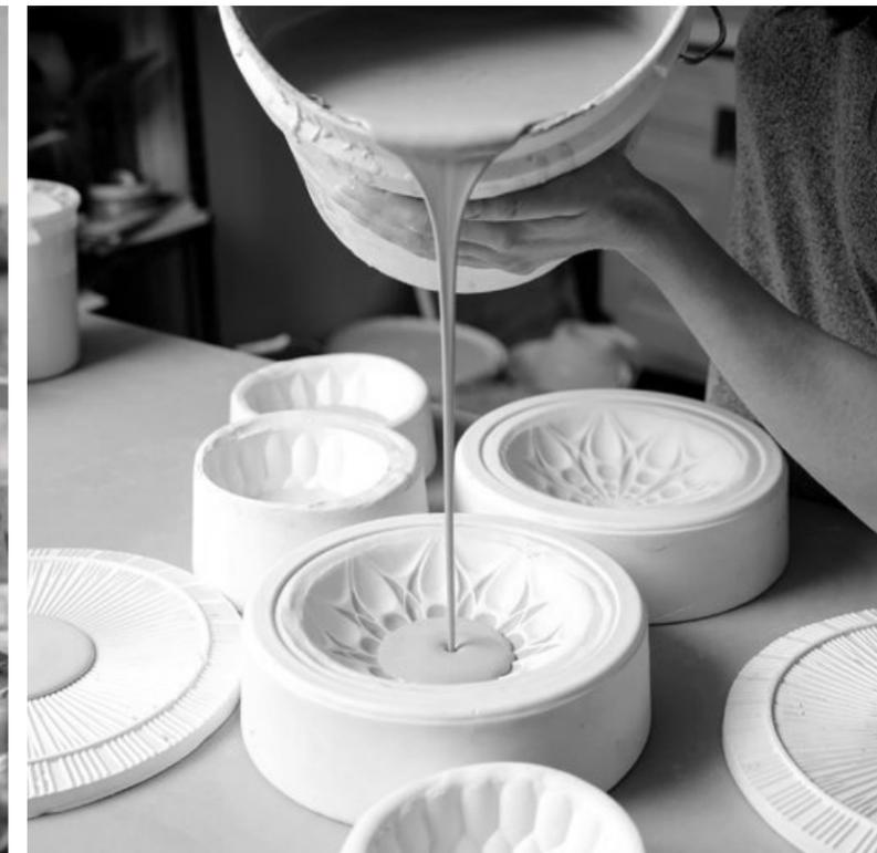
Figure 2.2.2 Inlaid slip casting moulds by Kelly Justice.
