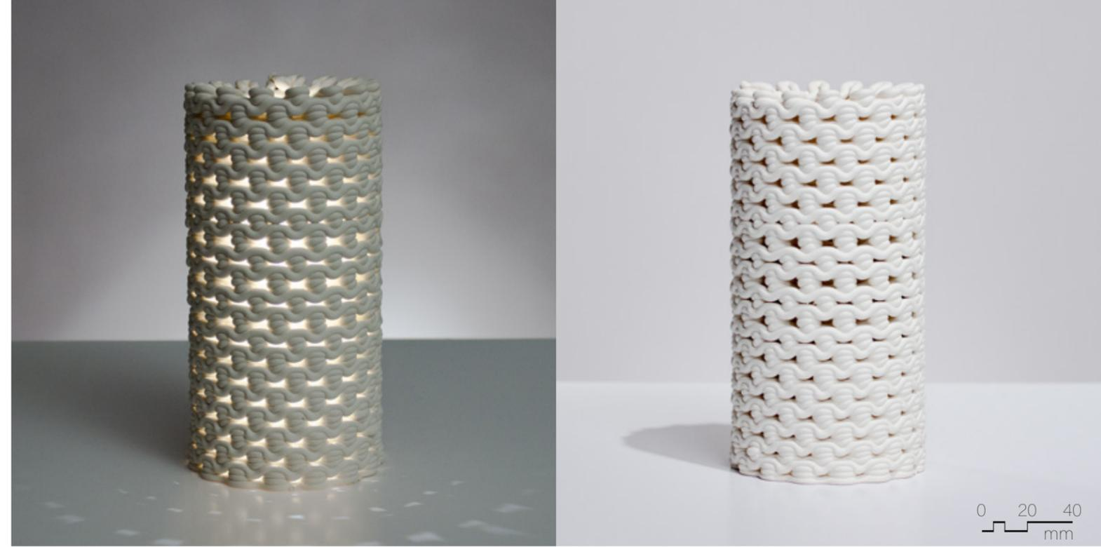
**Figure 4.5.27** Unglazed PSH-515, fired to cone 04, 90mm x 90mm x 180mm, 4 layer sequence (x2).
