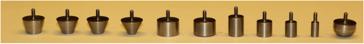
Figure 4.11 Pure iron core tip shapes
