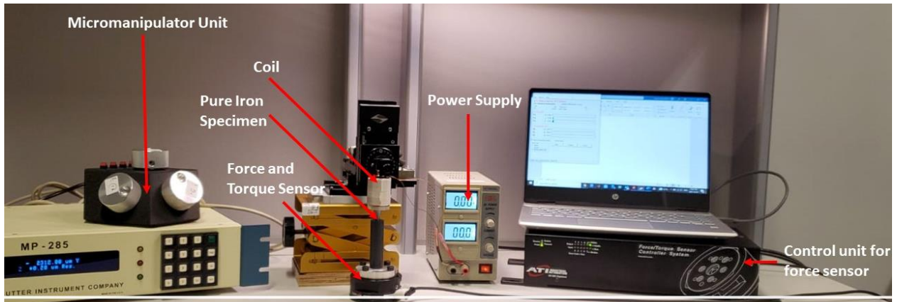
Figure 5.9 Experimental Measurement of Force using a Force and Torque Sensor
