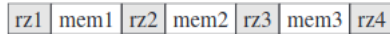
Figure 4: Redzones guarding heap allocations. These redzones contain allocation stack traces and allocator thread ID
