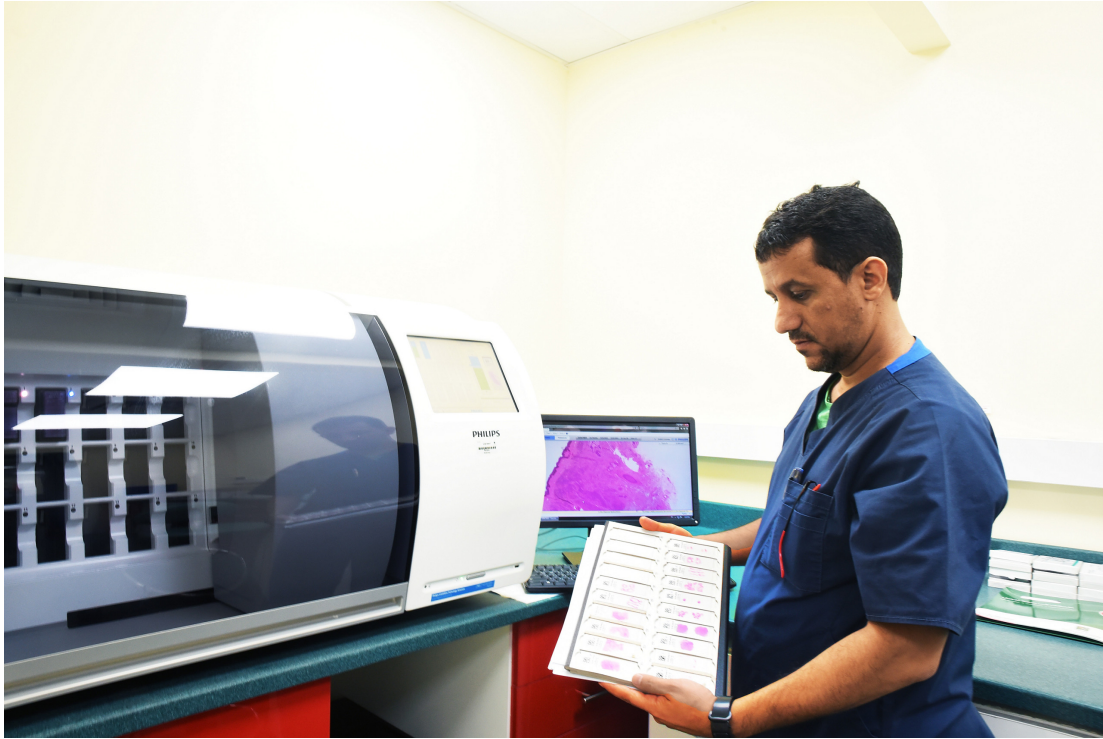
Figure 2.3: An example of a whole slide imaging scanner manufactured by Philips [5]. The whole slide scanner is on the left, the image management software shown on the monitor in the middle, and the operator holding glass slides on the right.
