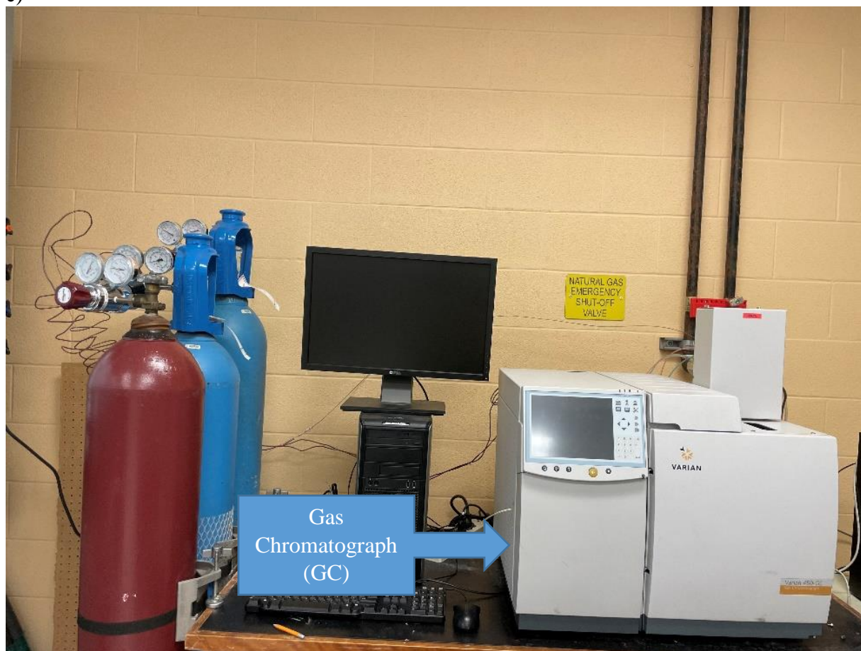
Figure 11: Photos of set-up for evaluation of sensing materials a) cylinders of gas analytes; b) sample gas flow set-up; c) gas chromatograph
