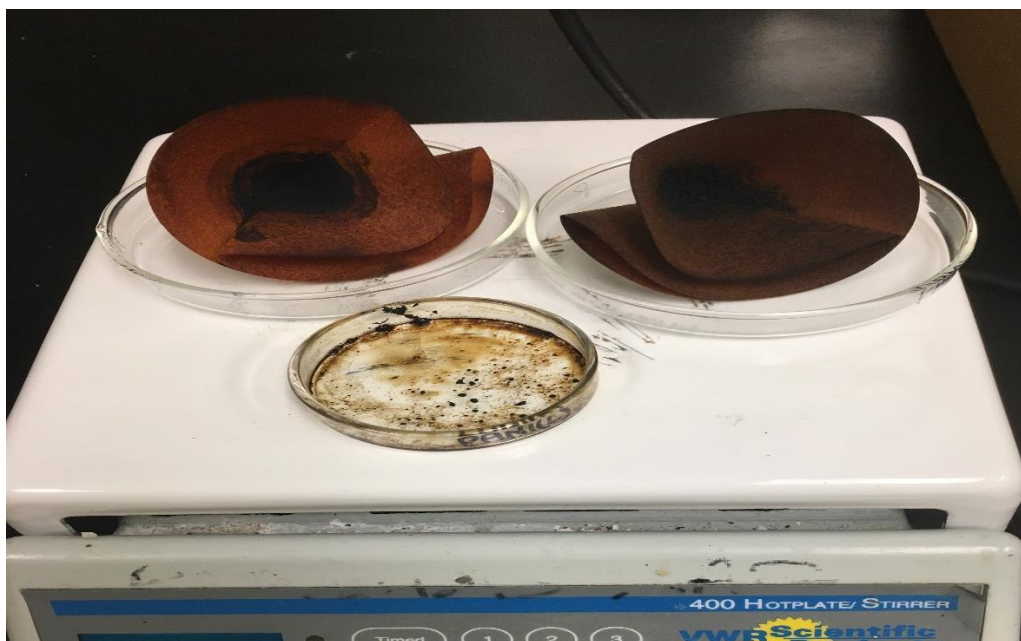
Figure D4: PANI (S) and PANI (L) filter paper in a petri dish on the heater plate for heating at 60 degrees Celsius for 3 hrs
