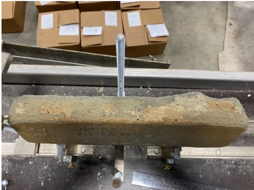
Figure 6-17 Visual images of the 400 samples at 0 and 180 cycles – thaw in water
