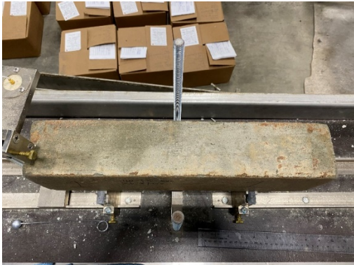
Figure 6-15 Visual images of the 600 samples at 0 and 180 cycles – thaw in water
