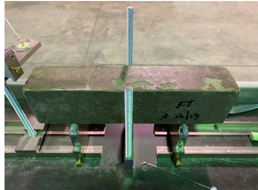
Figure 6-15 Visual images of the 600 samples at 0 and 180 cycles – thaw in water
