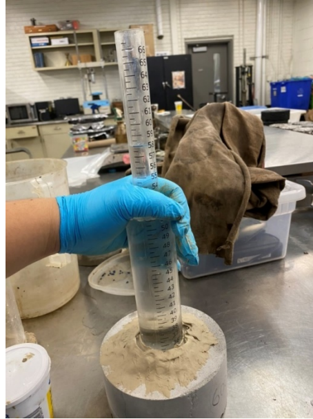
Figure 3-7 Permeability test layout
