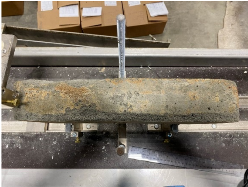
Figure 6-20 Visual images of the 400 samples at 0 and 180 cycles – thaw in air
