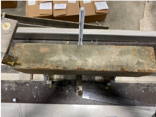
Figure 6-19 Visual images of the 475 samples at 0 and 180 cycles – thaw in air
