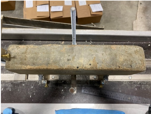
Figure 6-16 Visual images of the 475 samples at 0 and 180 cycles – thaw in water
