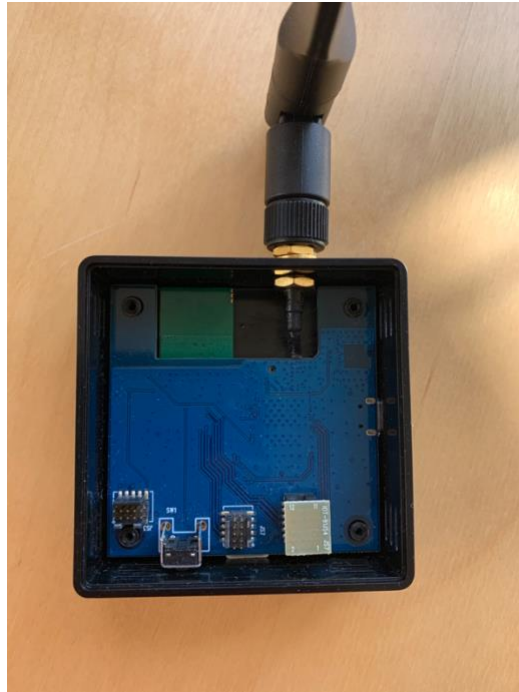
Figure 4-3. BLG840x acting as a gateway for sending data to cloud.
