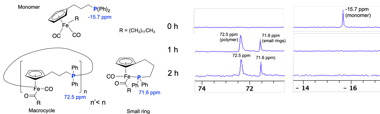
Figure 3.11. Time-dependent {}^{31}\text{P} NMR spectra for the MIP of {}^{\text{P}}\text{FpC}_{12} at 100 °C in toluene with 50% wt concentration.
