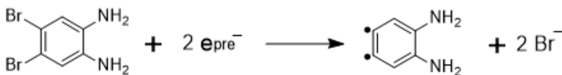
Figure 1- 10 The molecular structure of FMD-2Br-DAB and complete process of its DET reaction.
