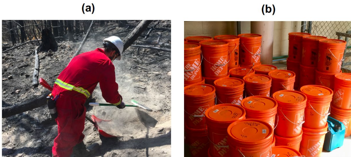
Figure 4.1: Ash collection following the Thuya Lake Road (TLR) wildfire near Little Fort B.C. (a) ; pails of post-wildfire ash samples used for preparing the severely deteriorated source water used during pilot-scale testing (b) .
