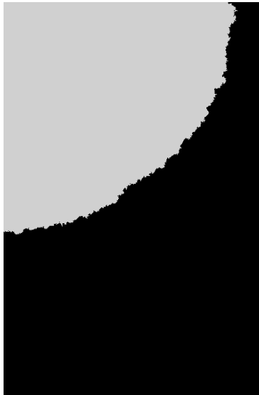
(b) An example of a cluster of faults placed in the top left of an SRAM array.
