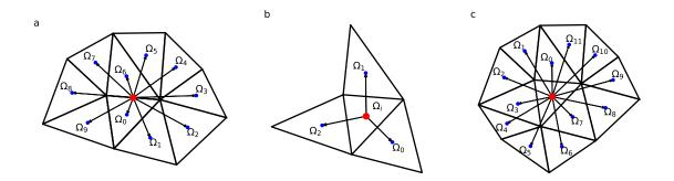
Figure 3.2: Examples of gradient reconstruction stencils for (a) Green-Gauss least squares method, (b) compact least squares method, and (c) extended least squares method.
