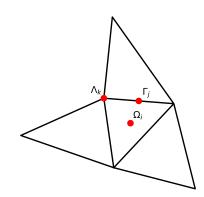
Figure 3.1: Mesh topology and nomenclature for a small subset of an unstructured triangular mesh.  $\Omega_i$  refers to element *i*, located at the element centroid.  $\Gamma_j$  refers to edge *j*, located at the edge midpoint.  $\Lambda_k$  is the *k*-th node. Edge  $\Gamma_j$  connects exactly two elements and two nodes, while element  $\Gamma_j$  is connected to exactly three edges.
