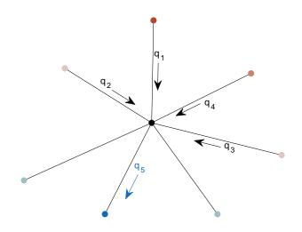
Figure 3.5: Schematic diagram of the mass conservation method at nodes. For this node, four edges have mass flow directed towards the node. The total flow is directed out through the edge with the steepest downhill potential  $(q_5)$ .
