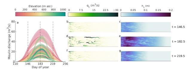
Figure 4.3: Overview of model outputs for the baseline scenario. (a) Moulin flux for the 50 moulins, colored by the elevation of the moulins The vertical dashed lines indicate the times used for panels (b-g). (b, d, f) Volume flux in the channels at noon on days 146, 182, and 219. (c, e, g) Sheet water thickness at noon on days 146, 182, and 219.
