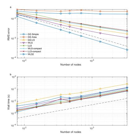
Figure 3.3: Comparison of gradient reconstruction methods on unstructured triangular meshes. (a) RMS error between exact and numerically approximated  $f_x(x, y)$ . Dashed line shows a linear reference. (b) Total time in seconds to compute the gradient for all mesh elements. Dashed line shows a linear reference.
