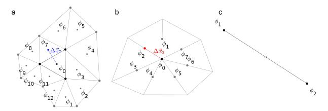
Figure B.1: (a) Gradient reconstruction stencil centered on element  $\Omega_0$ . The blue vector  $\Delta \mathbf{x}_7$  illustrates the distances used in equation (3.6) to calculate the gradient on element  $\Omega_0$ . (b) Stencil used to calculate the channel potential on node  $\Lambda_0$ . (c) The along-channel potential gradient is simply calculated from the potential difference on the connecting nodes and the length of the edge.
