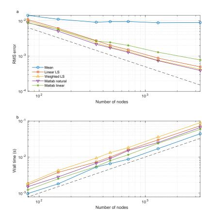
Figure 3.4: Comparison of gradient reconstruction methods on the edge network. (a) Evaluation of the methods by the root mean square (RMS) error in their reconstruction of the along-channel slope  $\frac{df}{ds}$ . (b) Total computational time in seconds to compute derivativess for the entire mesh.
