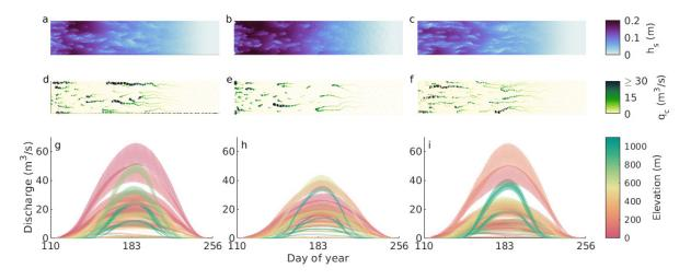
Figure 4.7: modelled drainage system for the baseline case (a, d, g), case R1 with a coarse mesh (b, e, h), and case R2 with a fine mesh (c, f, i). The panels show water sheet thickness (a-c) and channel flow (d-e) at time t = 182.5 days, and moulin inputs (g-i).
