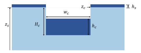
Figure 4.1: Cross-sectional geometry of supraglacial channels.
