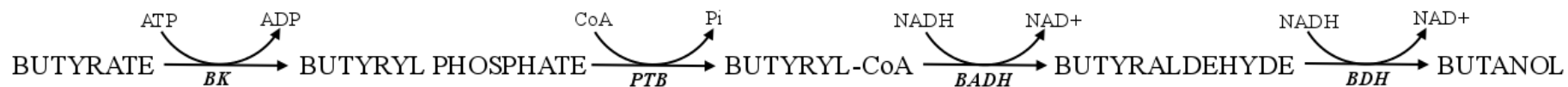
Figure 4. Schematic diagram showing two potential butanol production pathways (A and B) within the bacterium C. saccharoperbutylacetonicum N1-4. CoAT: CoA transferase, BADH: butylaldehyde dehydrogenase, BDH: butanol dehydrogenase, BK: butyrate kinase, PTB: phosphotransbutyrylase. (Modified from Al-Shorgani et al. 2012).
