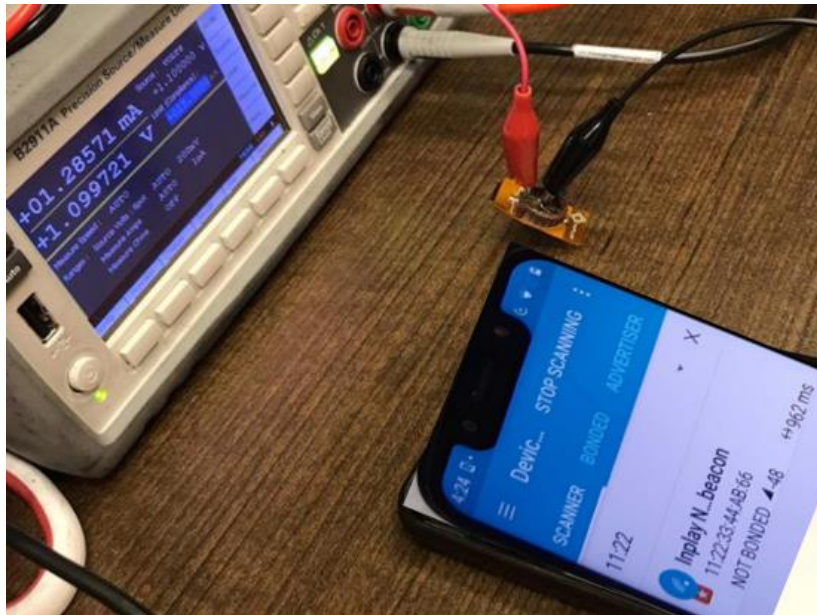
Figure 3.9 Displayed of transmitted beacon on android smart phone indicated with red showing (In-play Nanobeacon)
