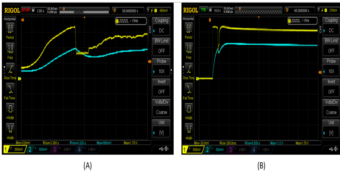
Figure 4.16: Waveforms of both sensors; a) flexible wetness sensor, b) water leak sensor
