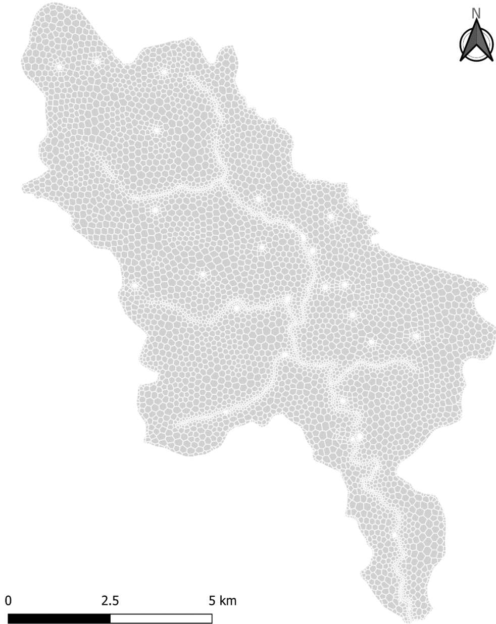
Figure 5-5 – Voronoi unstructured model grid used for the GW model, based upon HGS triangular grid for a previous model of the area. Locations of pumping and observation wells, as well as Alder Creek, can readily be observed in the grid discretization.
