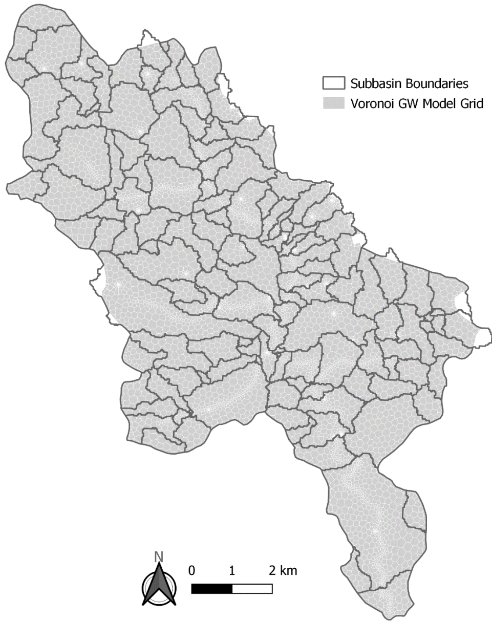
Figure 5-13 – Overlap of the model spatial representations. Priority was placed on ensuring every node of the groundwater model was covered by a subbasin.
