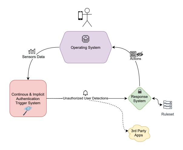
Figure 2.5: The information and actions flow between the continuous and implicit authentication system, the operating system, third party applications, and the response system.
