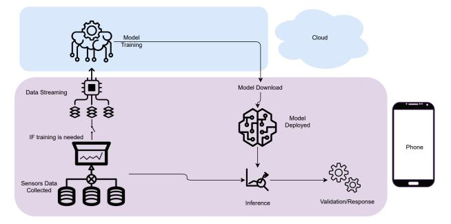
Figure 2.2: System architecture, showing the training taking place on a cloud resource.
