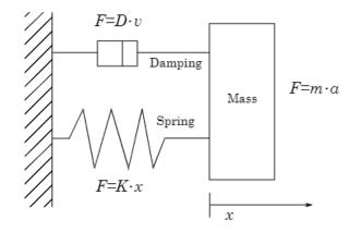
Figure 2.10: Schematic of an accelerometer. Source: [3]
