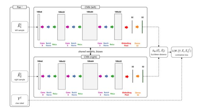
Figure A.9: Siamese Convolutional Neural Network architecture with FCN sub networks proposed by [15] as modeled after [17]. All filters use padding and the vector of the last layer (marked in green) is considered the deep feature representation. Adapted from [13]
