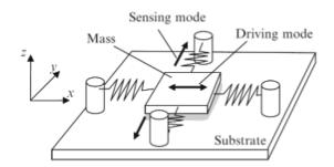
Figure 2.13: Schematic of a vibrating gyroscope. Source: [5]
