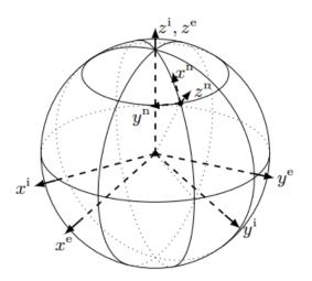
Figure 2.9: Coordinate frames, n-frame at a certain location on earth and the e-frame rotating with earth and the i-frame. Source: [2]
