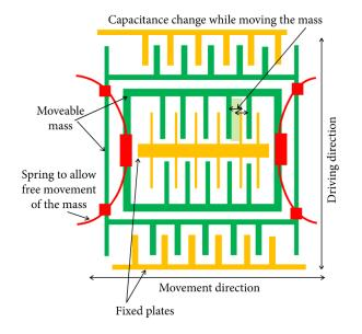
Figure 2.12: Gyroscope structure. Source: [4]
