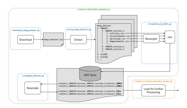
Figure A.3: Initial data preparation procedure along with corresponding python software modules. Adapted from [15]
