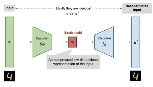
Figure 4.4: Auto-Encoder model architecture. Source: [10]
