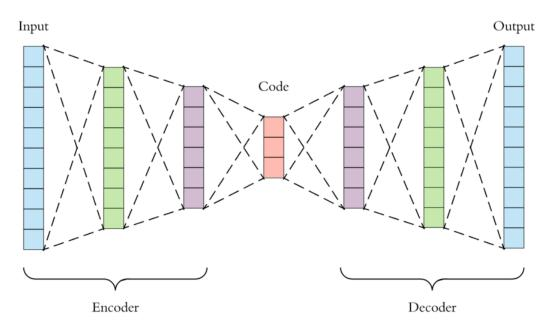
Figure 4.5: Auto-Encoder architecture featuring the encoder and decoder multi layered networks. Source: [11]
