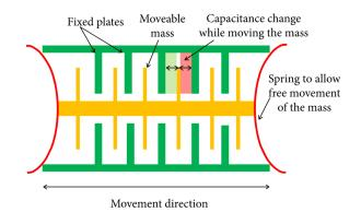
Figure 2.11: Accelerometer structure. Source: [4]
