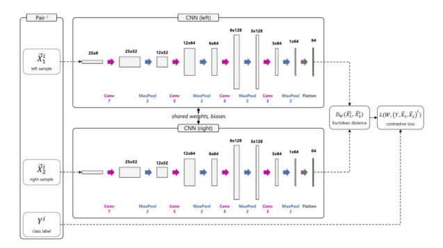
Figure A.8: Siamese Convolutional Neural Network architecture with 1D filters proposed by [16]. All filters use padding and the vector of the last CNN layer (marked in green) is considered the deep feature representation. Adapted from [13]
