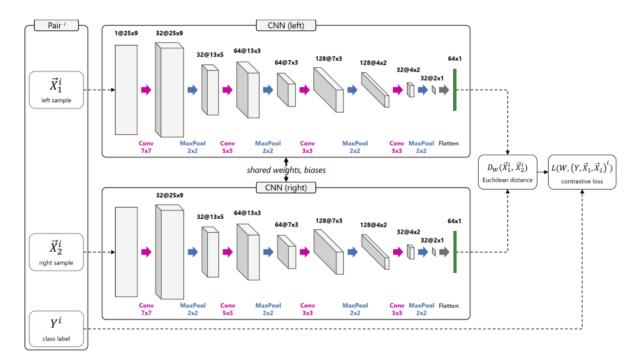
Figure A.10: Siamese Convolutional Neural Network architecture proposed by [16]. All filters use padding and the vector of the last CNN layer (marked in green) is considered the deep feature representation. Adapted from [13]
