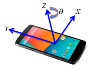
Figure 2.8: Axes of sensors on many phones. Source: [1]
