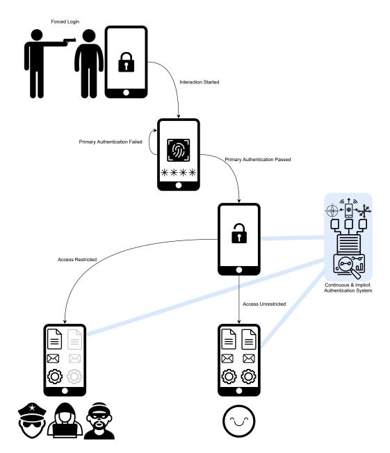
Figure 2.4: An example forced login scenario, showing how the proposed system can hide data, and apps on the phone to prevent losses and damages.
