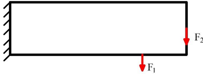
Figure 5.1: Simple cantilever design problem with two load cases.
