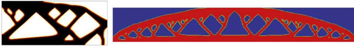
Figure 2.16: Optimal designs with 45° overhang angles for a half and full MBB beam by [101] and [76].
